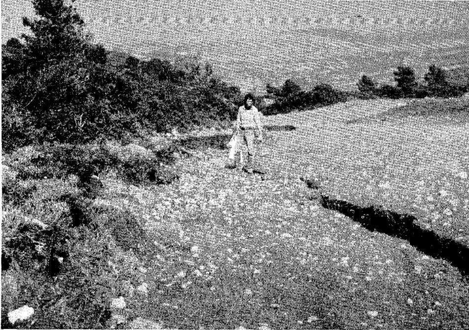
FIGURE 2.9 Eastern end of the Kalamaki trace at the location where ground motion was observed during a magnitude 5.7 earthquake on March 7, 1981. The main rupture trace is on left side of the photograph. The smaller rupture on the right is a secondary, near-surface cantilever failure in the soil, which appeared several days after the original surface break. This pattern is analogous to the relation between the southern and northern earthquakes and surface ruptures.
