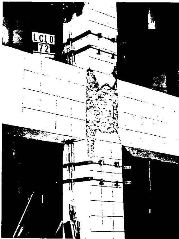
Fig. B31 Specimen LC10 after Cycle 12
