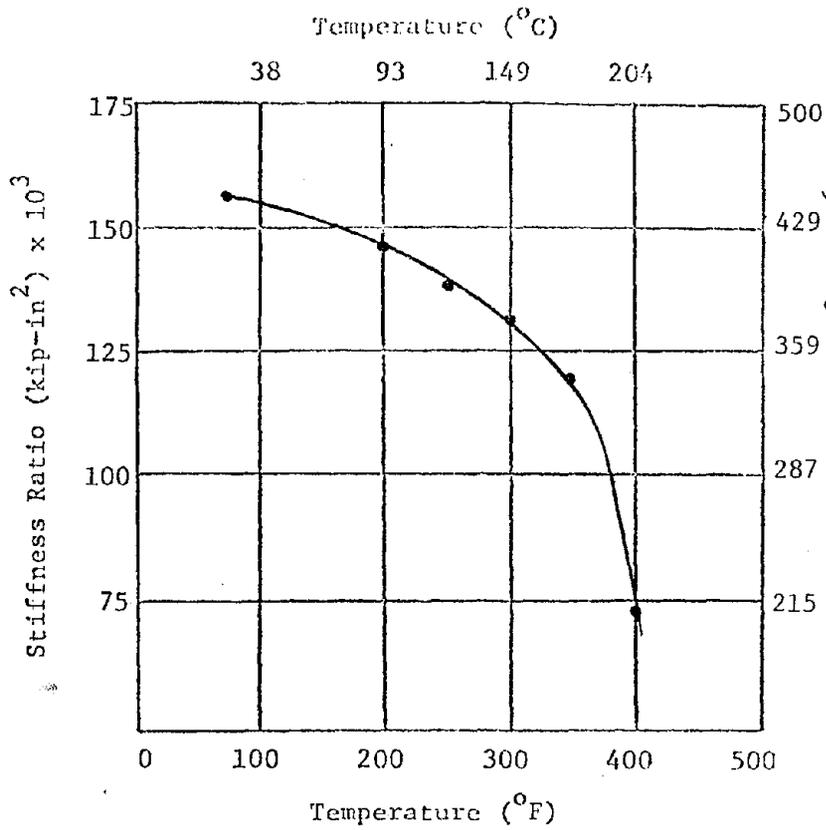
Figure 15: Effect of Temperature on Stiffness at P = 0 for Flexural Cracks (Hot Strength)
