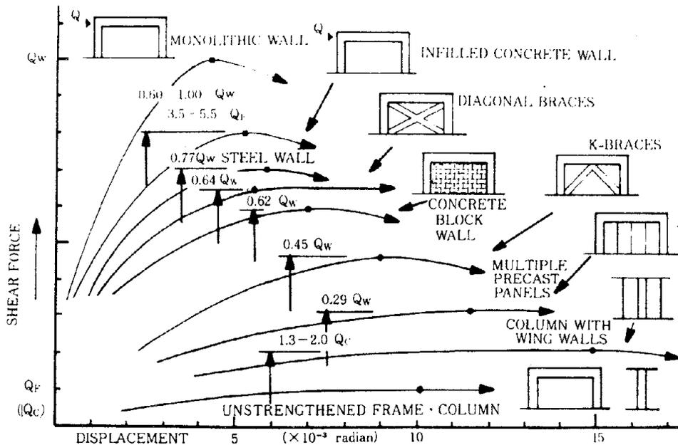
FIG. 10 TYPICAL LOAD-DISPLACEMENT RELATIONSHIPS FOR DIFFERENT STRENGTHENING TECHNIQUES
