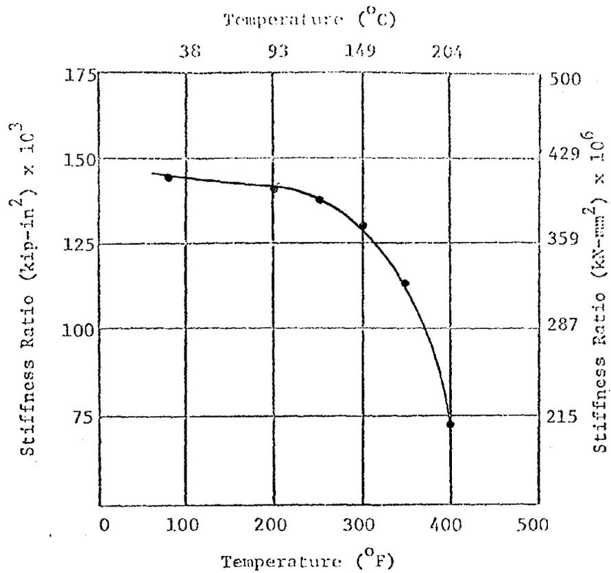
Figure 17: Effect of Temperature on Stiffness at  $P = 0.5 P_u$  for Flexural Cracks (Hot Strength)
