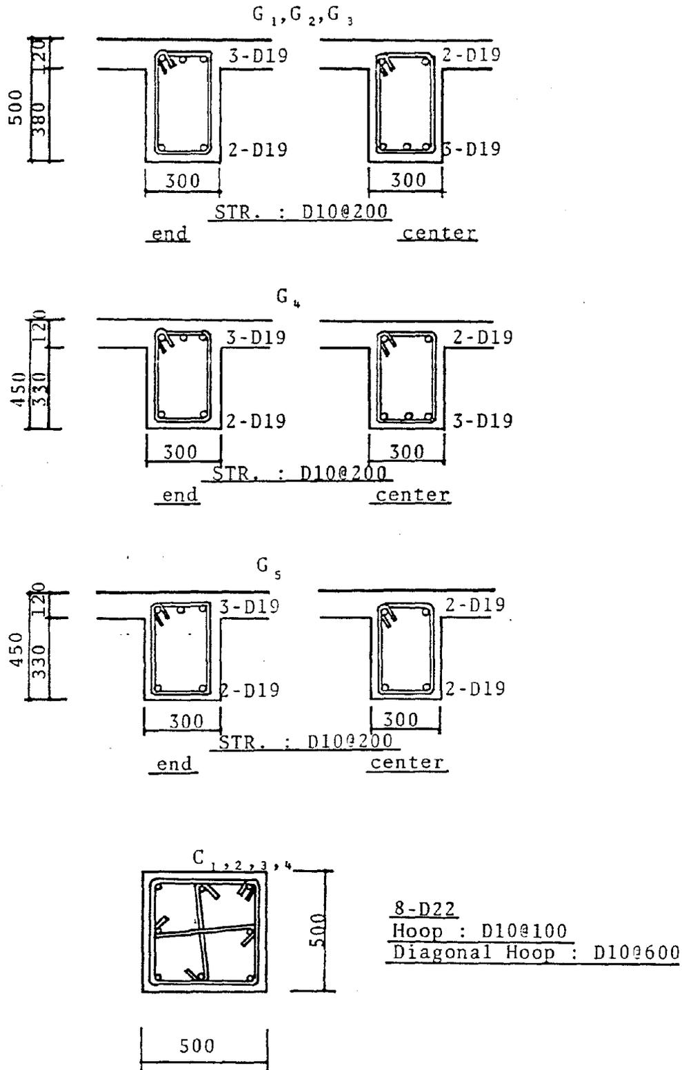
Fig. 2 : Longitudinal Reinforcement in Full-Scale Structure
