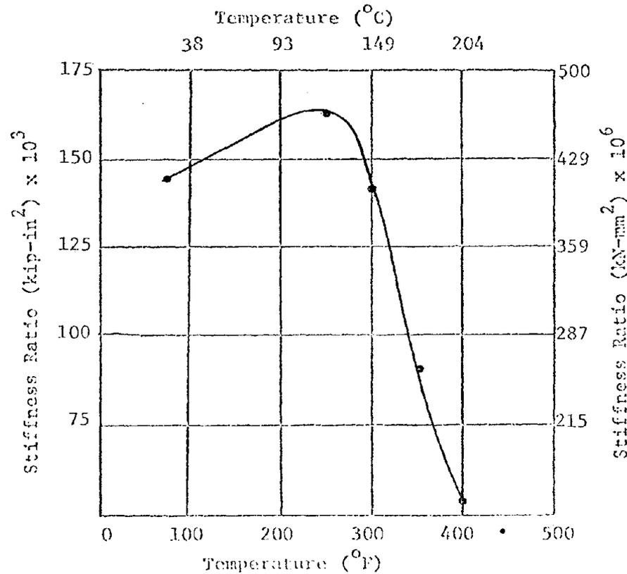
Figure 18: Effect of Temperature on Stiffness at  $P = 0.5 P_u$  for Flexural Cracks (Residual Strength)
