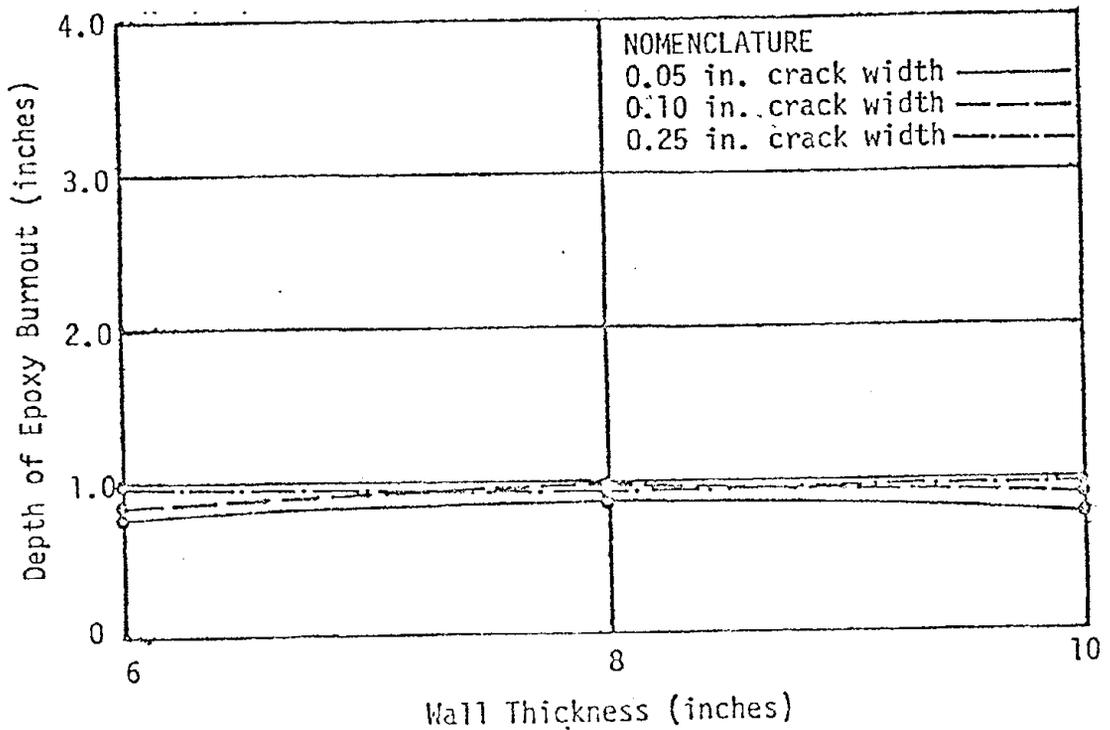
FIG. 2: AVERAGE DEPTH OF EPOXY BURNOUT AS A FUNCTION OF WALL THICKNESS FOR A 1-HOUR SDHI FIRE EXPOSURE
