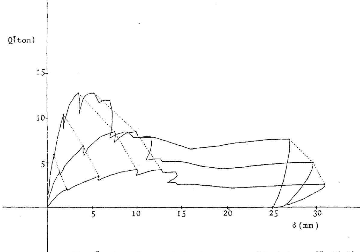
Fig. 8 Shear Force - Deflection Curve of Each Story (81-No.2)
