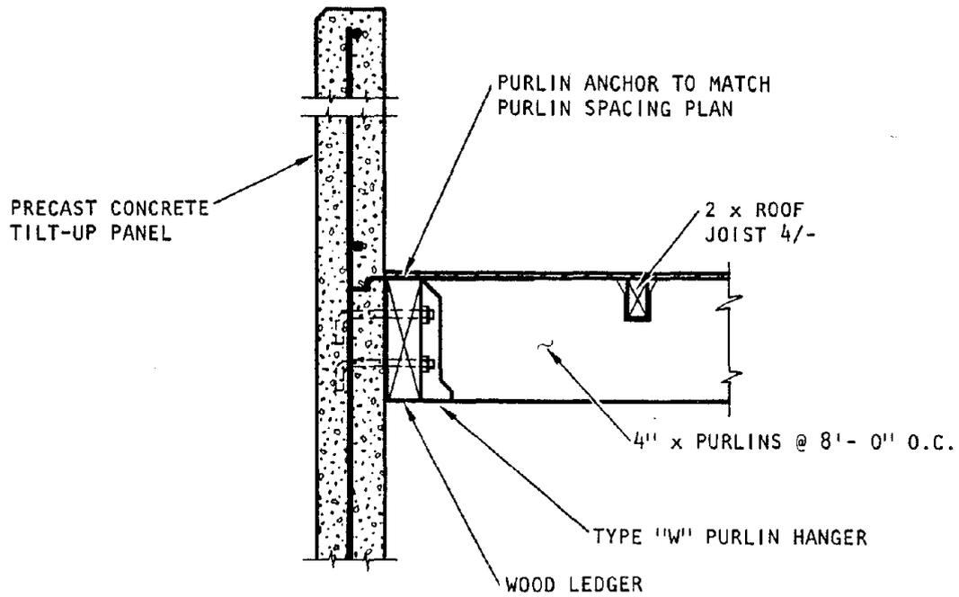
FIGURE 1. WOOD LEDGER AND WOOD PURLIN
