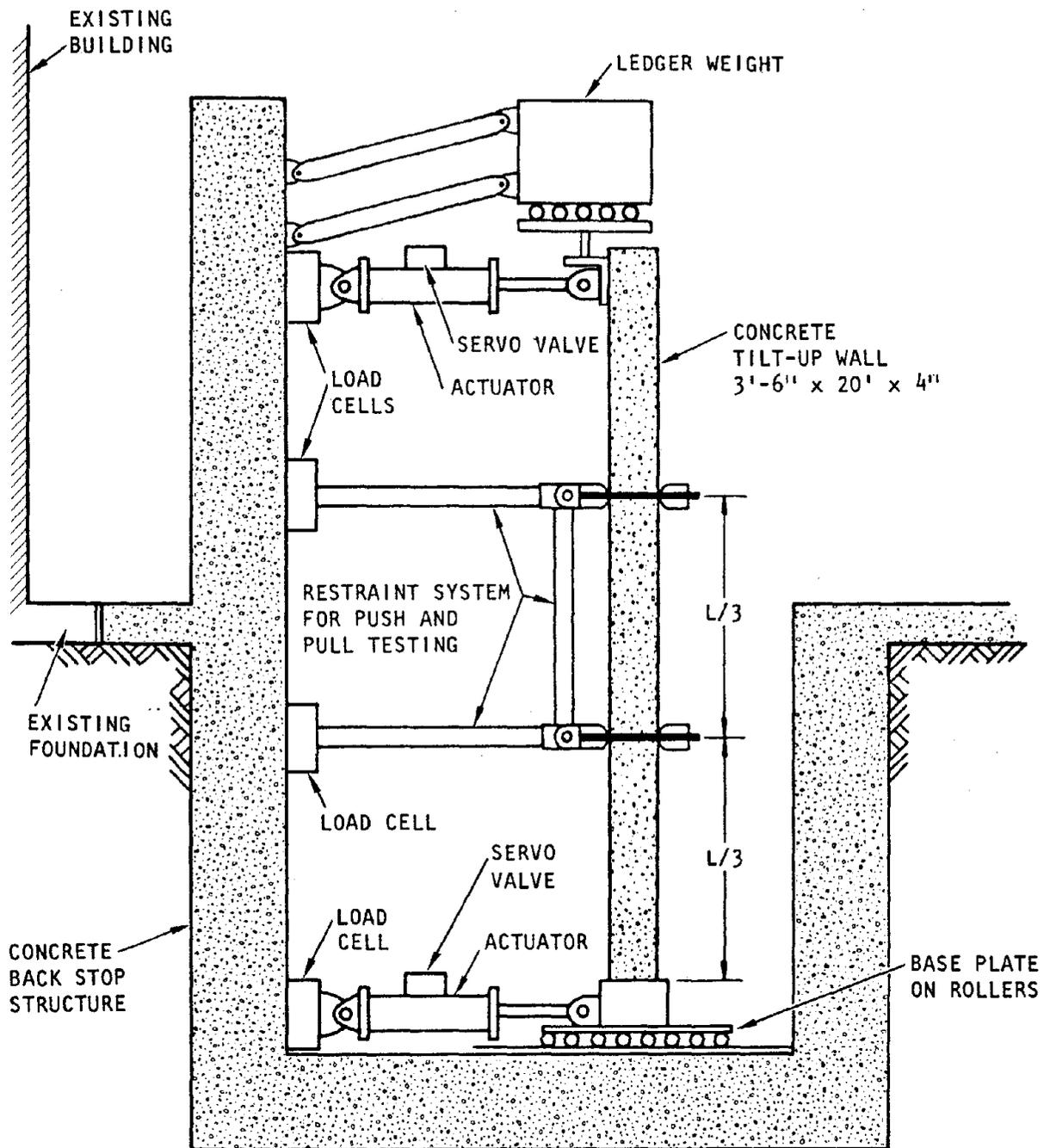
FIGURE 11. TEST SETUP FOR QUASI-STATIC TESTING OF WALLS IN THE DYNAMIC TEST FACILITY
