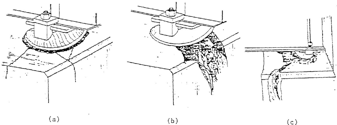
Fig-2 Fracture of shoe bed concrete
