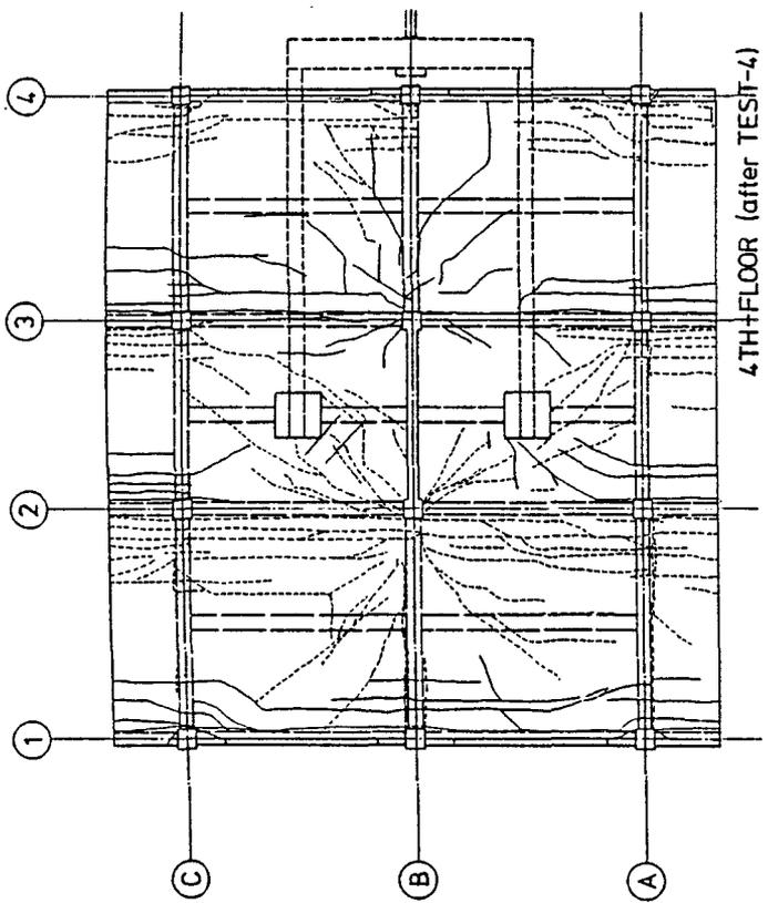
Fig. 22 Crack Pattern of 4th Floor (Test 488)
