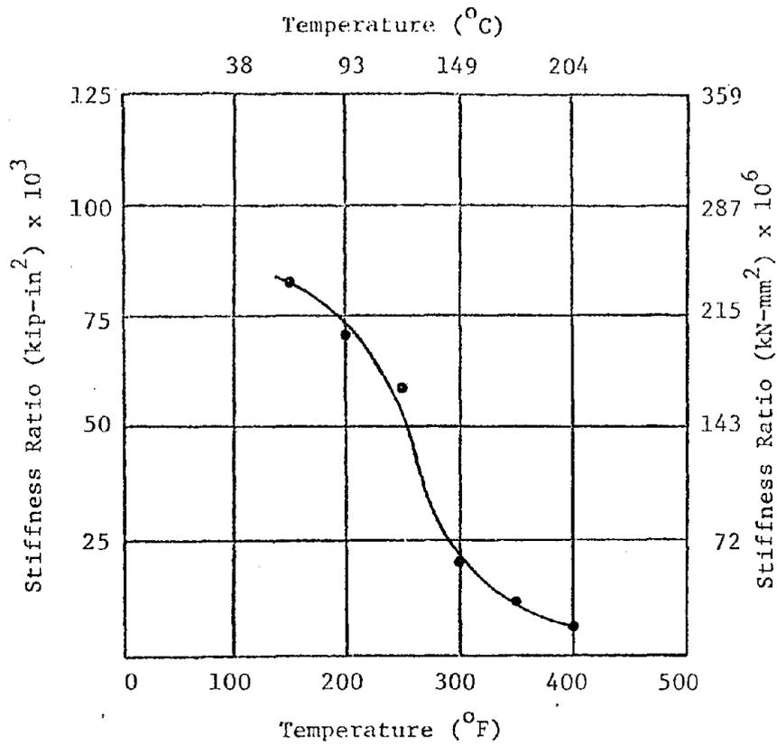
Figure 11: Effect of Temperature on Stiffness at  $P = 0$  for Shear Cracks (Hot Strength)
