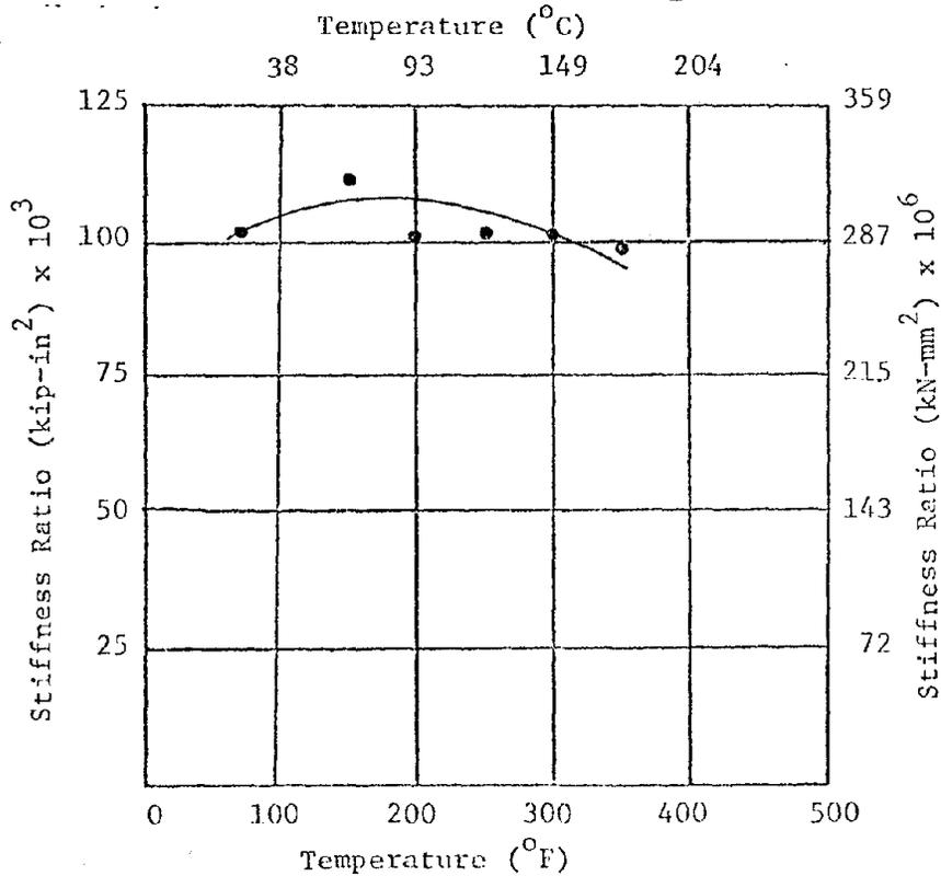
Figure 14: Effect of Temperature on Stiffness at  $P = 0.5 P_u$  for Shear Cracks Residual Strength)
