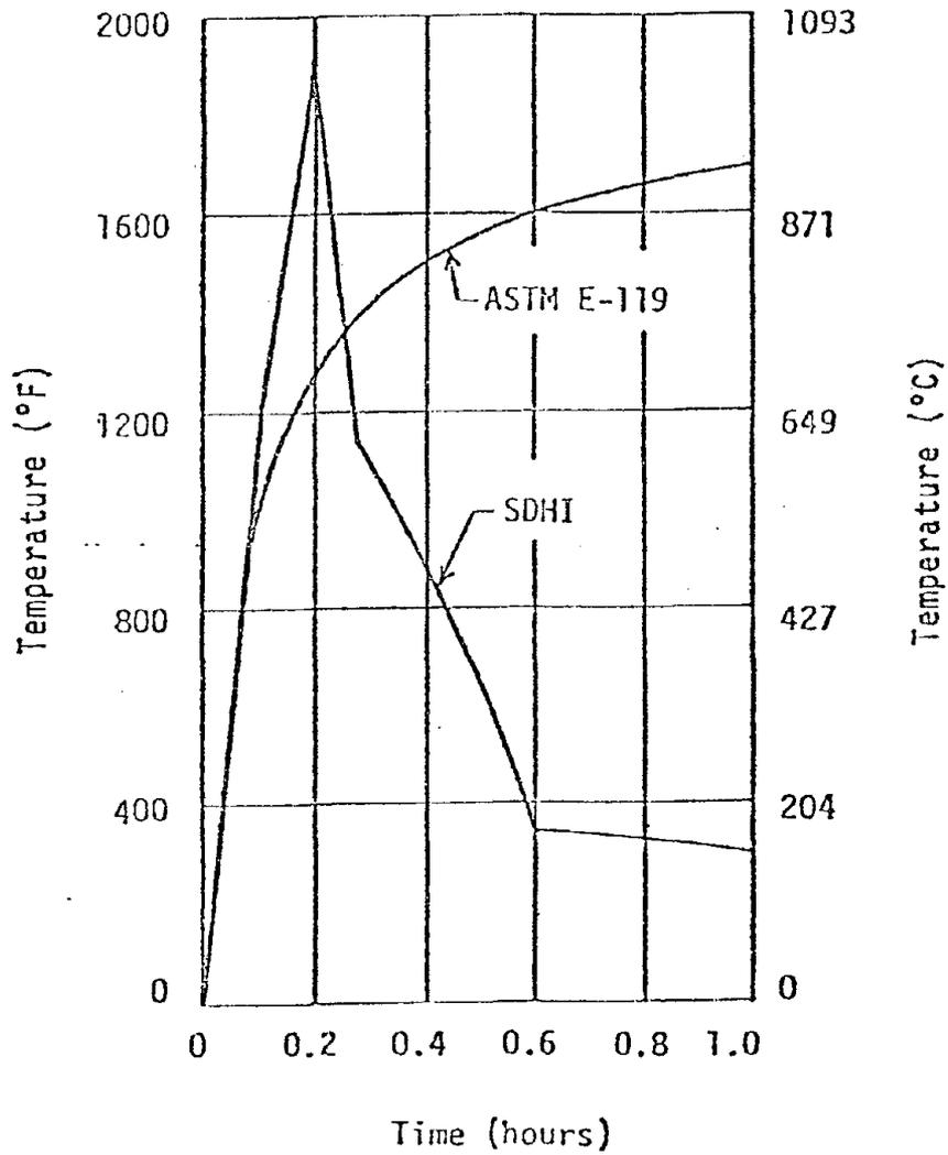
FIG. 5: ASTM E-119 AND SDHI TIME TEMPERATURE CURVES
