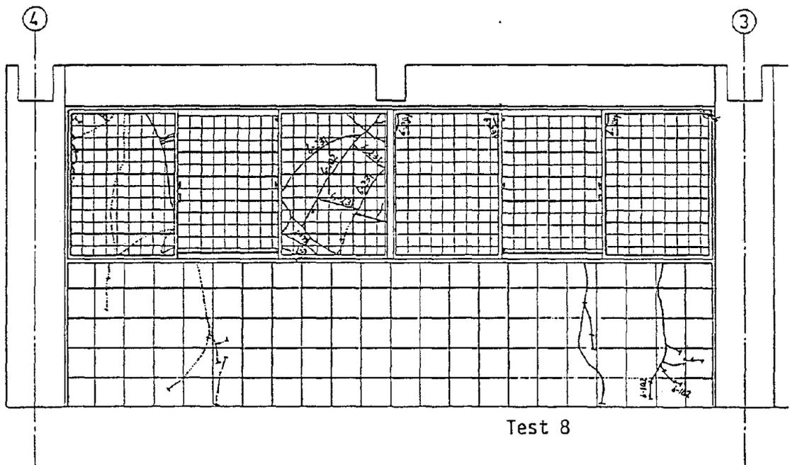
Fig. 25 Damage of Glasses & Spandrel Wall
