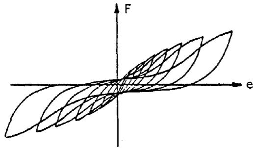
(a) Typical cyclic load deflection diagram for plywood diaphragms
