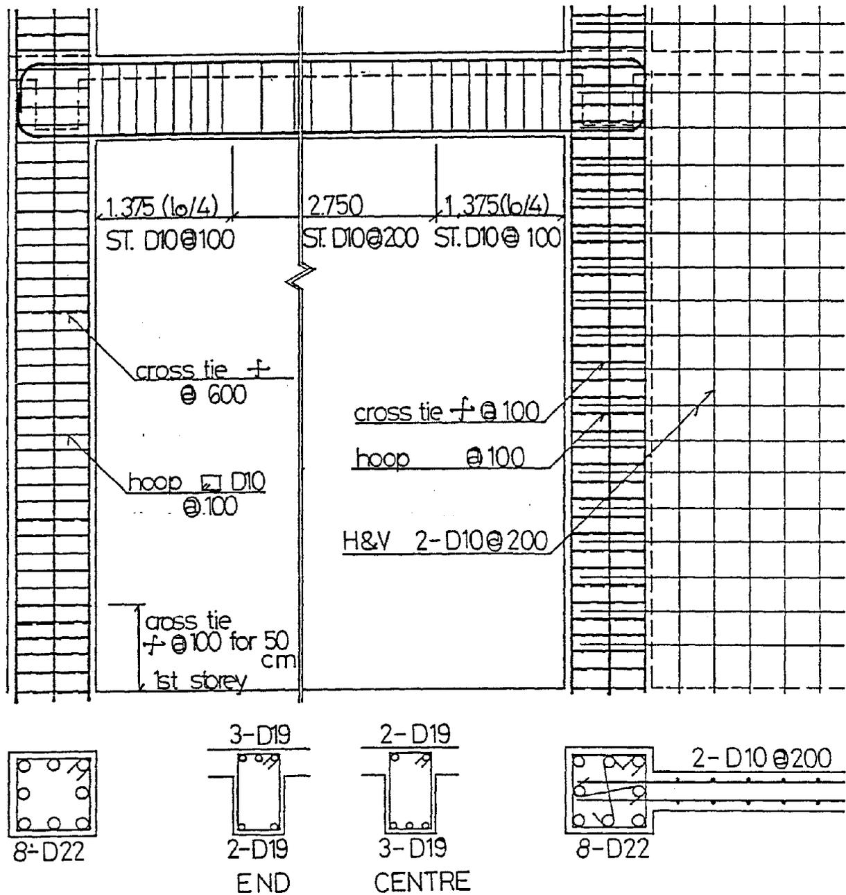
Fig. 2 Details of Reinforcing First Floor
