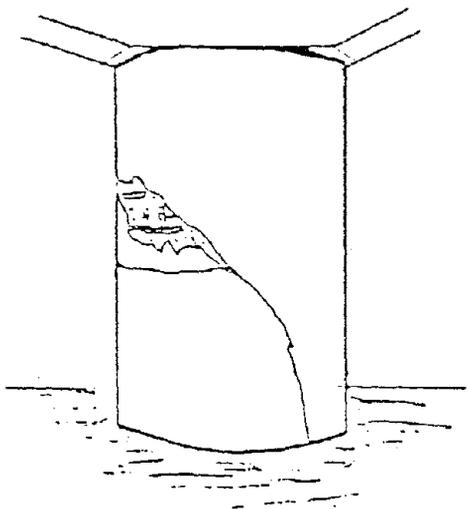
Fig-10 Flaking off of concrete
