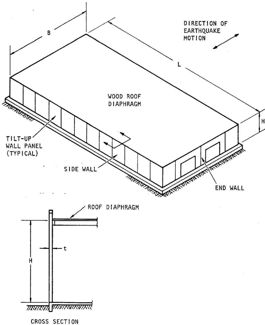
FIGURE 3. ONE-STORY TILT-UP-WALL BUILDING WITH A WOOD ROOF DIAPHRAGM
