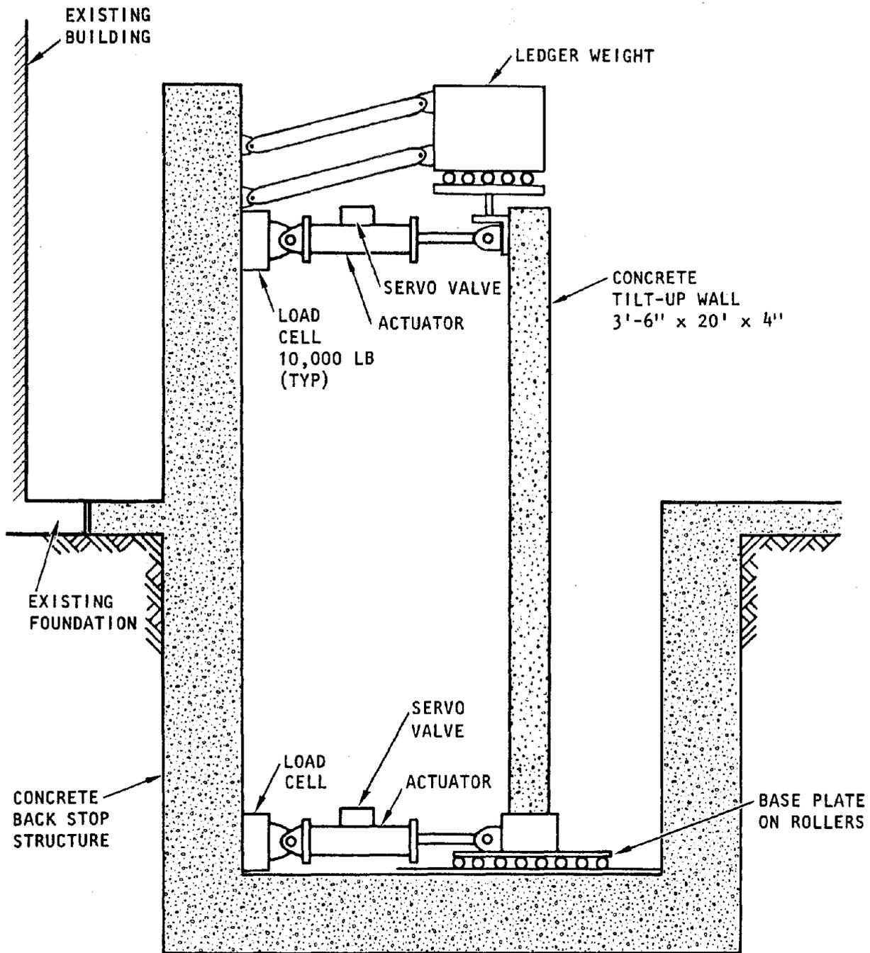
FIGURE 10. TEST SETUP FOR DYNAMIC TESTING OF WALLS
