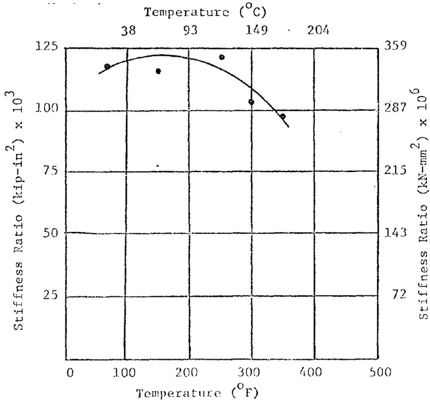
Figure 12: Effect of Temperature on Stiffness at  $P = 0$  for Shear Cracks (Residual Strength)
