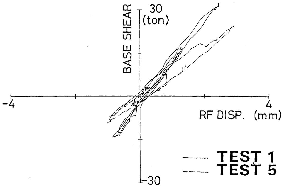
Fig. 9 Total Shear Force vs. RF Displacement Relationship
