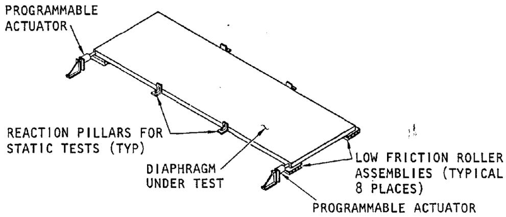
(a) Test setup for quasi-static testing of diaphragms
