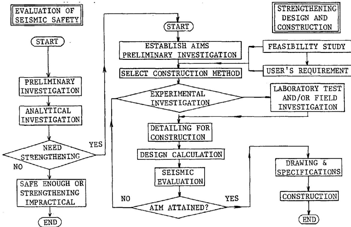
FIG. 2 FLOW CHART OF DESIGN AND CONSTRUCTION OF SEISMIC STRENGTHENING
