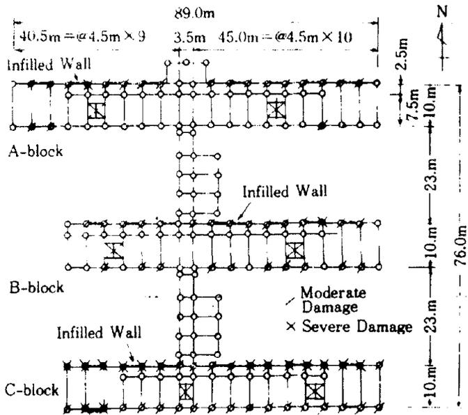
FIG. 14 STRENGTHENING OF THE DAMAGED SCHOOL BUILDING "B"
