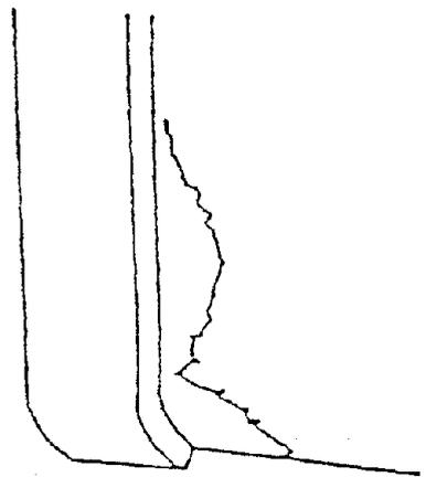
Fig-9 Horizontal cracking
