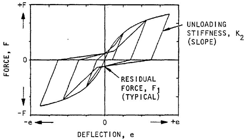
(c) Typical cyclic load-deflection diagram for model
