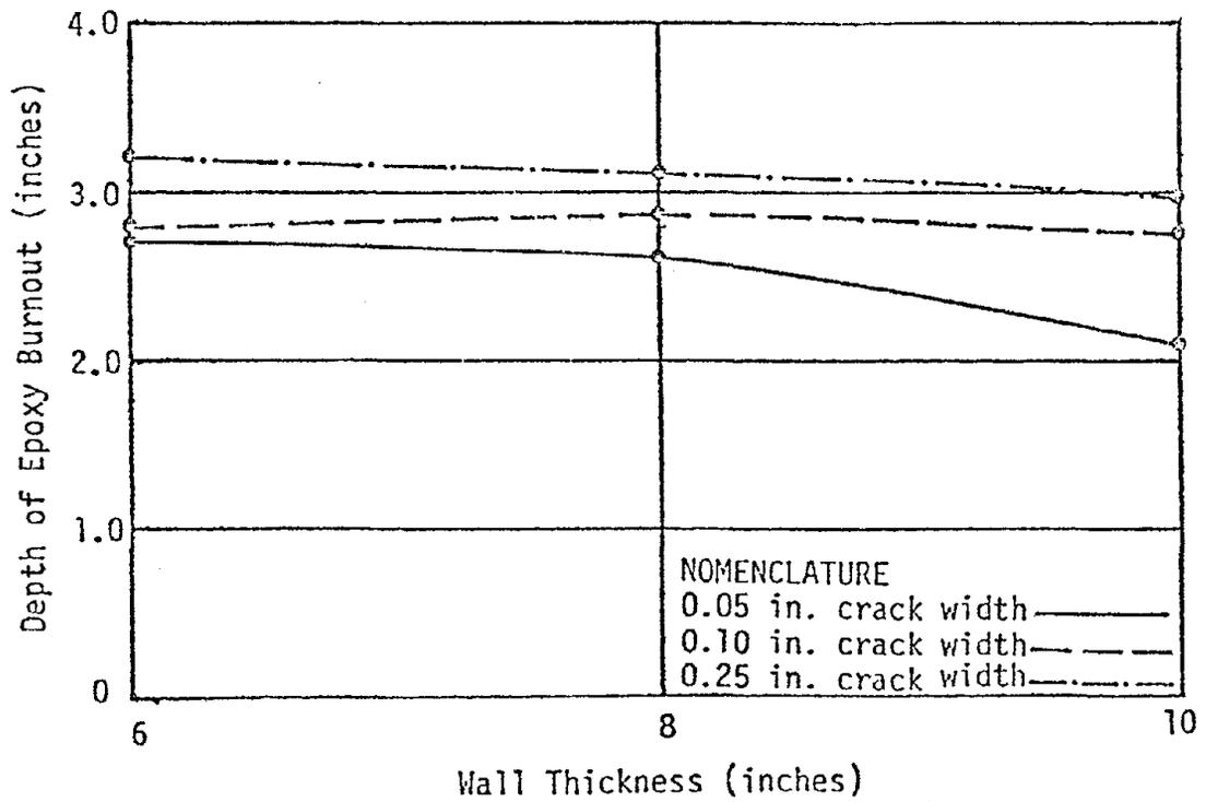
FIG. 1: AVERAGE DEPTH OF EPOXY BURNOUT AS A FUNCTION OF WALL THICKNESS FOR 2-HOUR ASTM E-119 FIRE EXPOSURE
