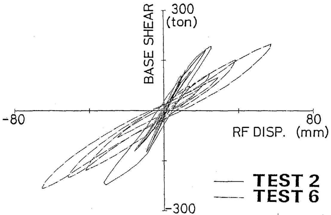
Fig. 10 Total Shear Force vs. RF Displacement Relationship
