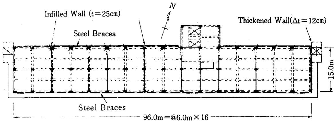
FIG. 13 STRENGTHENING OF THE DAMAGED SCHOOL BUILDING "A"
