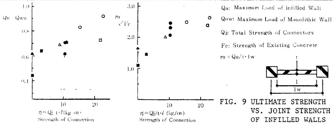
FIG. 9 ULTIMATE STRENGTH VS. JOINT STRENGTH OF INFILLED WALLS
