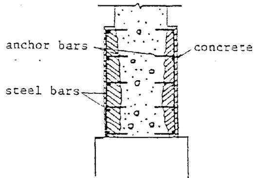
Fig-15 Supplemental reinforced concrete
