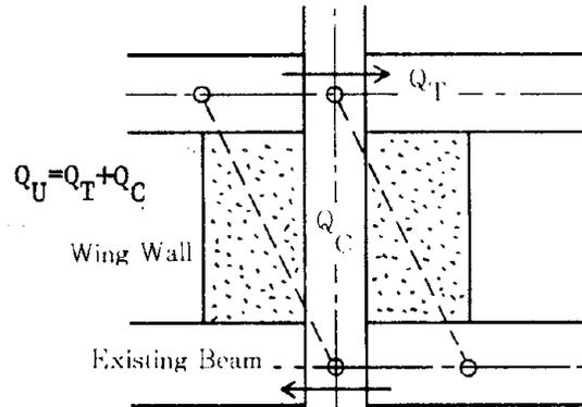
(b) WING WALLS WITH DOWEL CONNECTIONS
