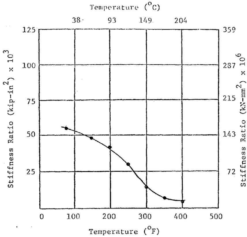
Figure 13: Effect of Temperature on Stiffness at  $P = 0.5 P_u$  for Shear Cracks (Hot Strength)
