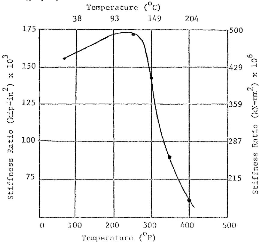
Figure 16: Effect of Temperature on Stiffness at P = 0 for Flexural Cracks (Residual Strength)
