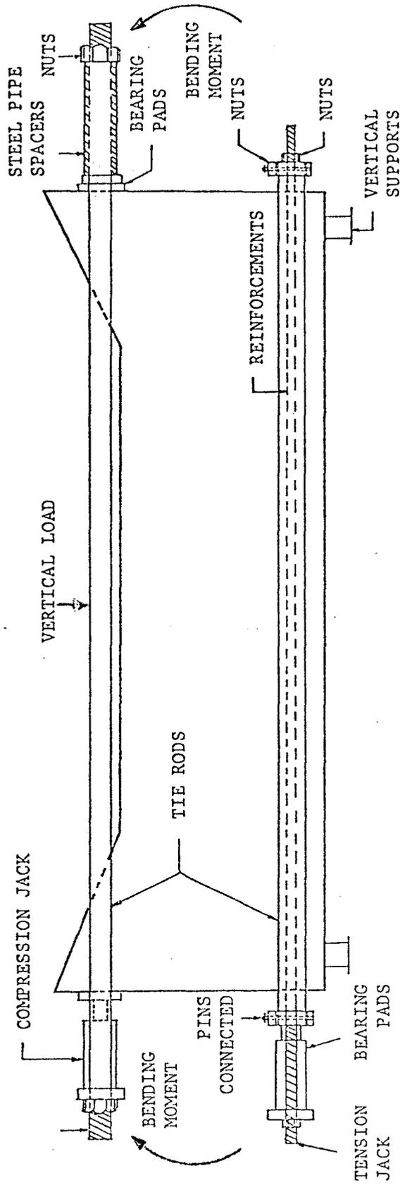
FIG. 4: GEOMETRY, REINFORCEMENT, AND LOADING PROCEDURE FOR INTERMEDIATE-SCALE SPECIMENS
