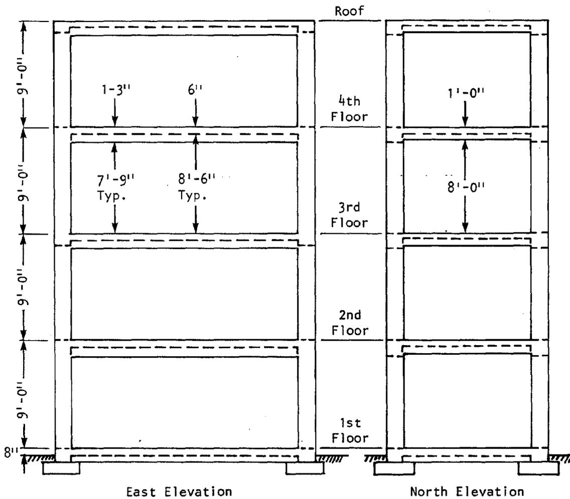
FIGURE 1 4-STORY CONCRETE TEST STRUCTURE
