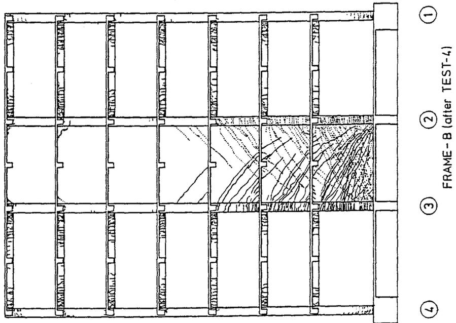
Fig. 21 Crack Pattern of Frame-B (Test 4&8)
