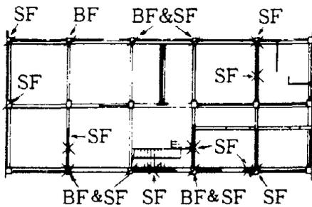
BF; Bending Failure
