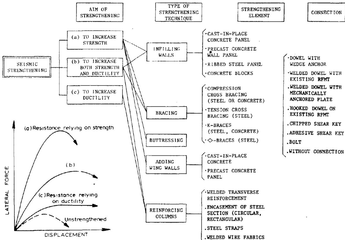
FIG. 3 CONCEPT OF SEISMIC STRENGTHENING AND TYPICAL STRENGTHENING METHODS
