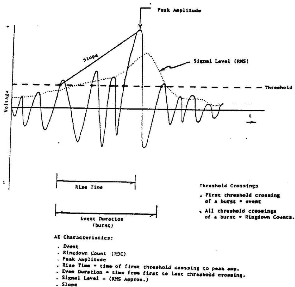
Figure 1 Stress Wave Characteristics
