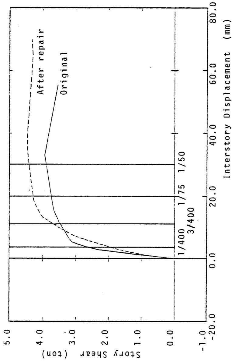
Fig. 18 Envelope Curve of Specimen I-1
