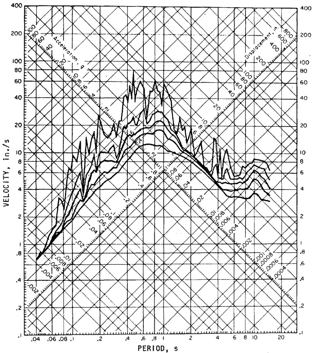
FIGURE 7. RESPONSE SPECTRUM OF SAN FERNANDO EARTHQUAKE, 9 FEBRUARY 1971: CASTAIC OLD RIDGE ROUTE, COMP N69W (Damping values are 0, 2, 5, 10, and 20 percent of critical—unscaled)
