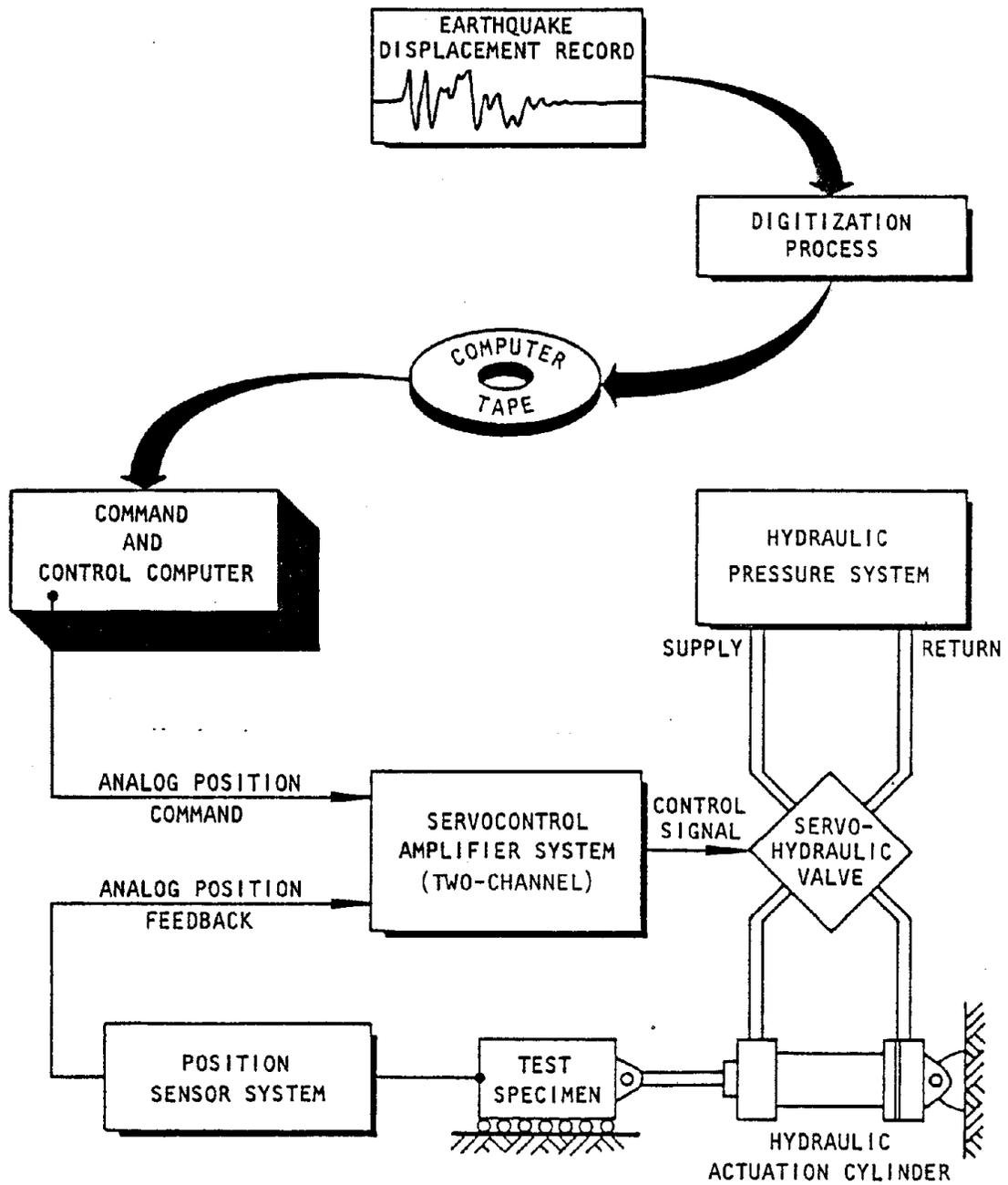
FIGURE 13. DISPLACEMENT-CONTROLLED HYDRAULIC ACTUATION SYSTEM
