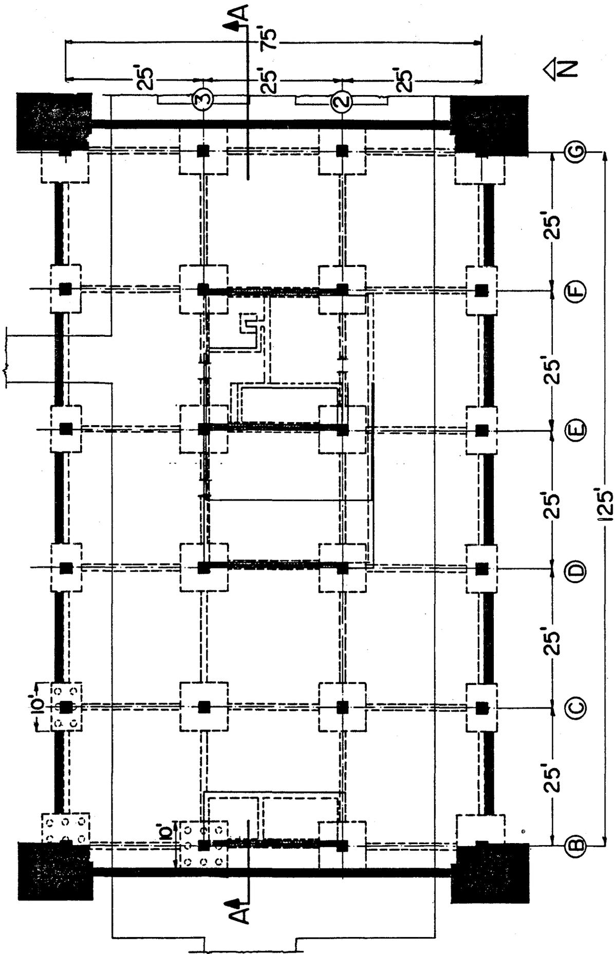
Fig. 4 FOUNDATION PLAN OF IMPERIAL COUNTY SERVICES BUILDING
