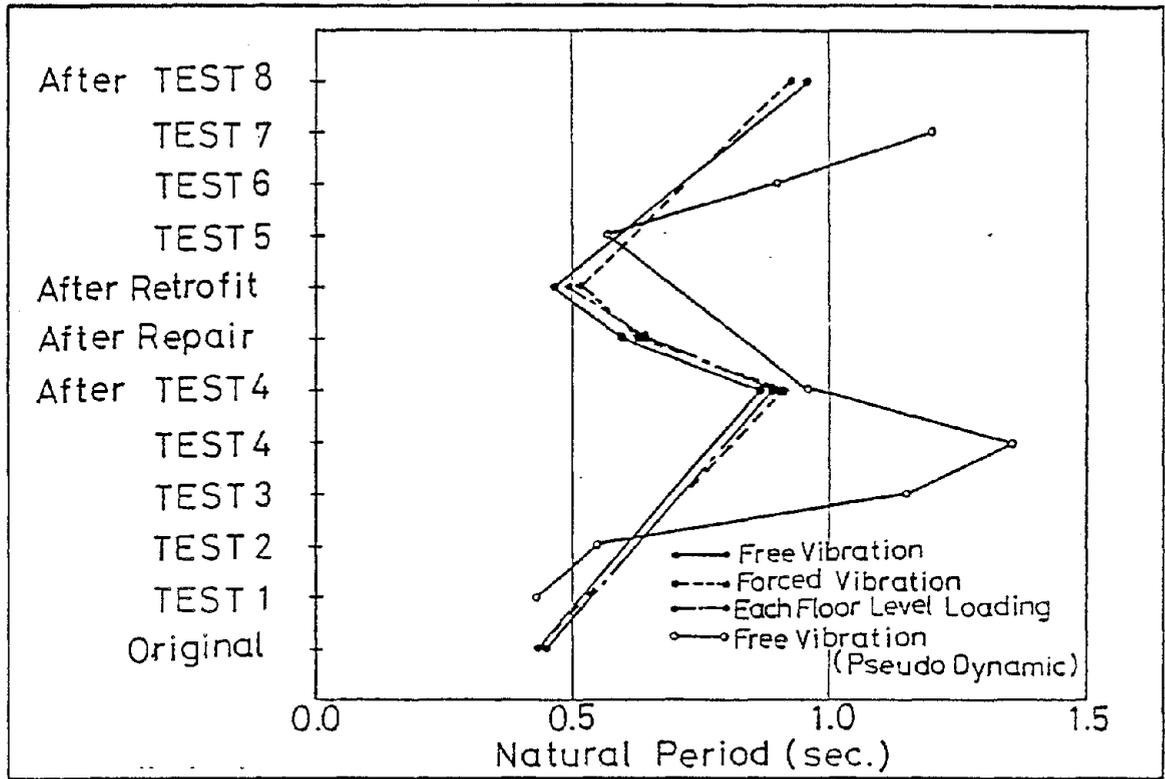
Fig. 26 Transition of Measured Natural Period by Vibration Test
