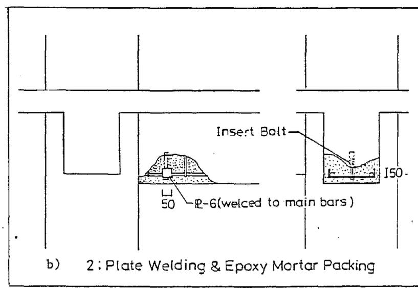
Fig. 4 Details of Repair Works at Beam End
