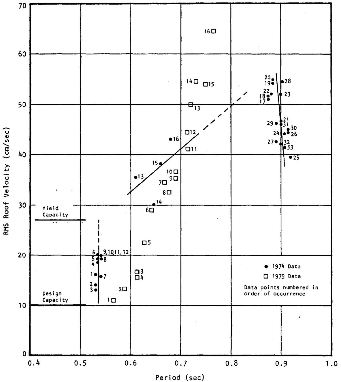
FIGURE 4 VELOCITY VERSUS PERIOD FOR THE DESTRUCTIVE TEST, LONGITUDINAL DIRECTION
