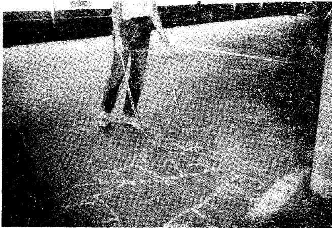
Figure 1 - Chain Drag to Determine Delamination by Sound
