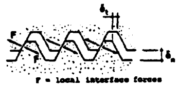
Fig.2a - Wedge effect: crack response depends on the ratio r = \delta_t/\delta_n .
