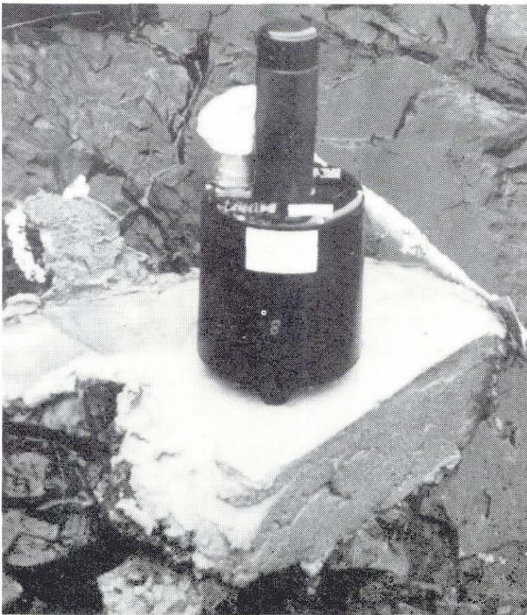
FIG. 2.10 Ranger Seismometer In Position On The Abutment Rock
