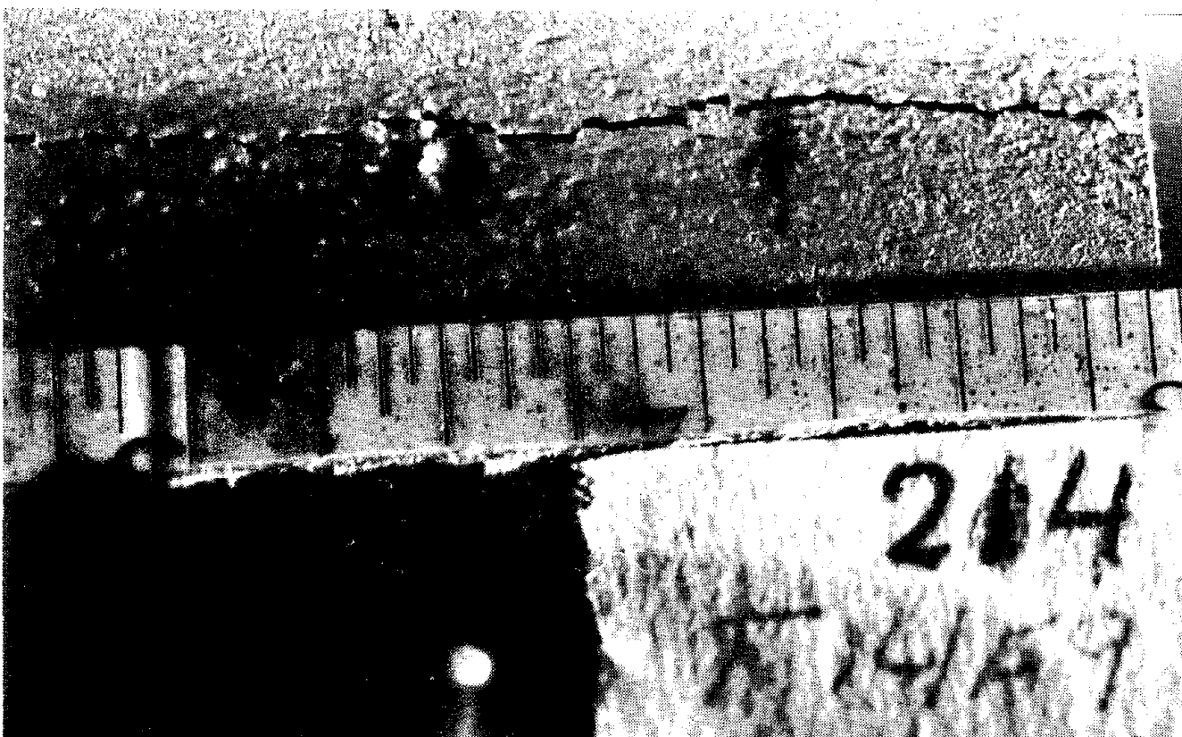
d. CRACK PATTERN AT 214 CYCLES
