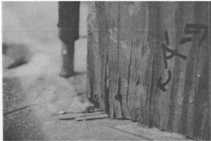
Figure 43: Specimen PD-4 Run No. 2 Crumbling of Plywood @ Lower Front Corner Test No. A-9, A-10, Frequency = 0.5 Hz Peak Command Displacement = \pm 2 Inches, \pm 2\text{-}1/2 Inches
