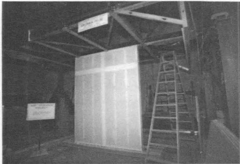
Figure 4A: Specimen PD3-V Run No. 1 Test No. A-2, Frequency = 0.5 Hz Peak Command Displacement \pm 1/4 Inch Damage - Loosening of Bottom Line of Nails
