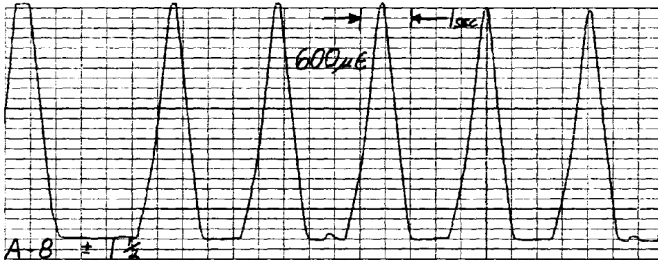
STRAIN GAGE @ RIGHT HOLDOWN BOLT
