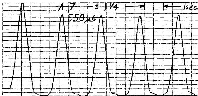
STRAIN GAGE @ LEFT HOLDOWN BOLT
