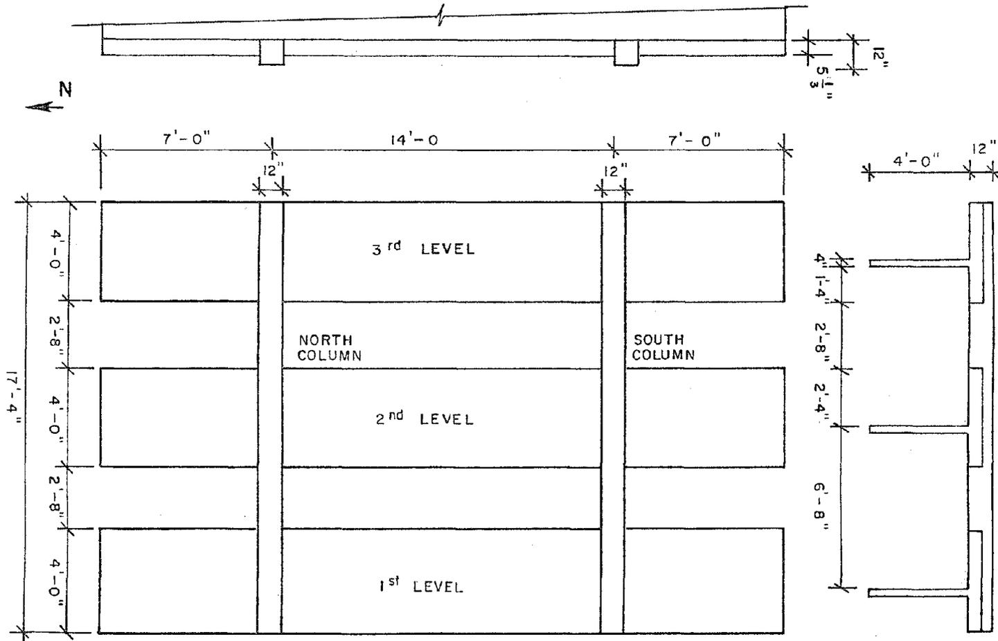
Fig. 2.9 Test Specimen (existing structure) - two bays between 3rd and 5th stories of exterior moment resisting frame
