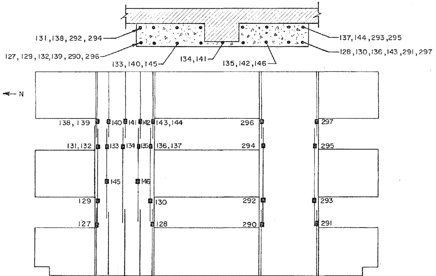
Fig. 2.50 Strain gage locations on the longitudinal reinforcement in the pier
