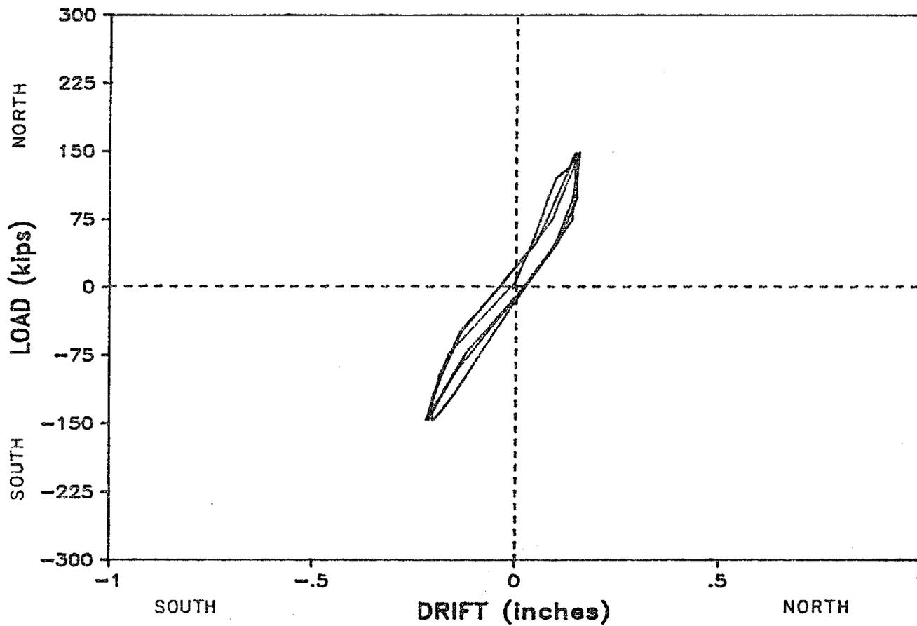
Fig. 3.4 Load vs. drift for three cycles to low (0.125%) drift
