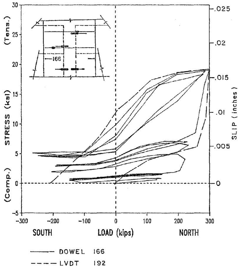
Fig. 4.18 Load vs. stress for dowel 166 and load vs. slip for LVDT 192.
