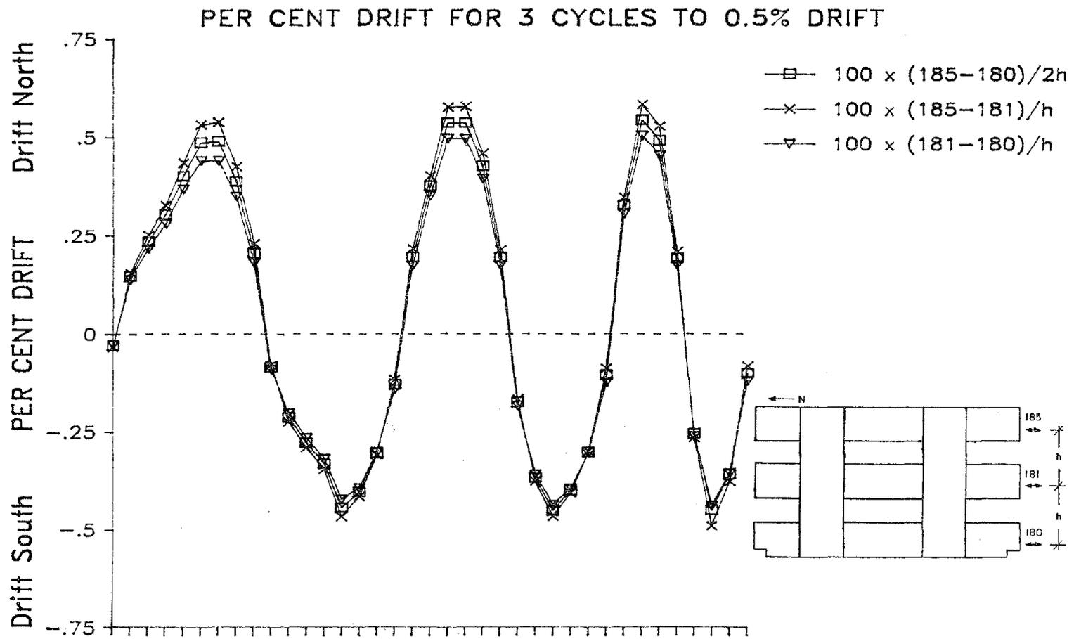
Fig. 4.1 Interstory drift for last three cycles of loading
