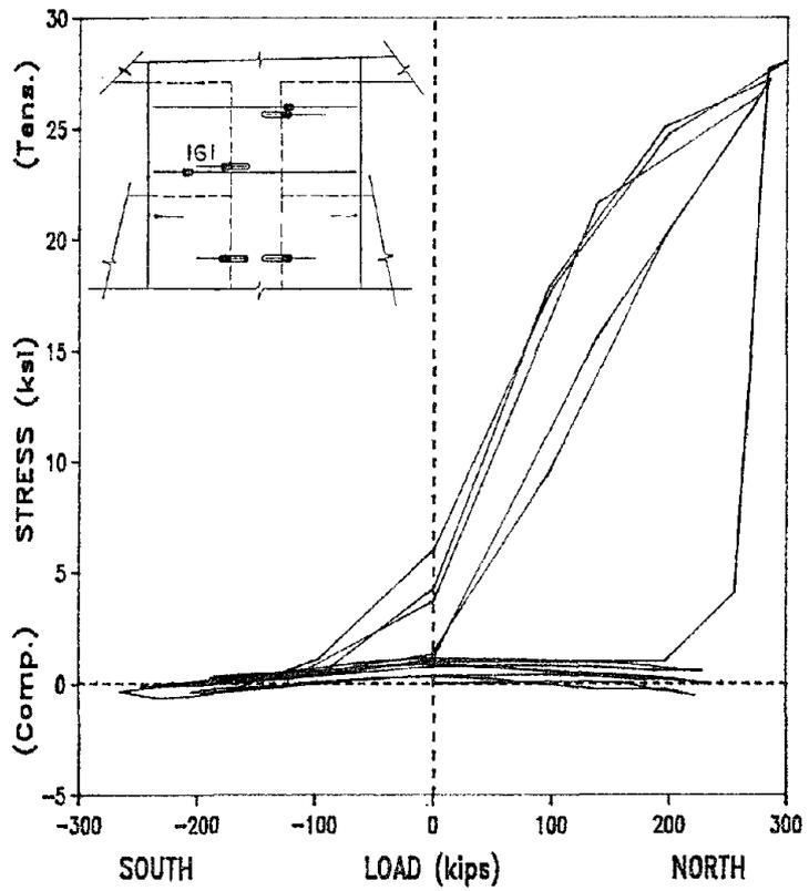
Fig. 4.20 Load vs. stress for dowel 161
