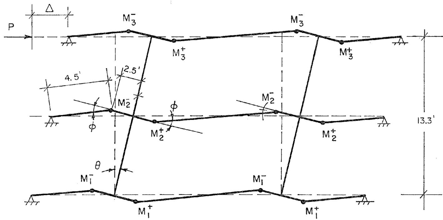
Fig. 5.1 Idealized failure mechanism for all beams hinged and infinitely stiff columns
