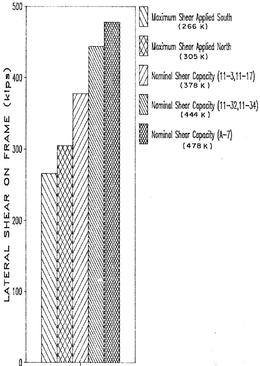
Fig. 5.4 Comparison of maximum shear applied to the piers and the calculated nominal strengths of the piers
