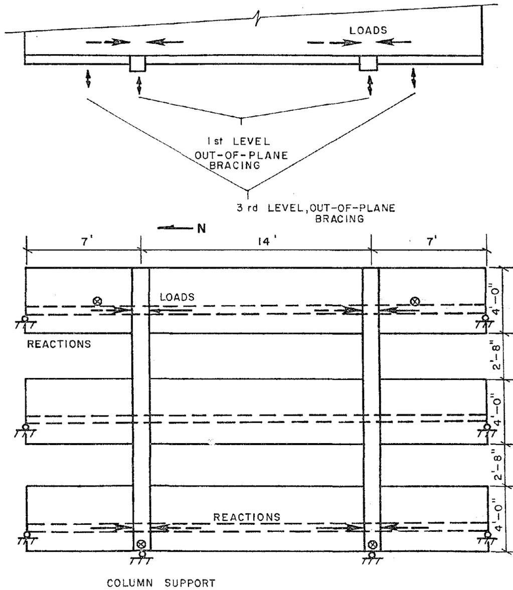
Fig. 2.11 Boundary constraints modeled on test specimen
