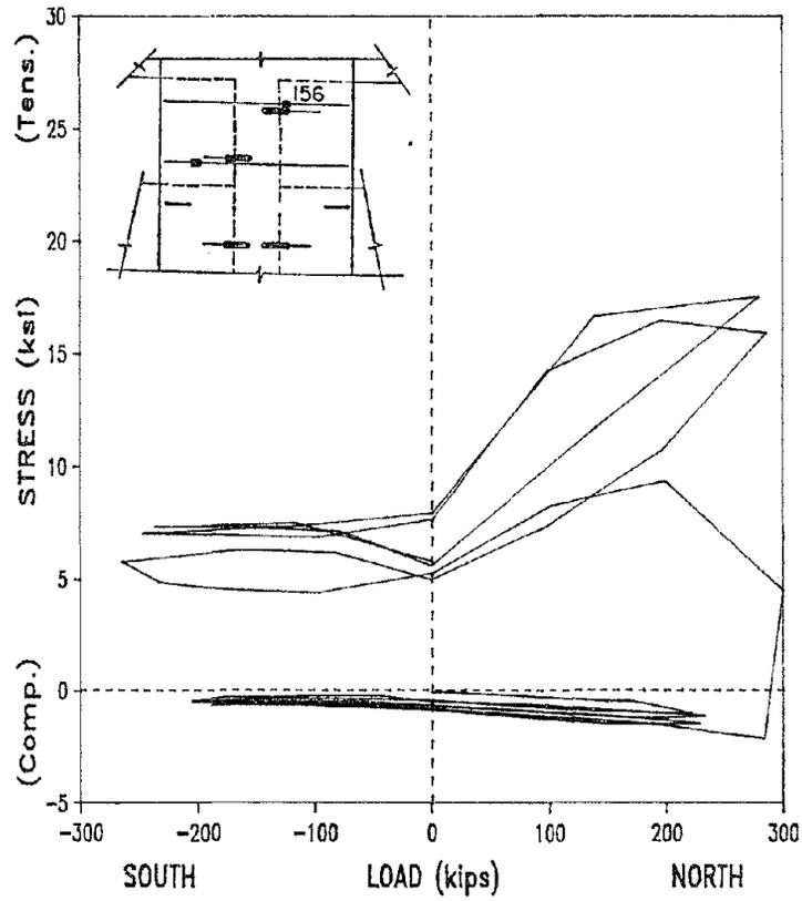
Fig. 4.27 Load vs. stress for stirrup gage 156
