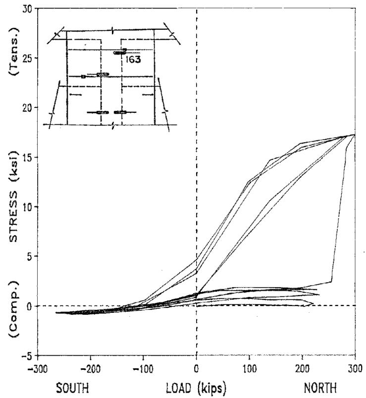
Fig. 4.21 Load vs. stress for dowel 163
