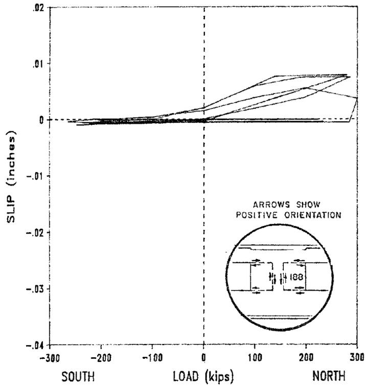
Fig. 4.16 Load vs. slip for LVDT 188
