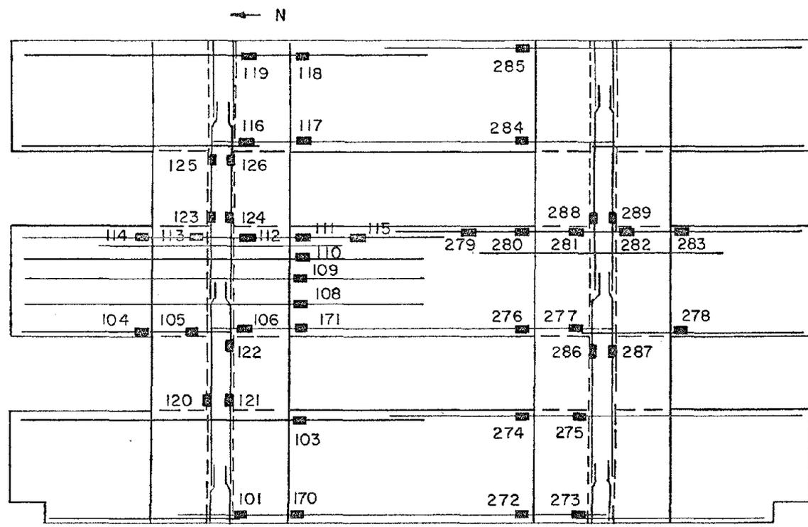
Fig. 2.49 Strain gage locations in the original frame
