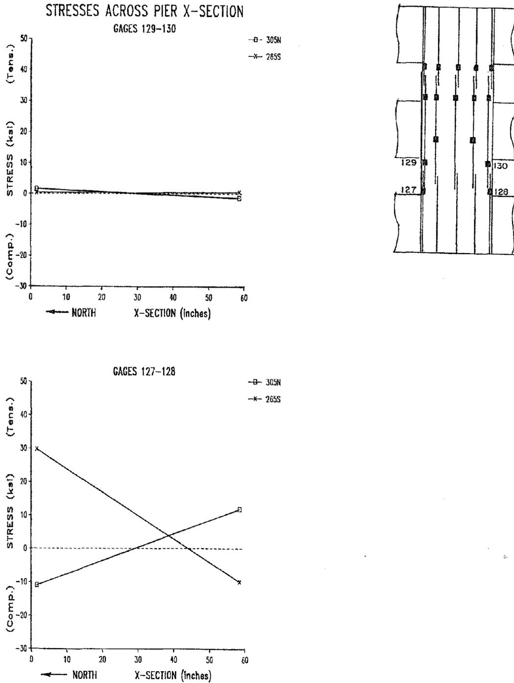
Fig. 4.5 Stress gradients across top and bottom cross sections of north pier, first level
