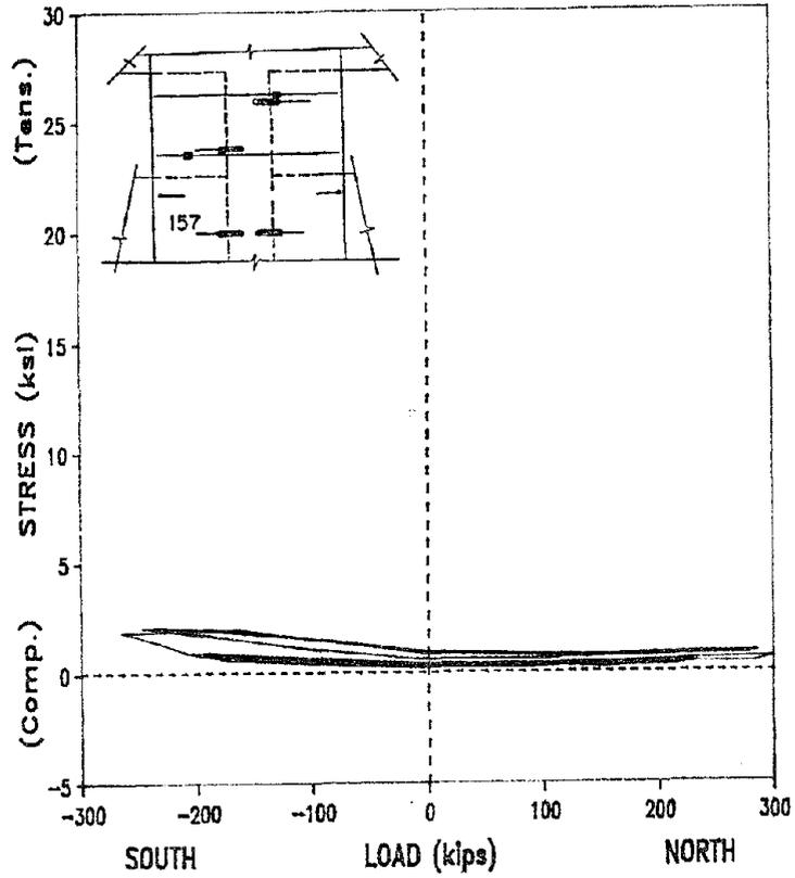
Fig. 4.22 Load vs. stress for dowel 157
