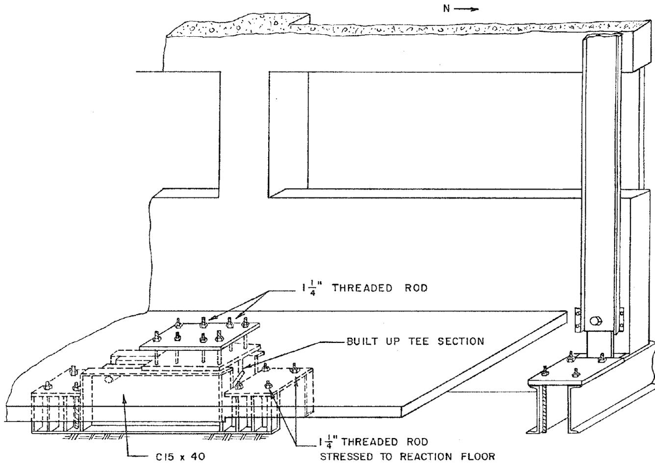
Fig. 2.42 Reaction assemblage under first level slab
