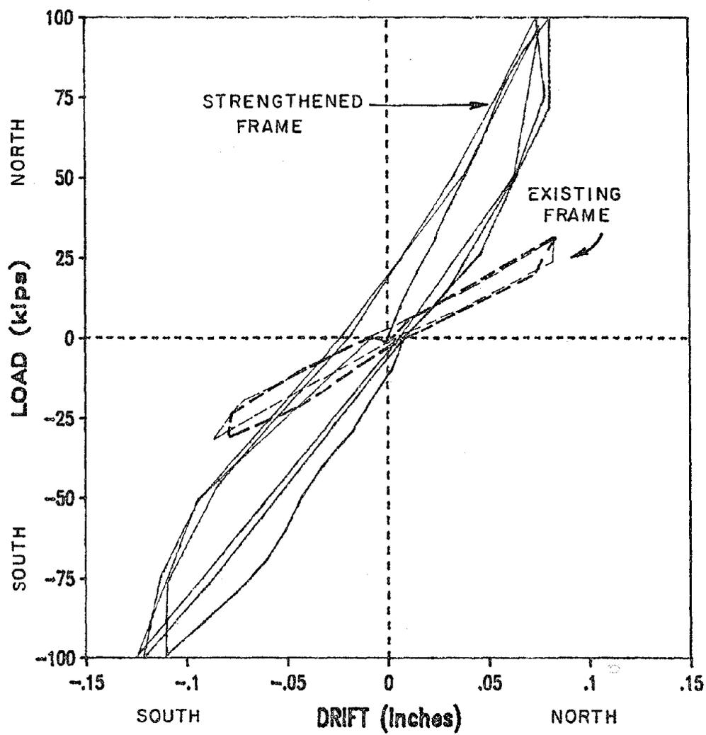
Fig. 3.3 Load vs. drift for the strengthened frame and existing frame models for cycles to 0.05% drift
