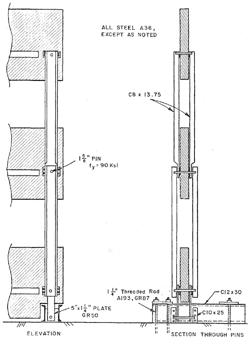
Fig. 2.46 Steel struts to provide vertical deflection restraints at ends of beams
