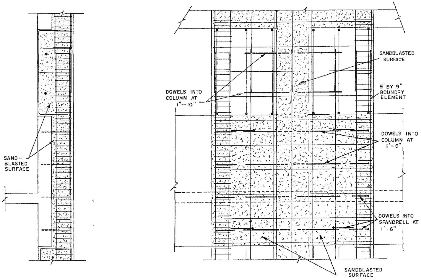
Fig. 2.6 Reinforcement in pier
