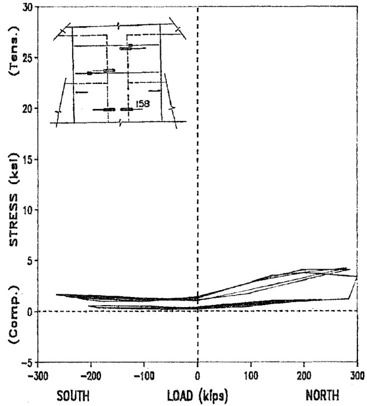
Fig. 4.23 Load vs. stress for dowel 158
