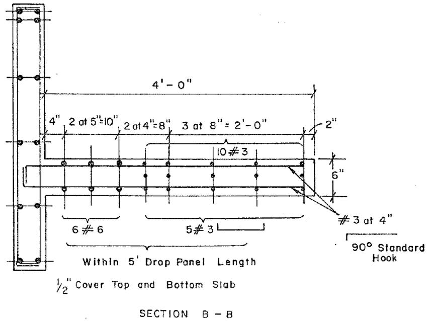
Fig. 2.13 Section through slab and drop panel
