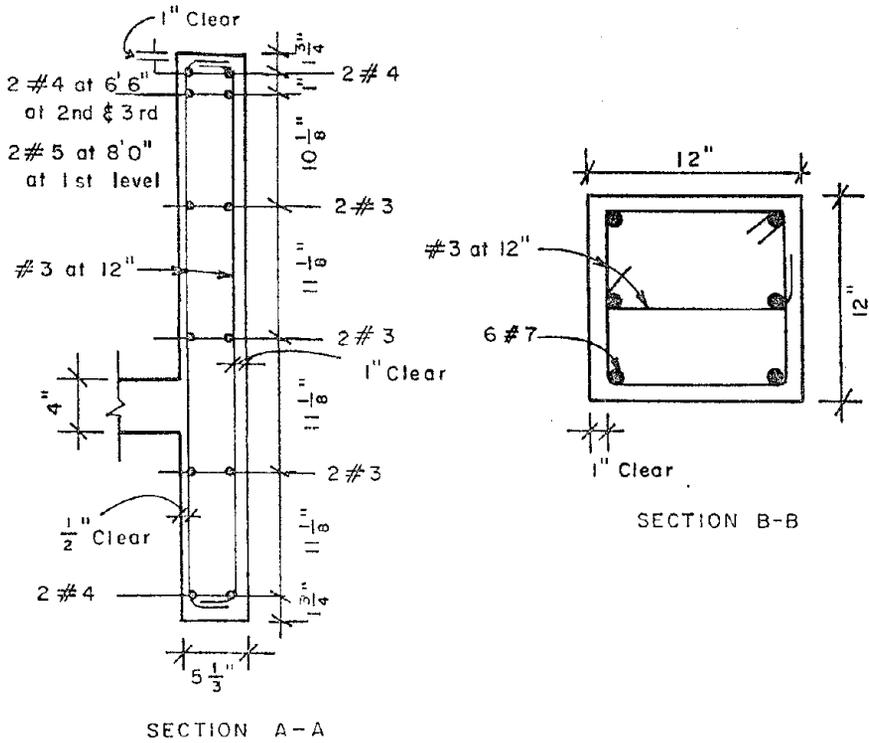
Fig. 2.10 Details of 2/3 scale model of existing frame.
