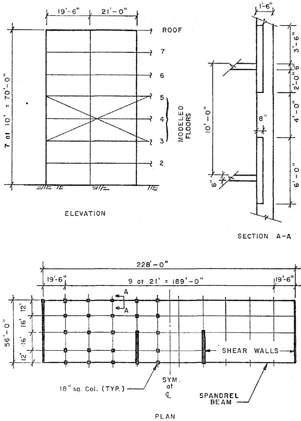
Fig. 2.1 Prototype building, plan and elevation
