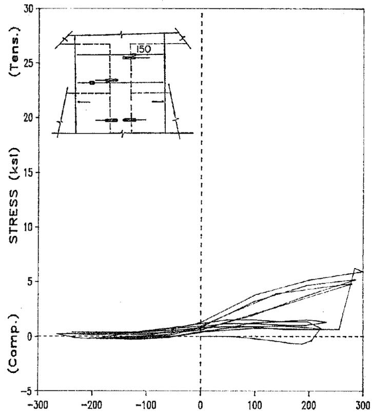
Fig. 4.26 Load vs. stress for stirrup gage 150
