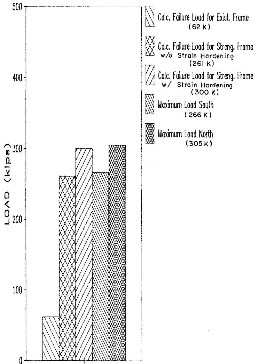
Fig. 5.3 Comparison of model with the calculated failure load of the existing frame model, the predicted failure load of the strengthened frame and the maximum loads on the frame
