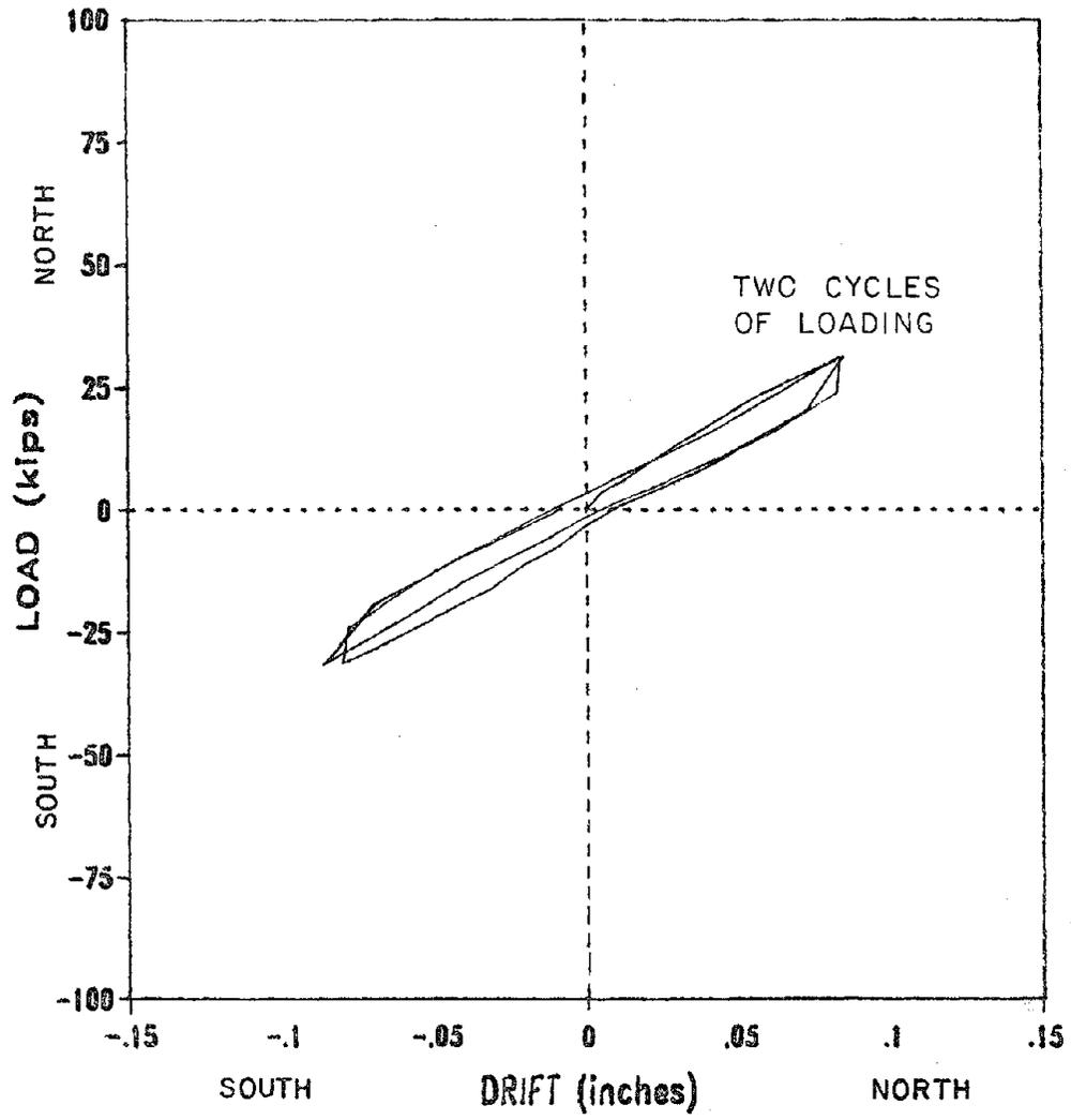
Fig. 3.1 Load vs. drift for test of existing frame model
