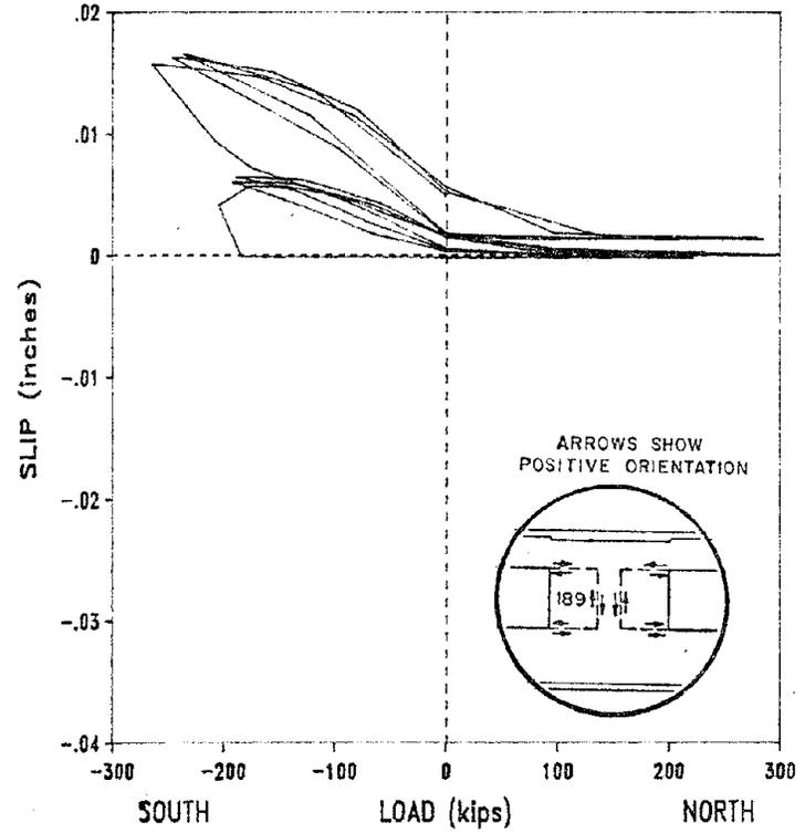
Fig. 4.17 Load vs. slip for LVDT 189
