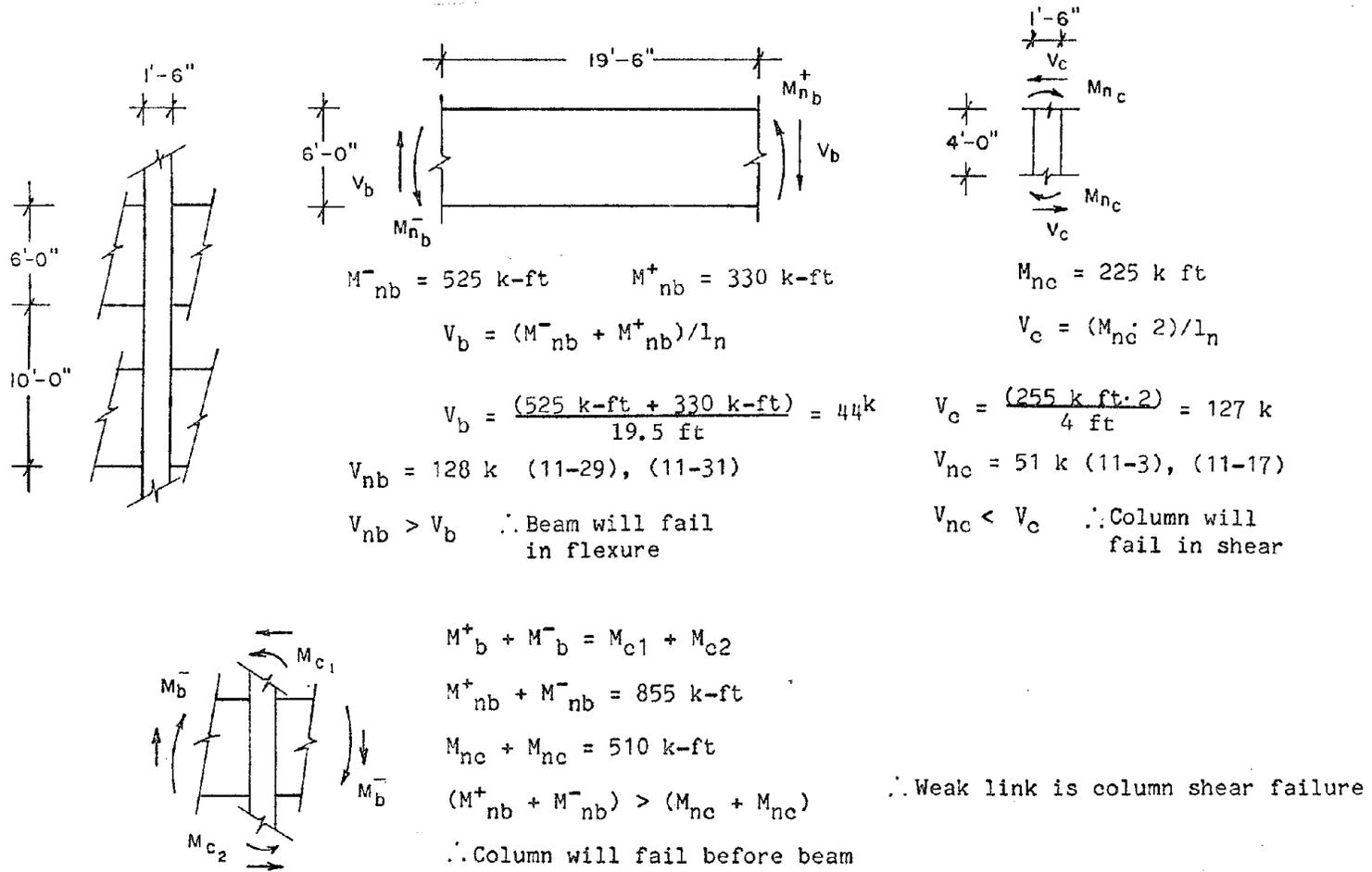
Fig. 2.4 Evaluation of exterior frame failure mode
