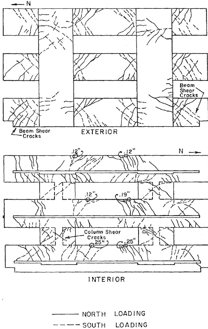
Fig. 3.11 Crack pattern after three cycles to 0.5% drift
