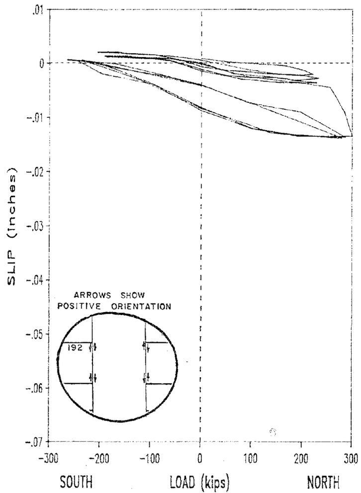
Fig. 4.12 Load vs. slip for LVDT 192.
