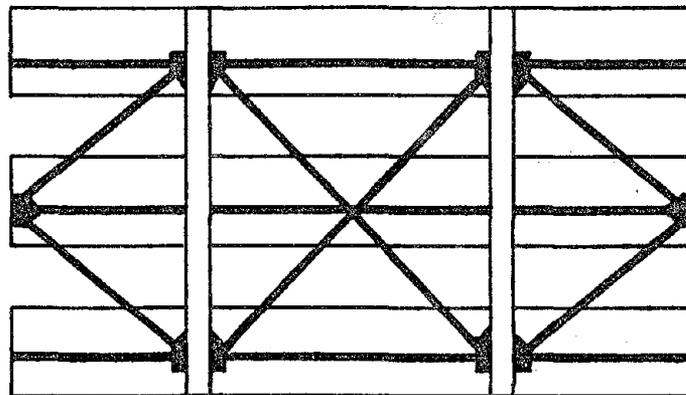
c. Steel bracing strengthened frame.
