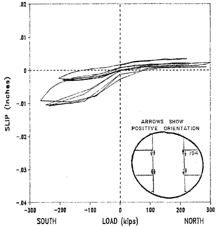
Fig. 4.15 Load vs. slip for LVDT 194
