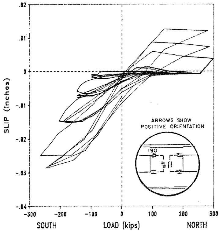
Fig. 4.10 Load vs. slip for LVDT 190
