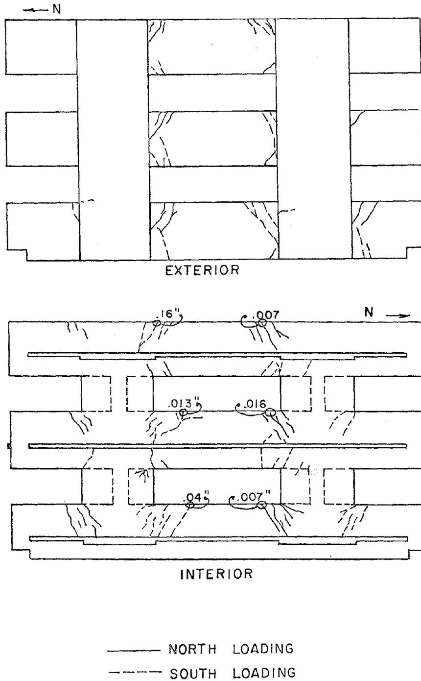
Fig. 3.5 Crack pattern after three cycles to 0.125% drift
