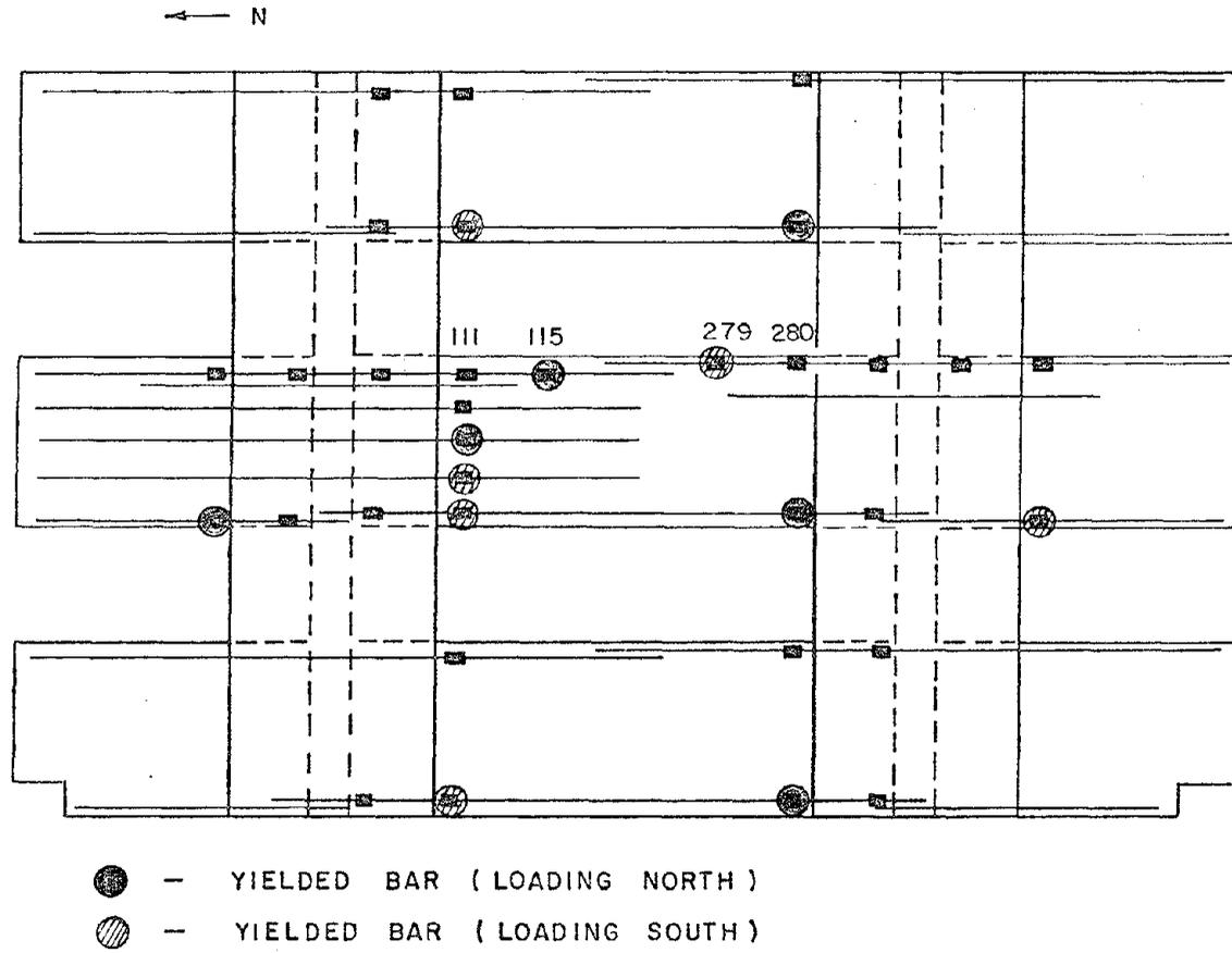
Fig. 3.9 Locations of yielded bars in beams indicated by strain gages after three cycles to 0.25% drift
