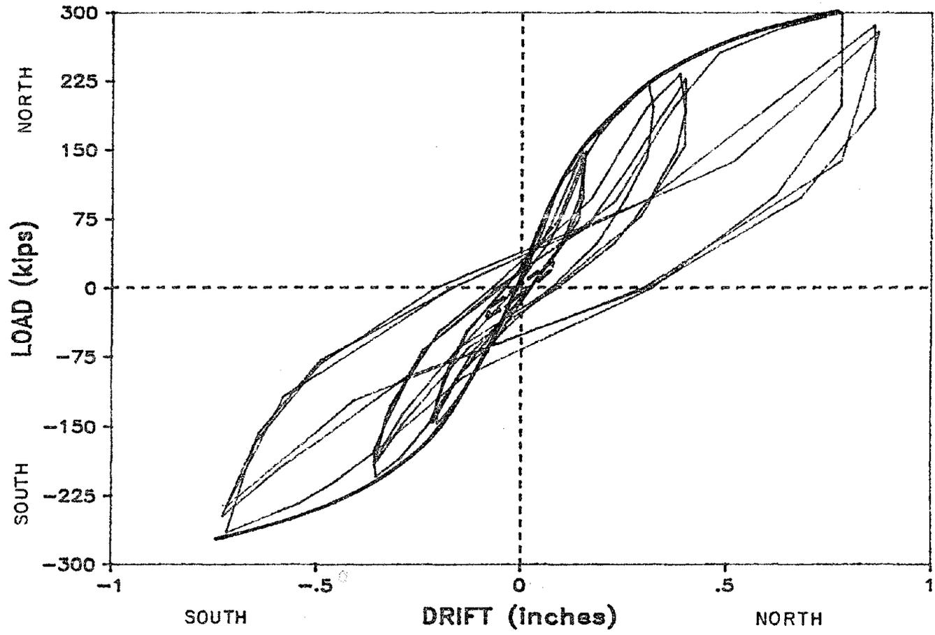
Fig. 3.17 Envelope of Load vs. drift plots for all cycles strengthened frame test
