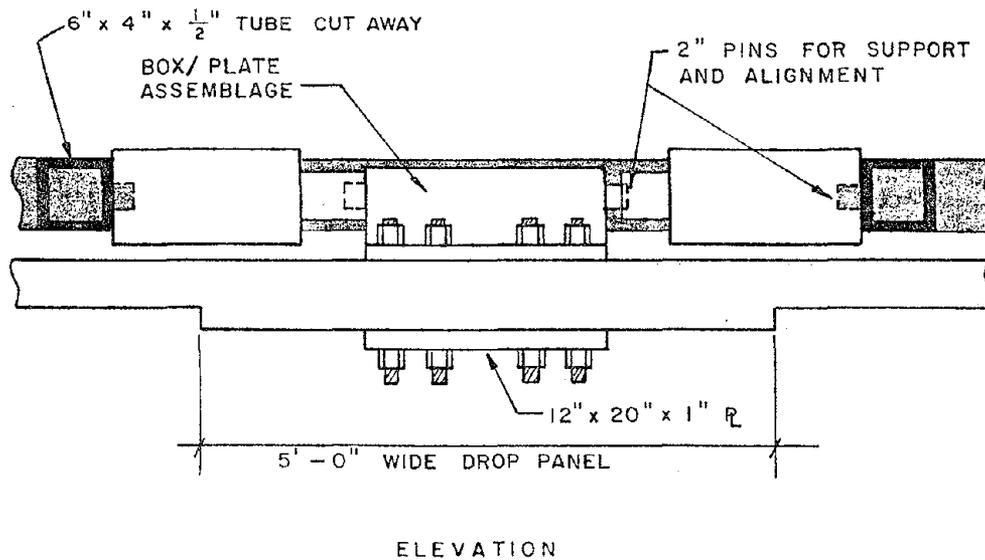
Fig. 2.40 Loading frame, hydraulic rams and box/plate assemblage at loading point
