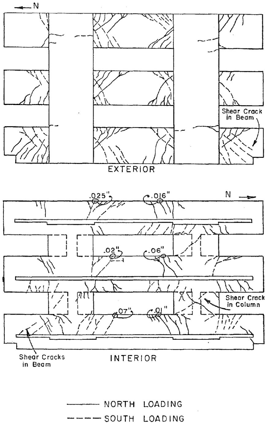
Fig. 3.8 Crack pattern after three cycles to 0.25% drift
