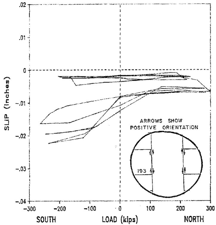
Fig. 4.14 Load vs. slip for LVDT 193
