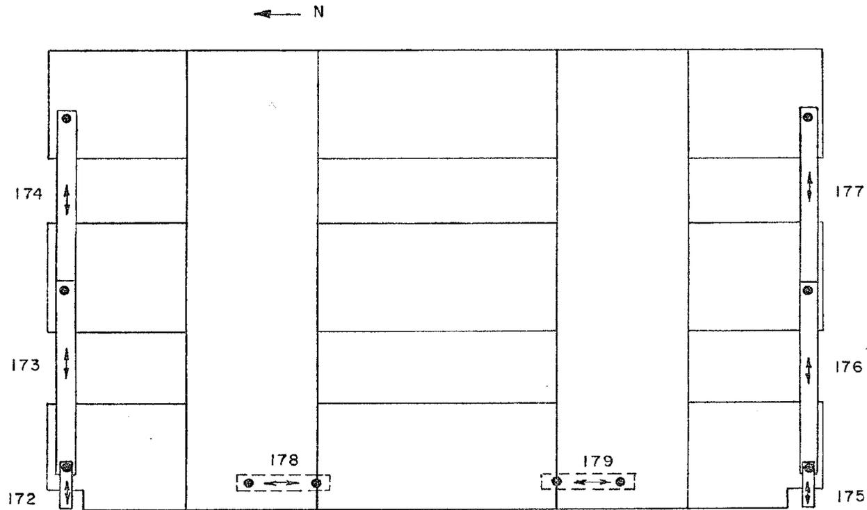
Fig. 2.52 Locations of load cells in the boundary restraints
