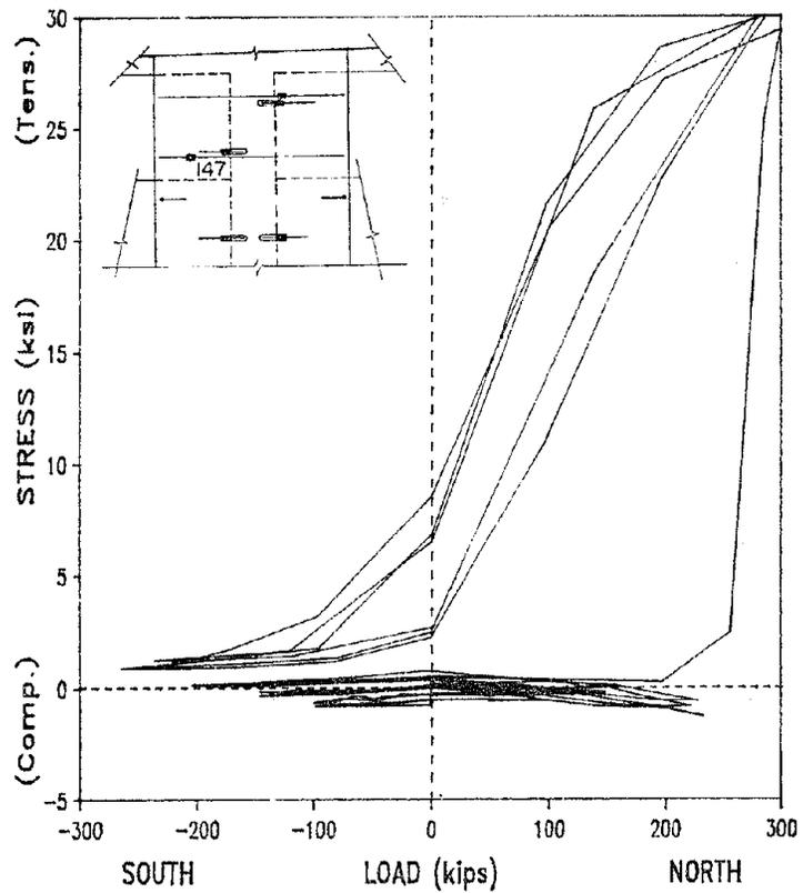
Fig. 4.25 Load vs. stress for stirrup gage 147
