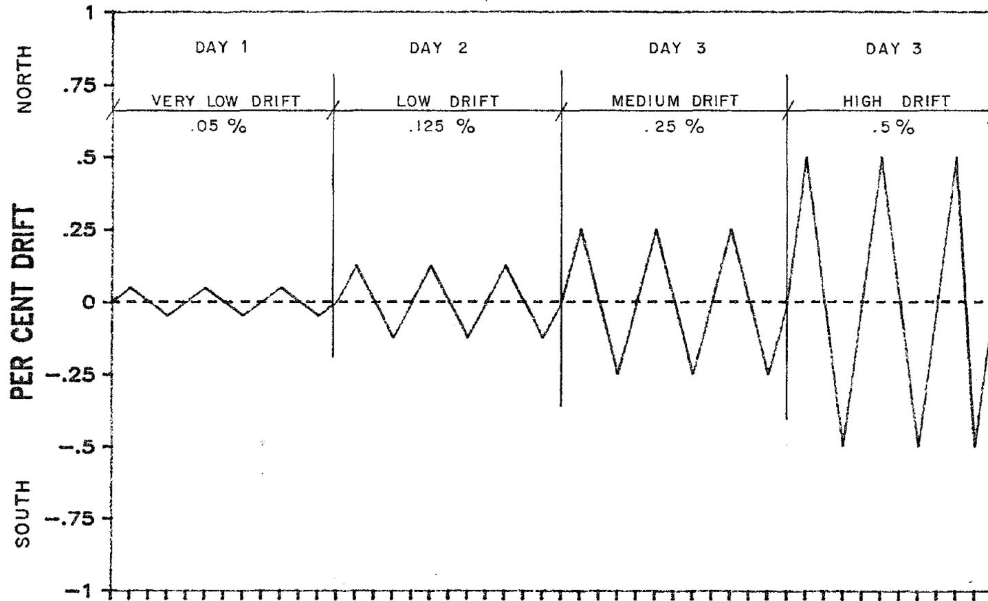
Fig. 3.2 Deformation history of the strengthened frame model
