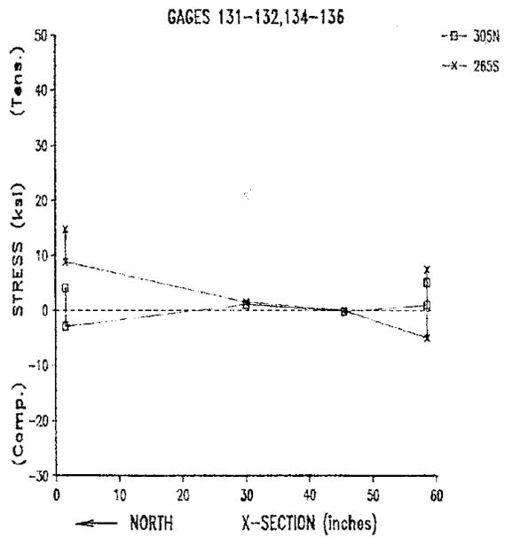
Fig. 4.6 Stress gradients across top and bottom cross sections of north pier, second level
