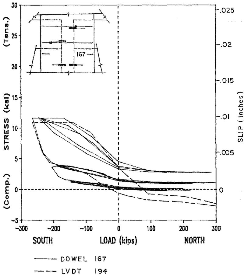
Fig. 4.19 Load vs. stress for dowel 167 and load vs. slip for LVDT 194
