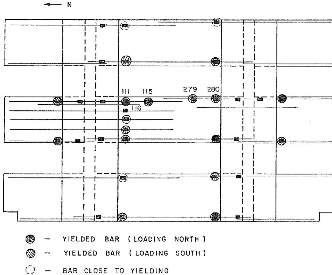
Fig. 3.16 Locations of yielded bars in beams indicated by strain gages after three cycles to 0.5% drift
