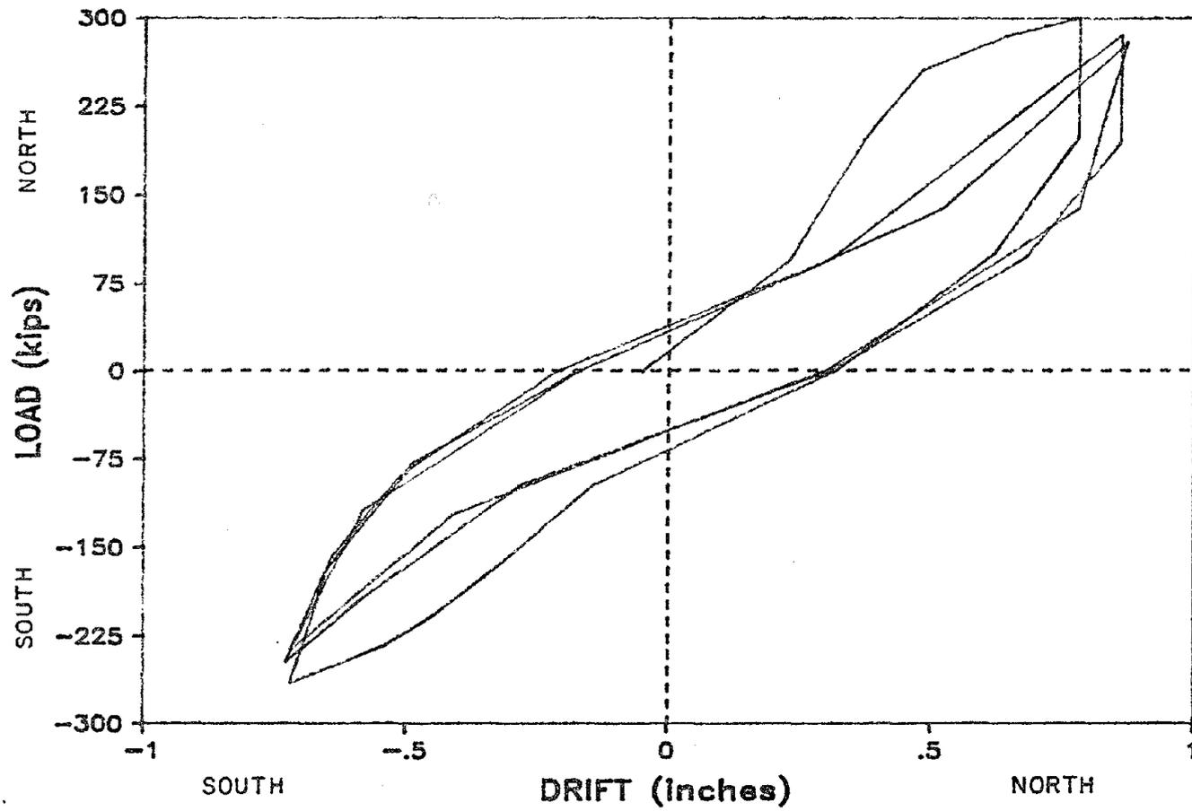
Fig. 3.10 Load vs. drift for three cycles to high (0.5%) drift
