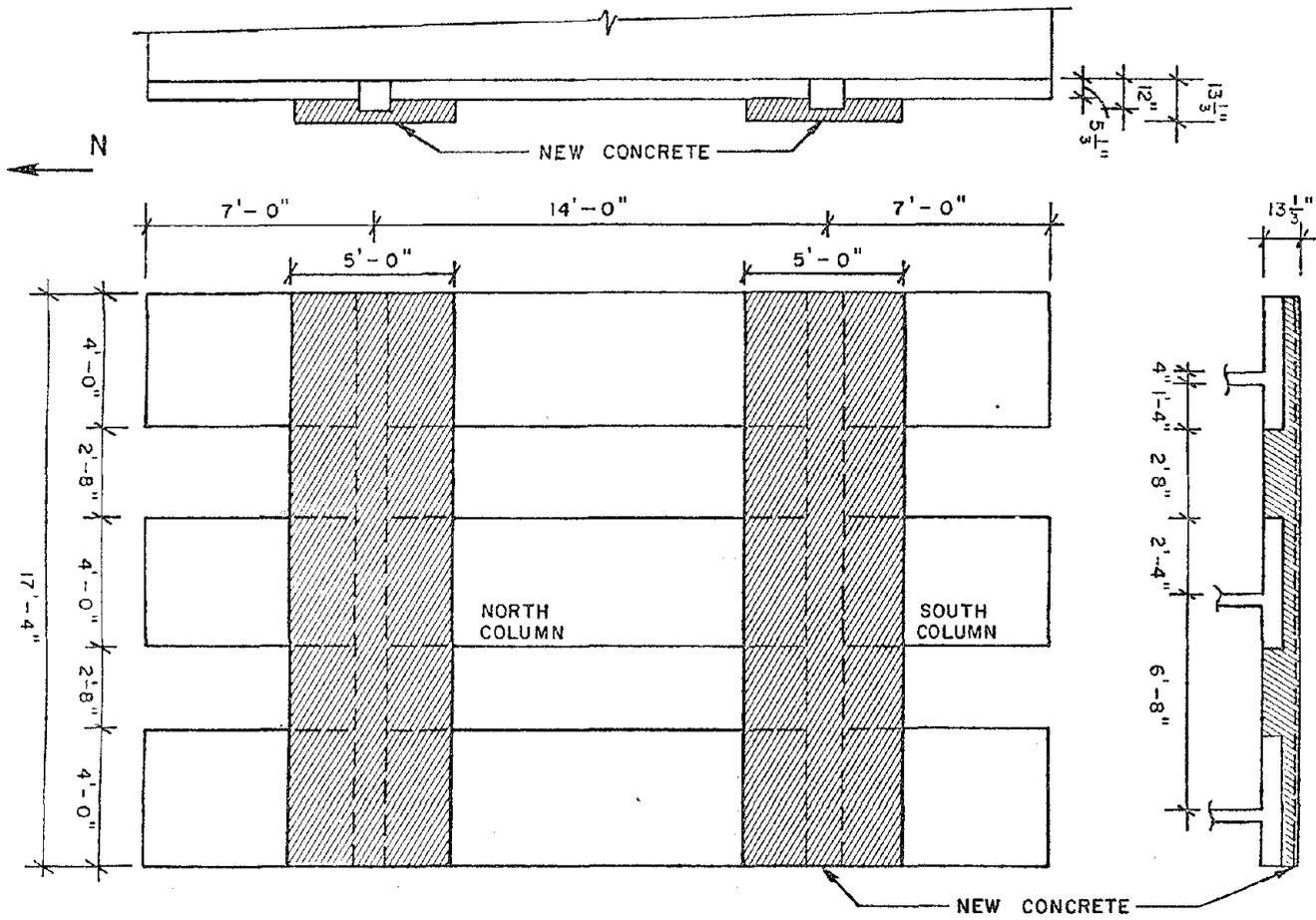
Fig. 2.21 Model retrofitted with R/C piers
