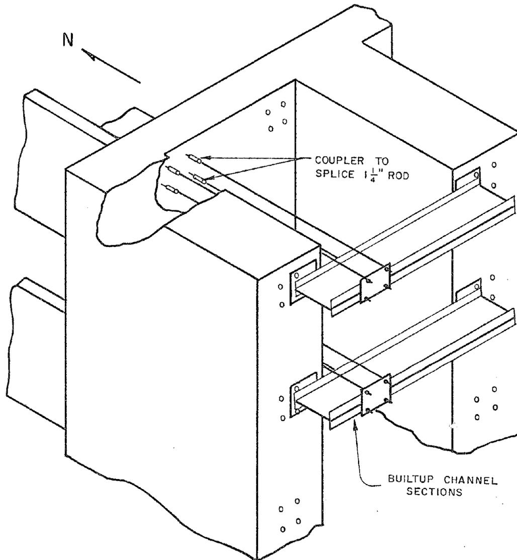
Fig. 2.37 Connection of loading frame to buttresses of reaction wall
