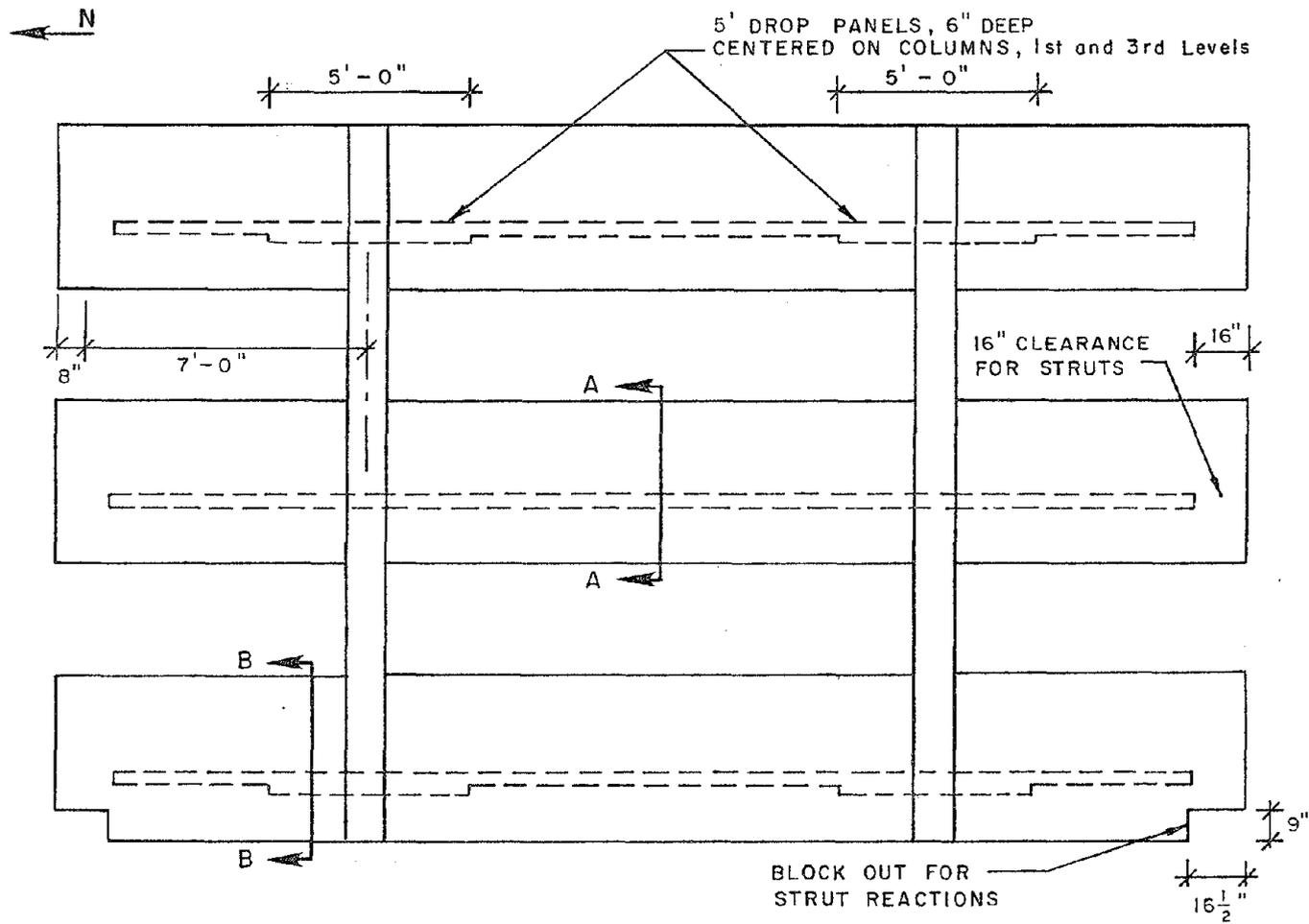
Fig. 2.12 Final design of test specimen.
