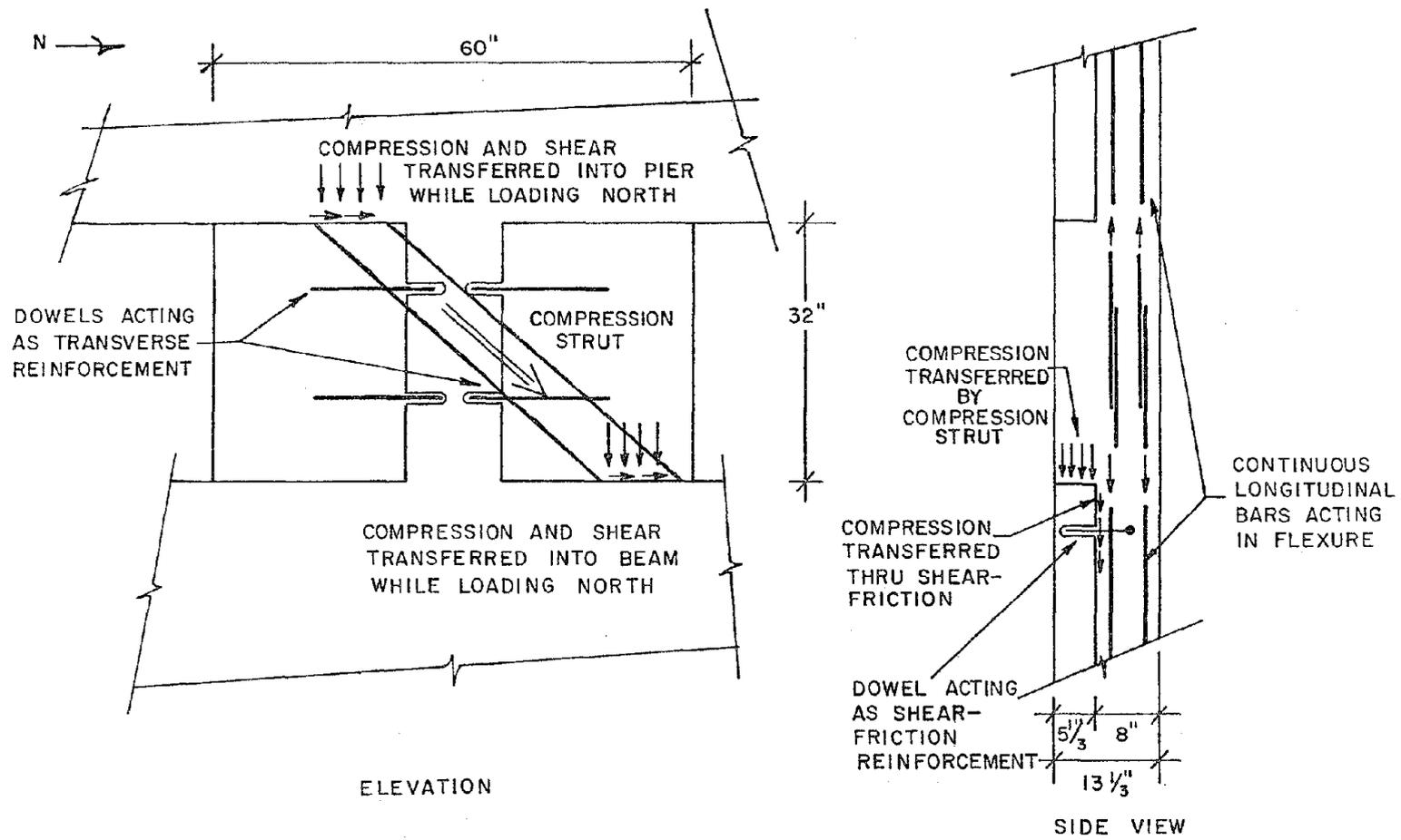
Fig. 4.4 Assumed behavior pattern of window segment under north loading conditions.
