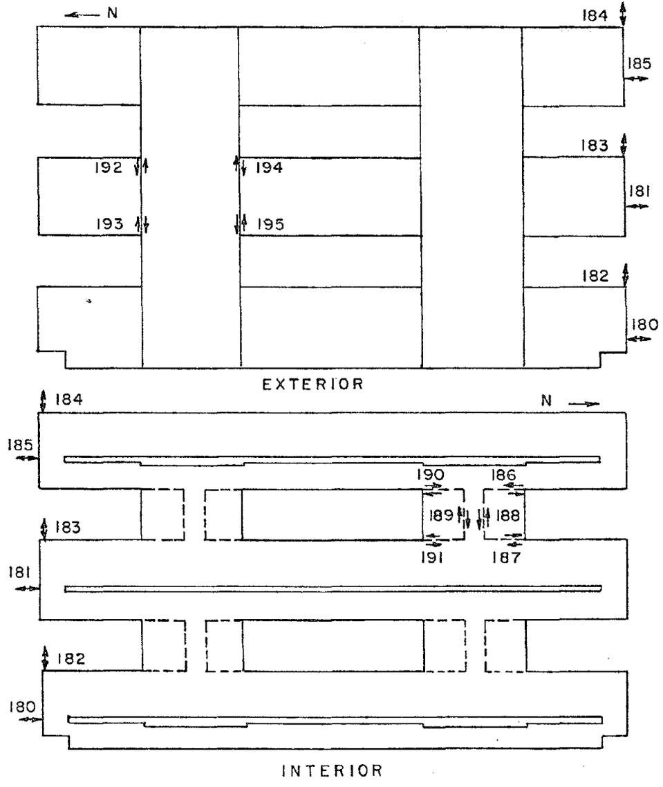
Fig. 2.53 Orientation and Location of LVDTs
