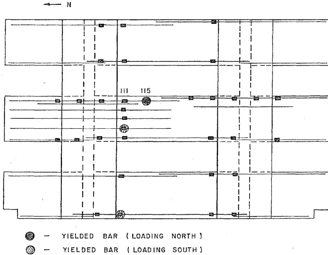
Fig. 3.6 Locations of yielded bars in beams indicated by strain gages after three cycles to 0.125% drift
