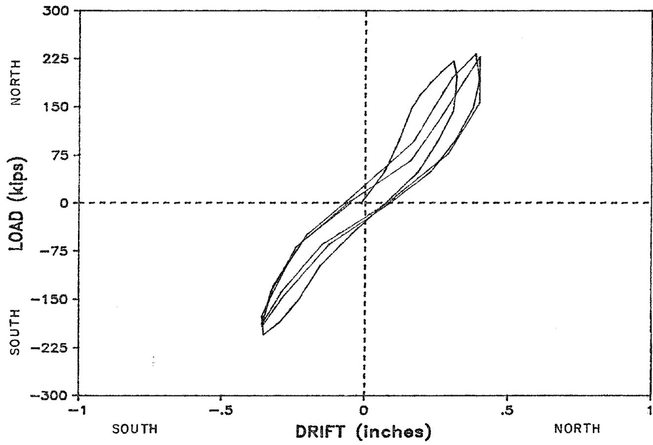
Fig. 3.7 Load vs. drift for three cycles to medium (0.25%) drift
