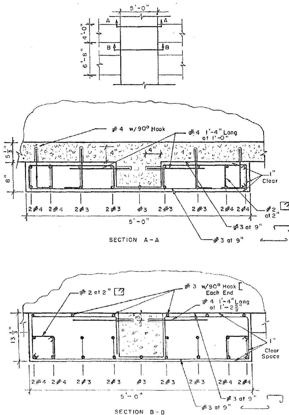
Fig. 2.22 Details of 2/3 scale model of R/C pier
