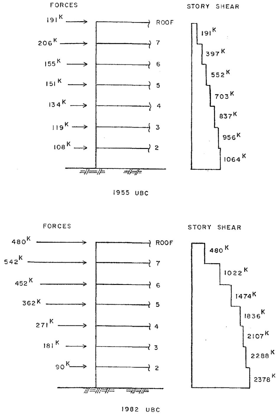
Fig. 2.3 Design loads for prototype building based on UBC earthquake regulations
