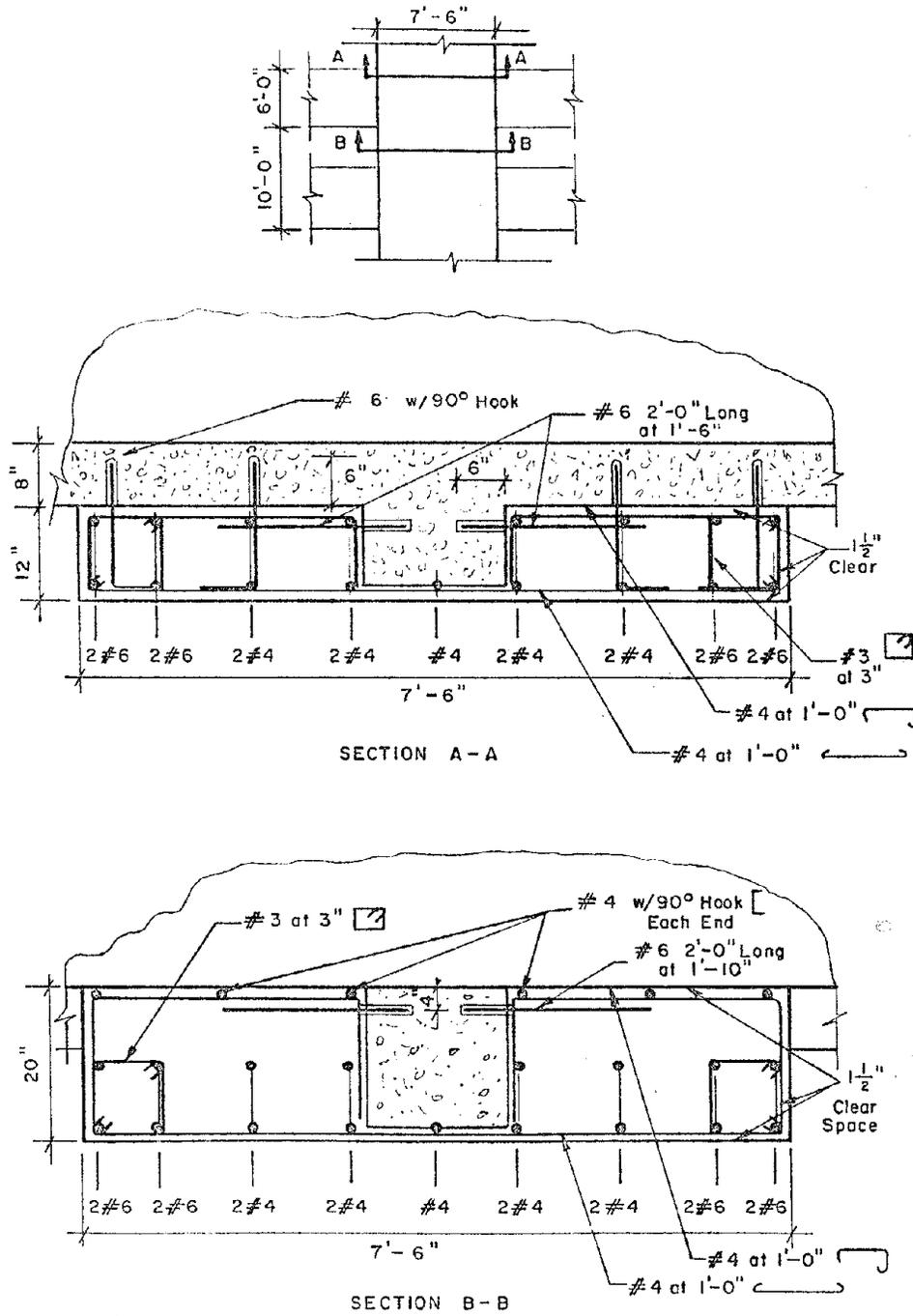
Fig. 2.5 Details of reinforced concrete pier
