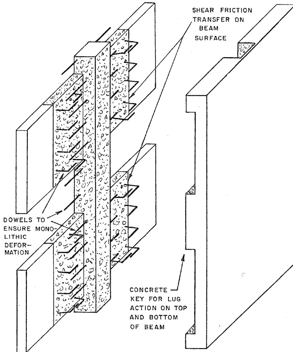
Fig. 2.7 Load transfer actions in pier strengthening
