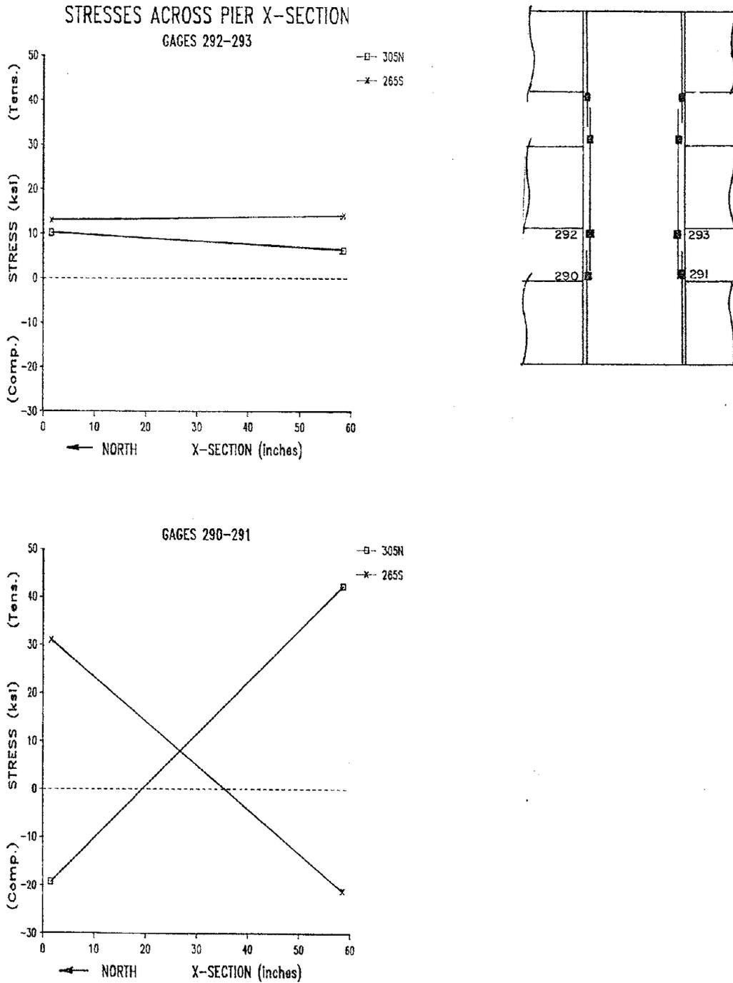
Fig. 4.7 Stress gradients across top and bottom cross sections of south column, first level
