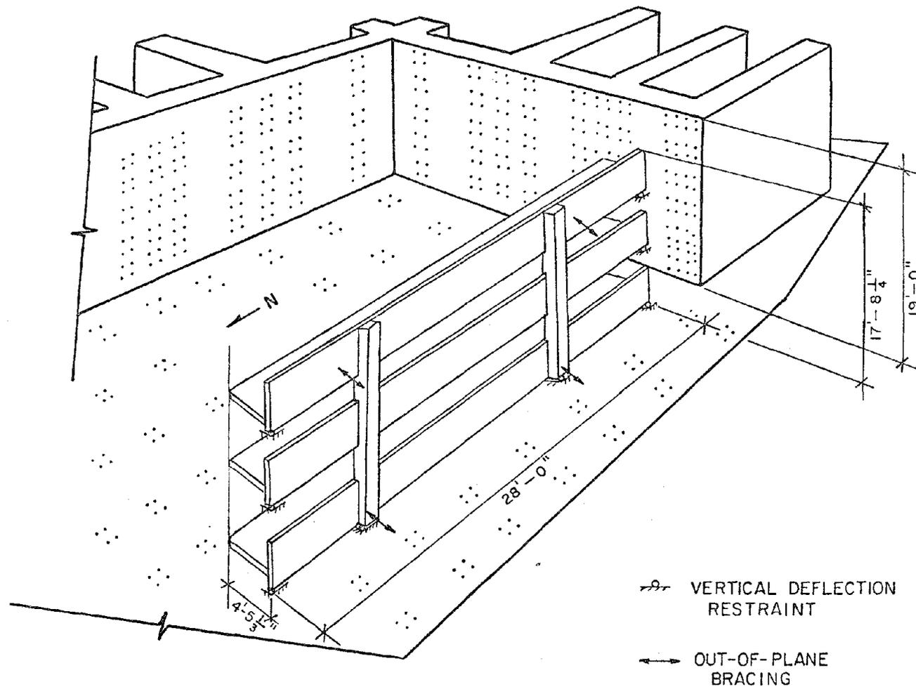
Fig. 2.14 Frame location on floor wall reaction system
