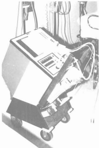
Figure 5.6 Portable EKG machine. Wheel locks are not provided on this example.
