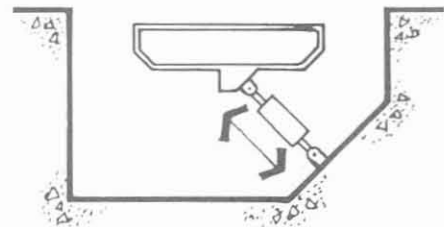
Figure 4.1b Vector biaxial-single direction of input motion at an angle to the test table.
