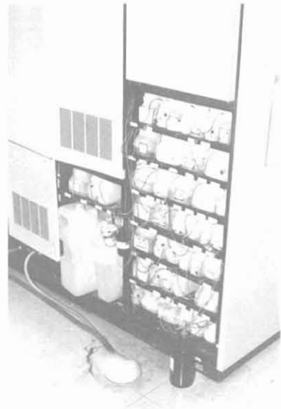
Figure 5.33 Detail of analyzer shown in Figure 5.31. Note the glass and plastic tubes that are susceptible to pulling out or breaking in an earthquake.
