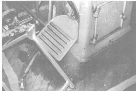
Figure 2.2 — Lathe in a school showing vertical displacement that occurred during the Coalinga earthquake. Note the shavings under the previous location of the base that were not disturbed when that part of this heavy equipment item was displaced in the earthquake.
