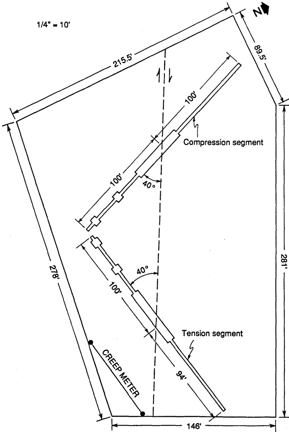
Figure 3-5. Trenches for Welded Steel Segments
