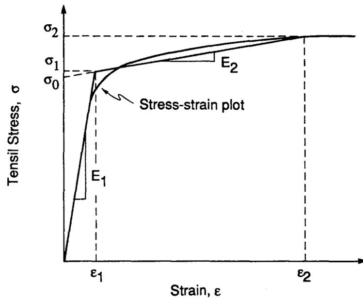
**Figure 2-2. Steel Stress-Strain Relation Assumed in Newmark-Hall Design Approach**
