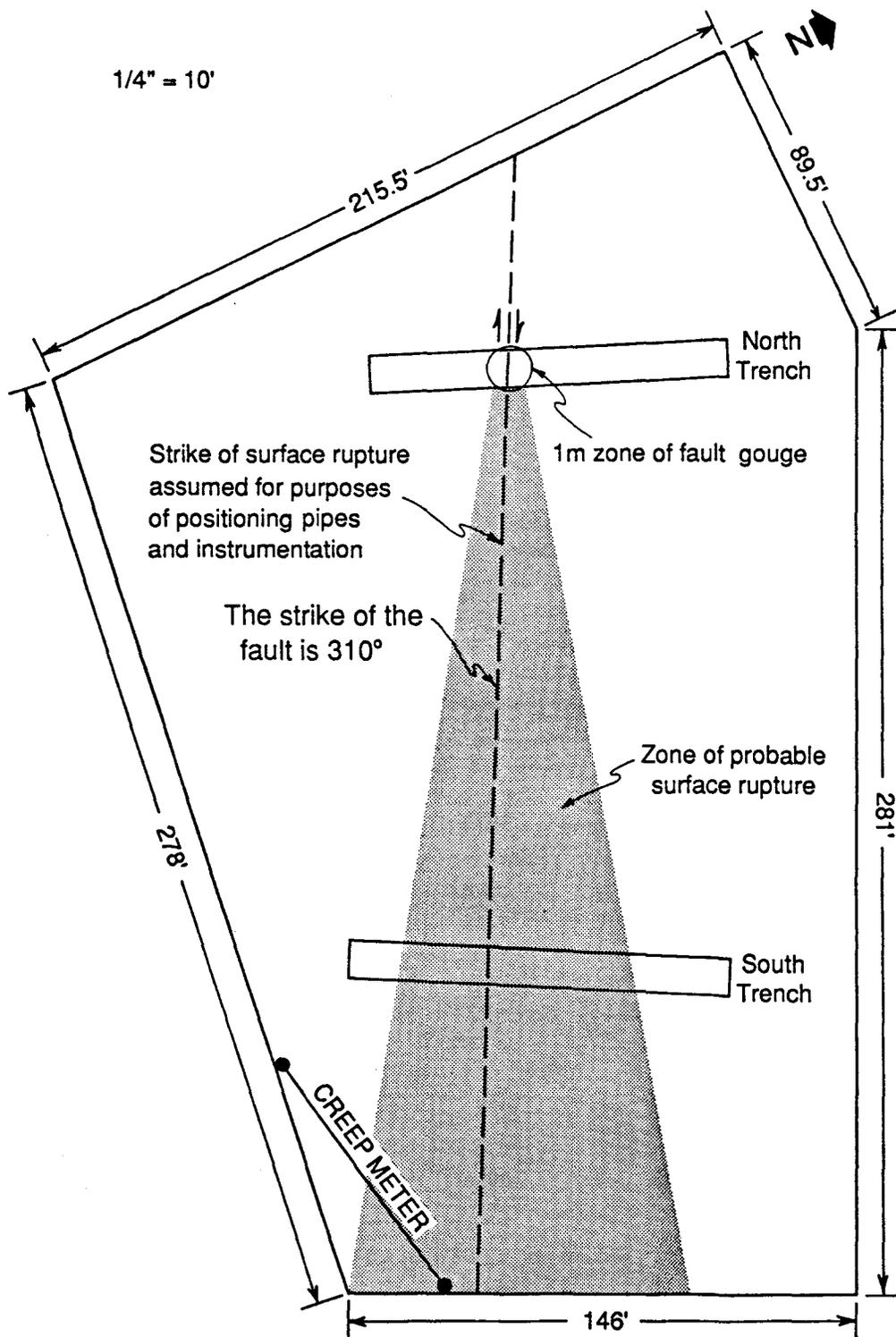
Figure 3-2. Assumed Zone of Surface Rupture, Owens Pasture
