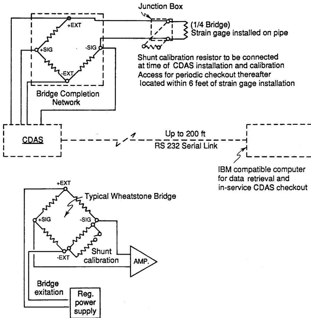
**Figure A-1. Wheatstone Bridge Used to Measure Strains on Welded Steel Pipe**
