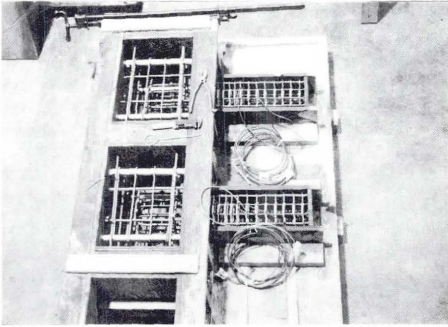
FIG. 2.2 Test Specimens Ready for Casting
