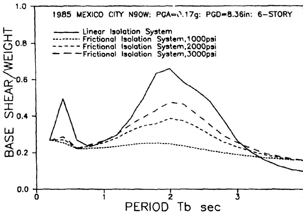
**FIGURE 7-7 Spectra of Basemat Displacement and Base Shear of 6-Story Isolated Structure Subjected to Mexico City Earthquake**
