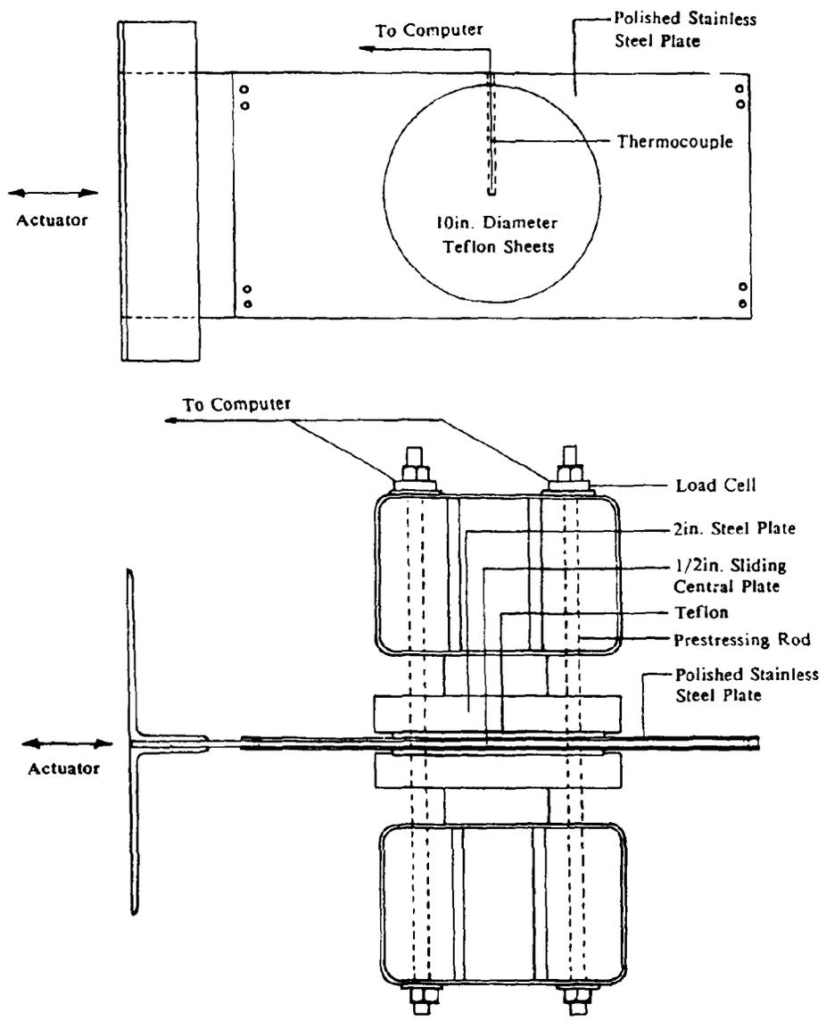
**FIGURE 4-1 Testing Arrangement**
