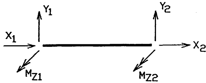
Figure 2.19 - Unrestrained Longitudinal Deck DOF's
