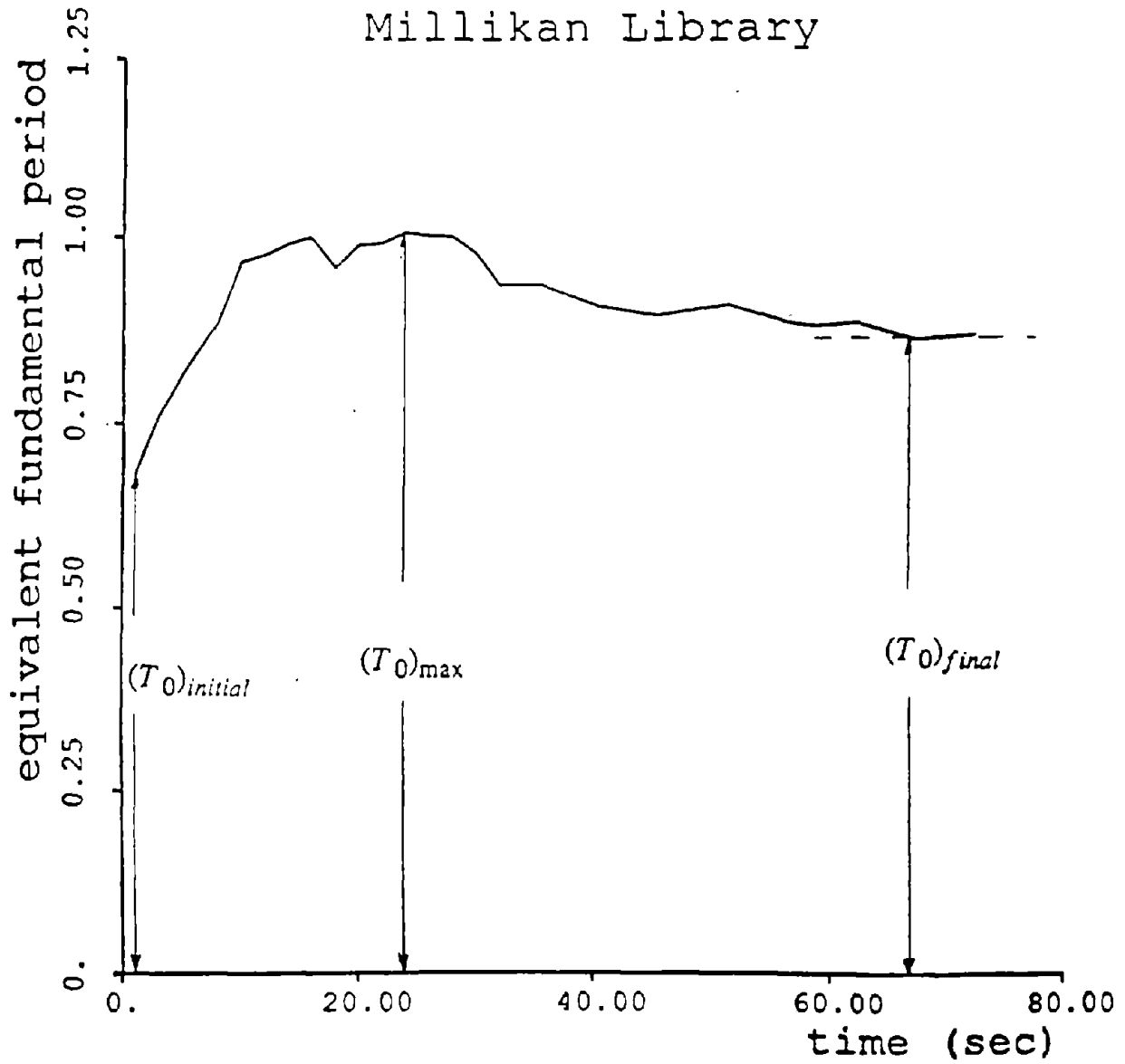
Figure 1.1: Evolution of the Equivalent Fundamental Period for the Millikan Library
