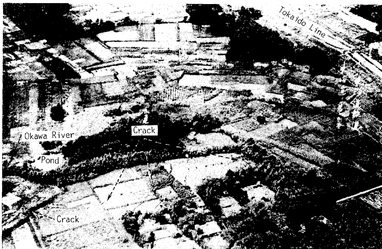
Fig.3 Aerial photo of Nakajima Area taken shortly after the earthquake showing ground cracks (Association for the Development of National Education, 1923)
