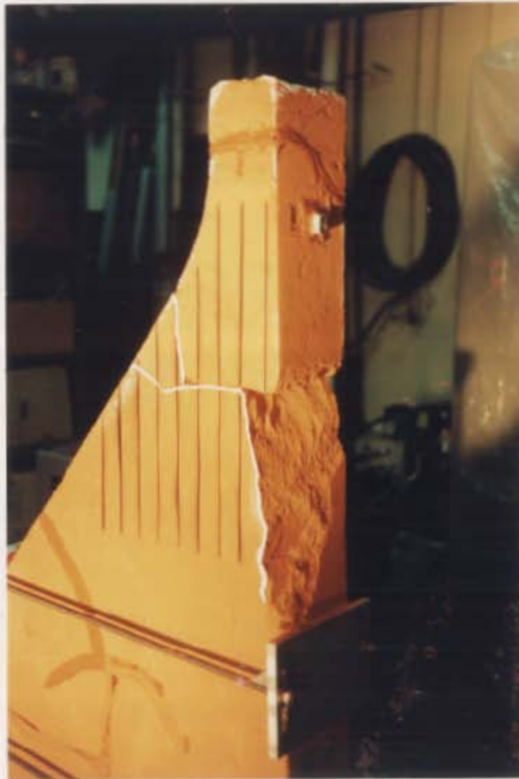
Figure 4.15: (a) Filmed side of monolithic model after second earthquake test.
