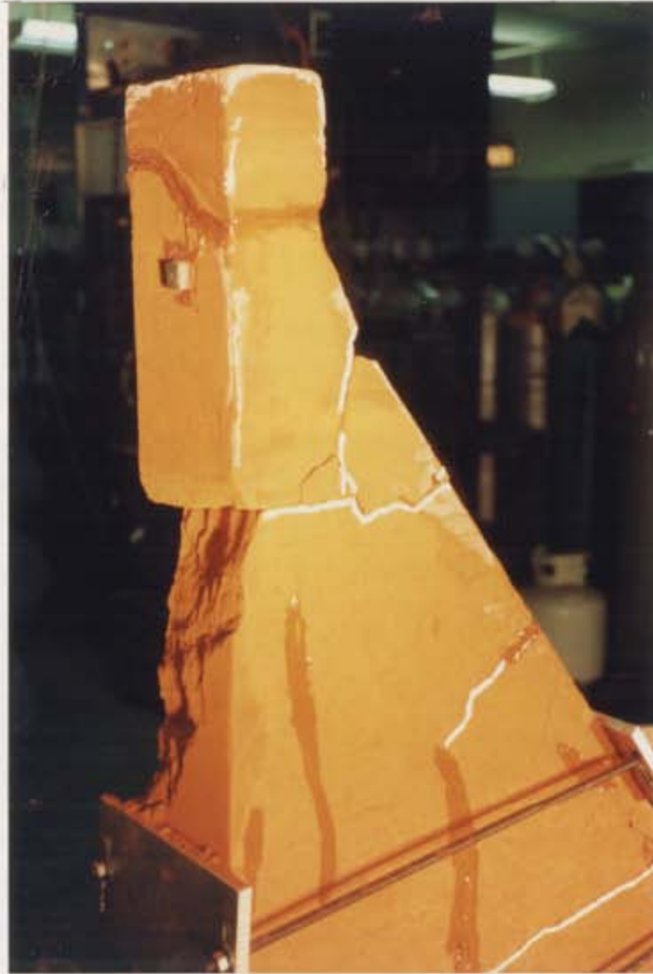
Figure 4.15: (b) Opposite side of monolithic model after second earthquake test.
