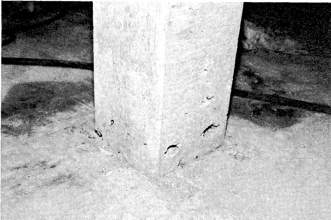
**Fig. 3.8 Honeycombs in Column of Specimen 3**
