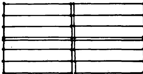
FIG. E06.5 SEVERAL ELEMENTS PER PANEL IMPROVES COMPATIBILITY AT VERTICAL EDGES
