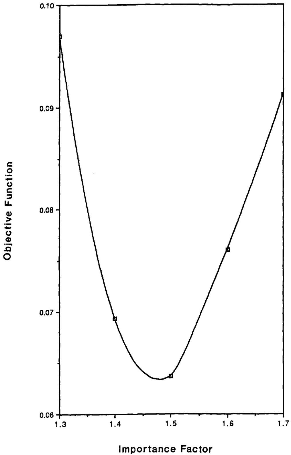
**FIGURE 9-10** Determination of Importance Factor for Essential Buildings ( $E_D = 0.3$  g,  $P_{F_C,T} = 1/5000$  per year)
