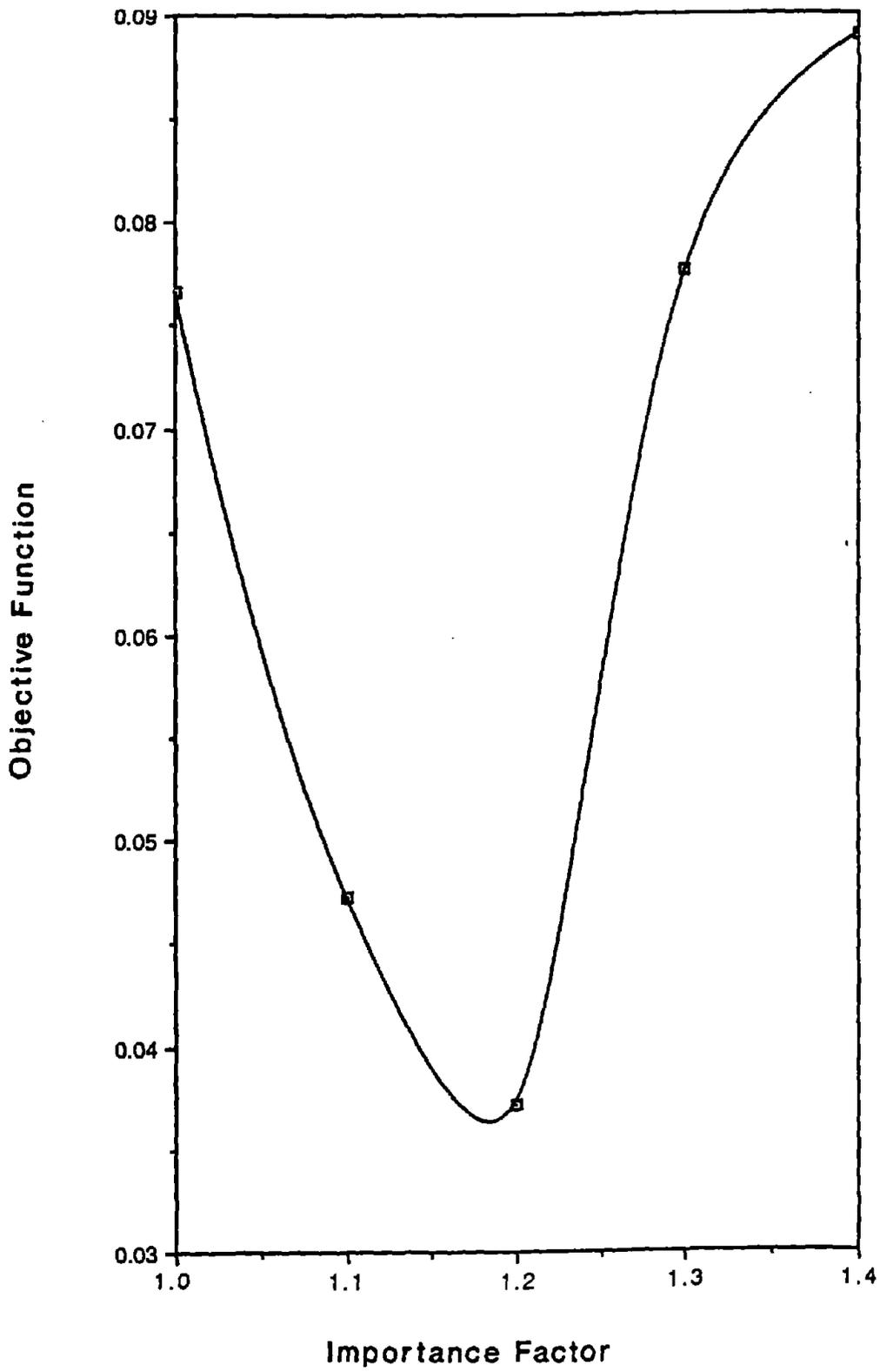
**FIGURE 9-7** Determination of Importance Factor for High-risk Buildings ( $E_D = 0.3 g$ )
