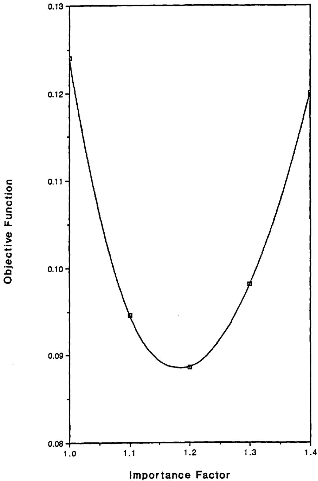
**FIGURE 9-6** Determination of Importance Factor for High-risk Buildings ( $E_D = 0.4$  g)
