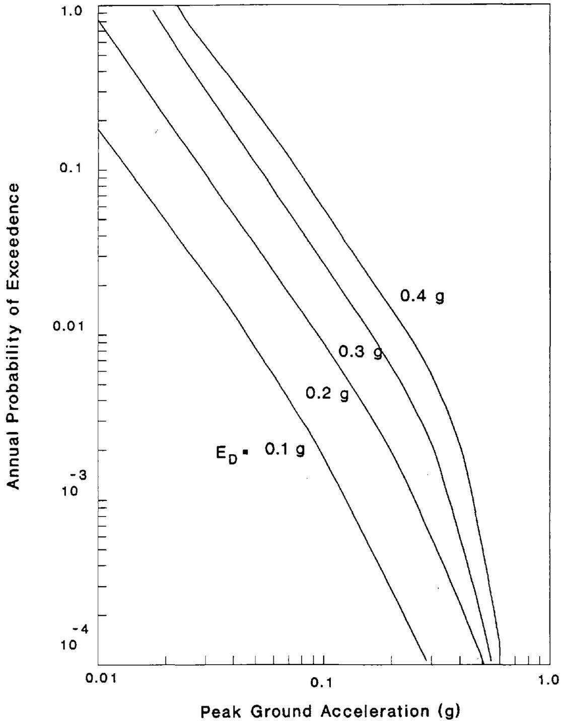
**FIGURE 2-1 Seismic Hazard Curves (NEHRP Recommended Provisions 1988)**
