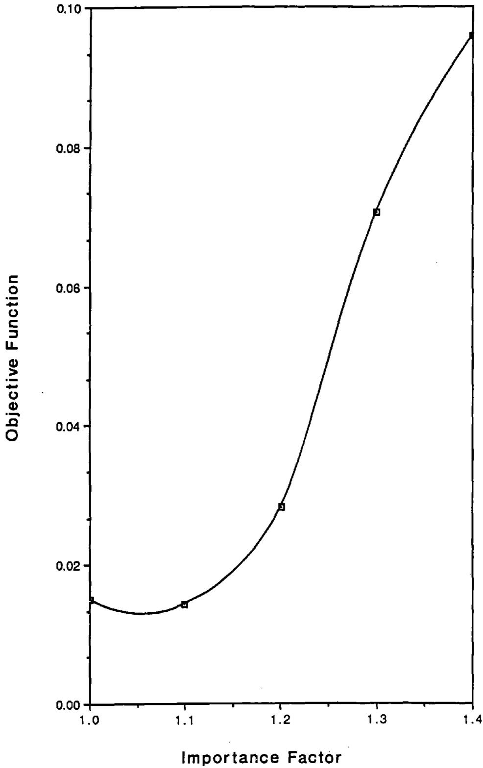
**FIGURE 9-8** Determination of Importance Factor for High-risk Buildings ( $E_D = 0.2$  g)
