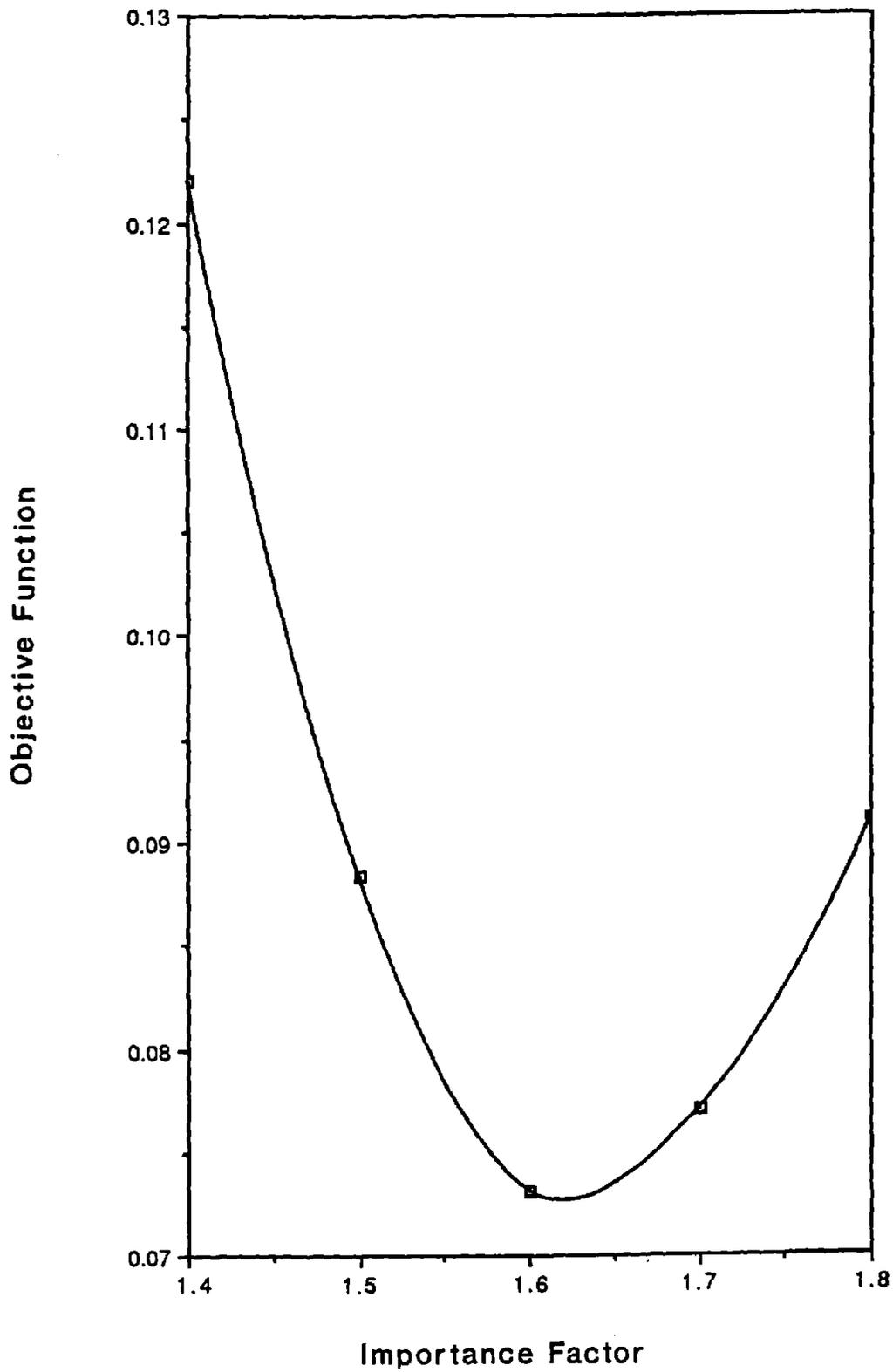
**FIGURE 9-9** Determination of Importance Factor for Essential Buildings ( $E_D = 0.4$  g,  $P_{F_{C,T}} = 1/5000$  per year)
