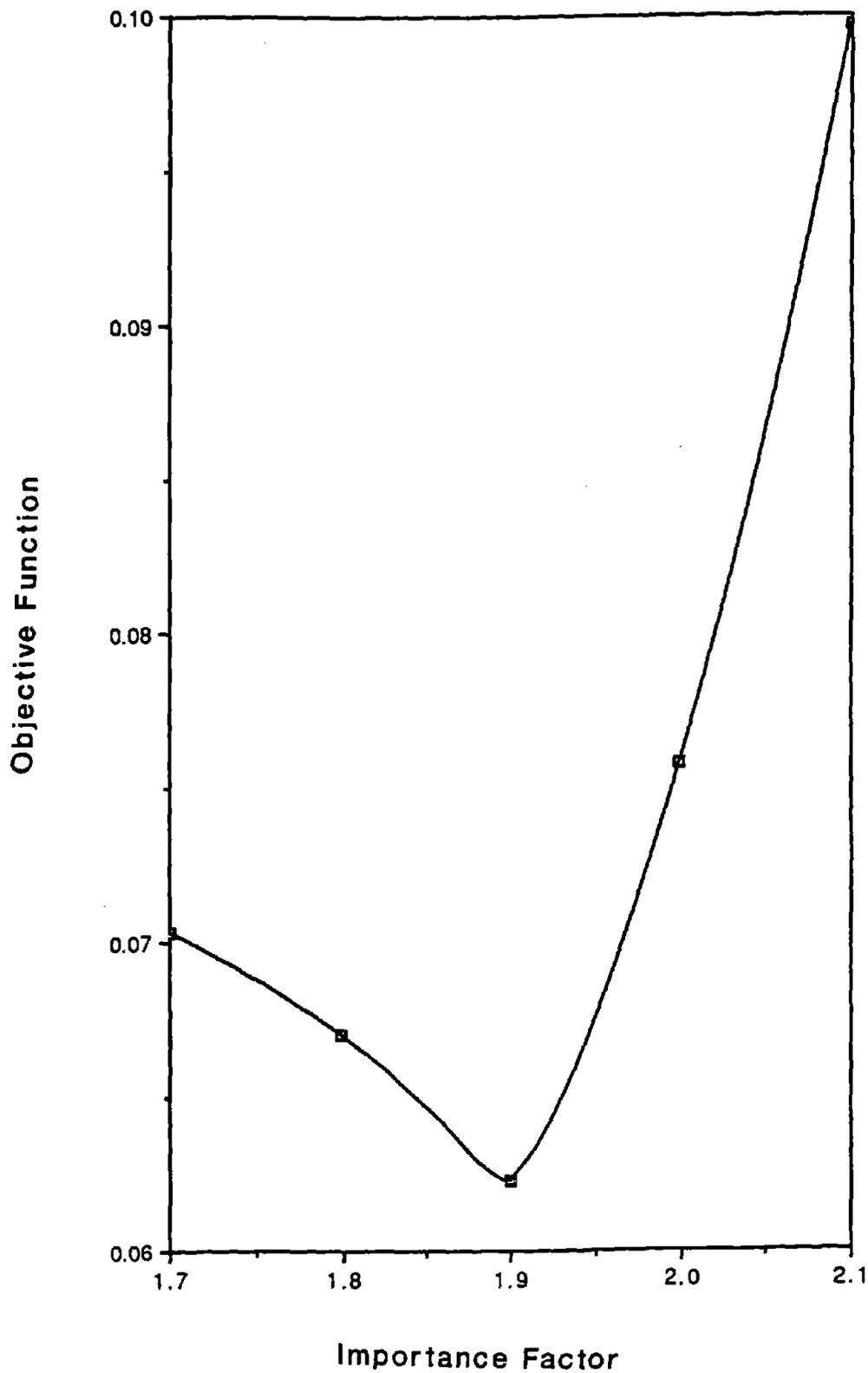
**FIGURE 9-13** Determination of Importance Factor for Essential Buildings ( $E_D = 0.3$  g,  $P_{F_C,T} = 1/10,000$  per year)
