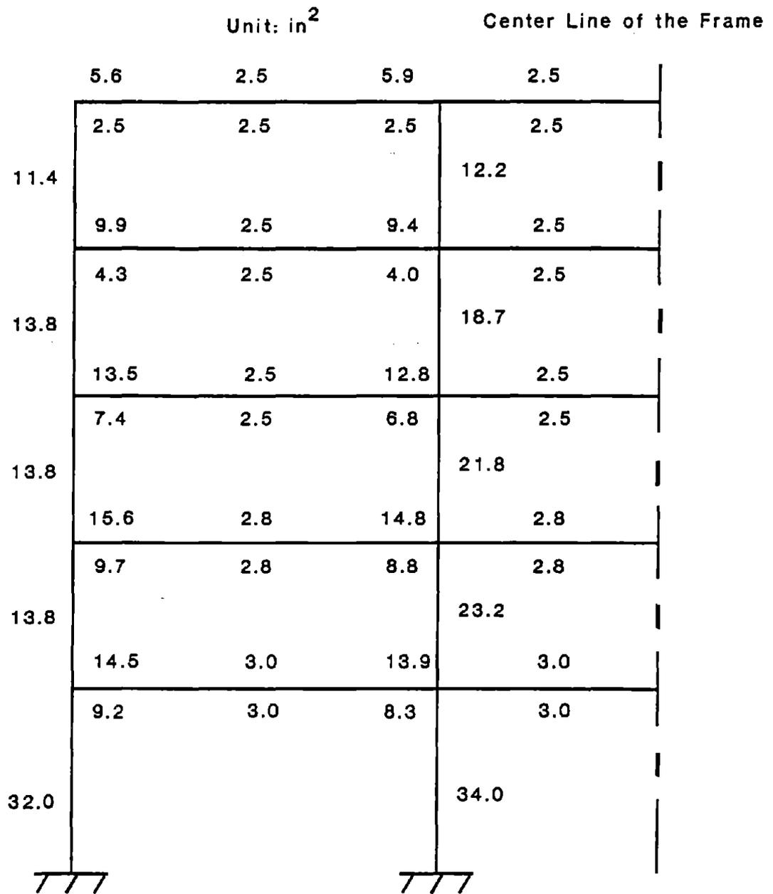
**FIGURE 5-6 Required Steel Areas of the Illustrative Frame**
