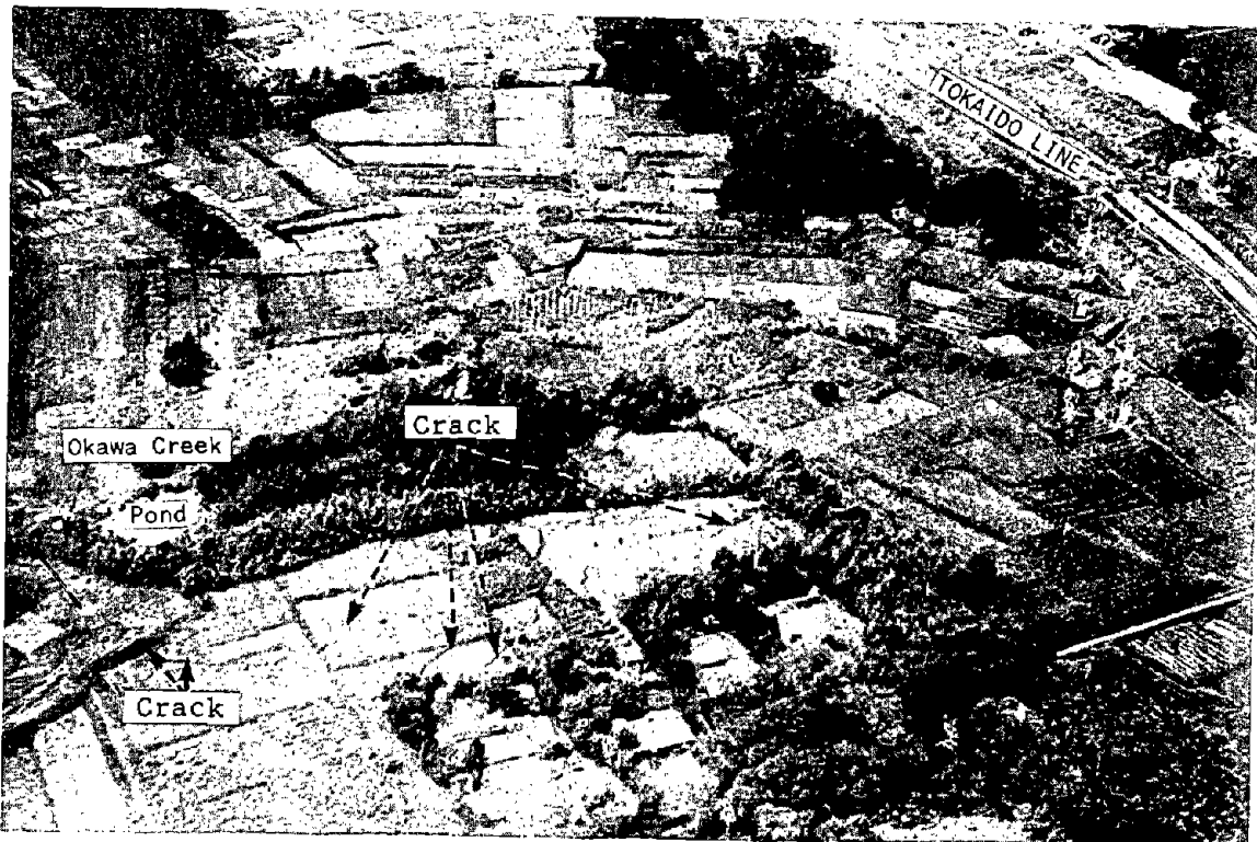
Figure 7 Aerial Photograph of Nakajima Area Showing Ground Cracks Caused by the Kanto Earthquake (Looking Southeast) (Association for the Development of National Education, 1926) 15)
