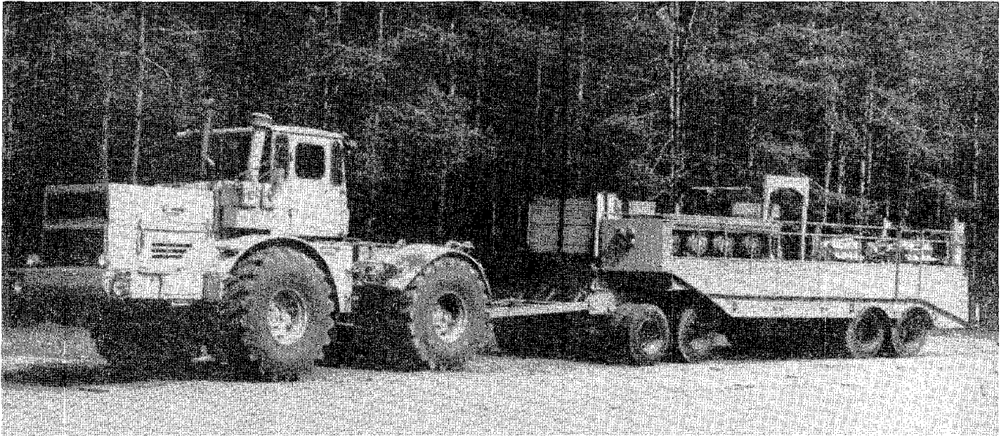
Figure 12. 30-ton seismic vibrator with 8-ton inertial mass used in Russia for generation of seismic waves for study of nonlinear soil properties on attenuation of waves.
