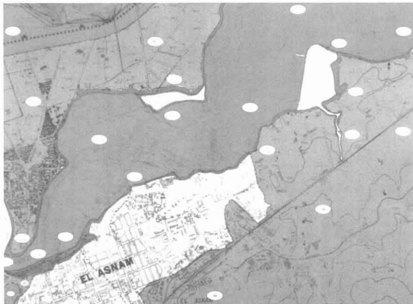
Figure 3.4.7. Seismic hazard map of El Asnam and vicinity showing three seismic hazard zones. The darkest areas (I) are the most hazardous, the lightest areas (II) are moderately hazardous, and the medium tone areas are the safest. Subscripts in the ovals further identify the specific hazards present.
