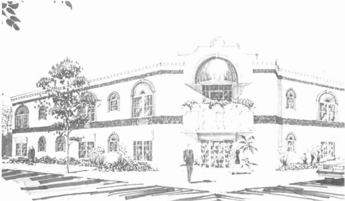
Figure 4.2.5. Sketch of a planned stucco building with brick trim – a proposed compromise.
