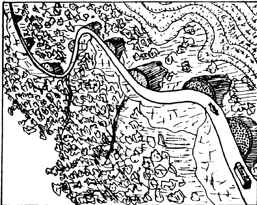
Fig. 1 Schematic representation of organised dumping of hill road construction debris
