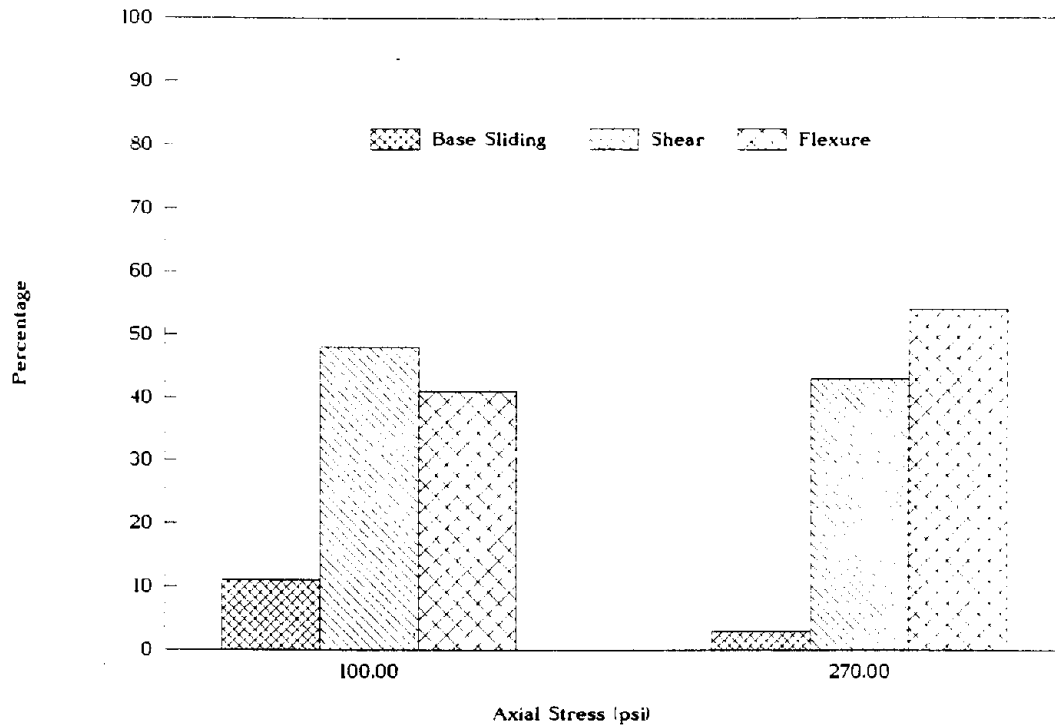
Figure 6.6 - Contribution of Different Deformation Mechanisms at about One-Inch Total Displacement (No. 6 Vertical and No. 4 Horizontal Bars)
