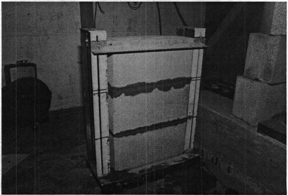
Figure 4.1 - Construction of Masonry Prism
