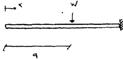
$$\gamma(x) = -\frac{w}{6EI} ((x-b)^3 - 3a^2(x-b) + 2a^3) \quad \text{where } b = L - x$$
