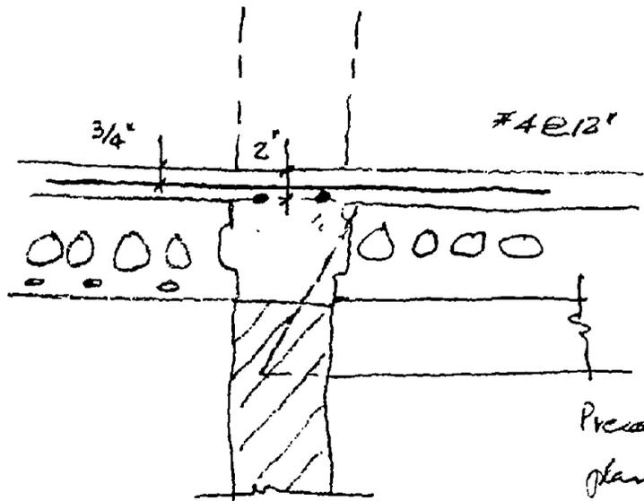
Precast beam to support plank over corridor
