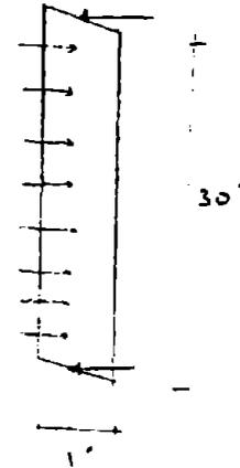
$$\text{Vertical Load @ Mid-height} = \left(1 \times \frac{30}{2} \times 77\right) + (1 \times 4 \times 15)$$
