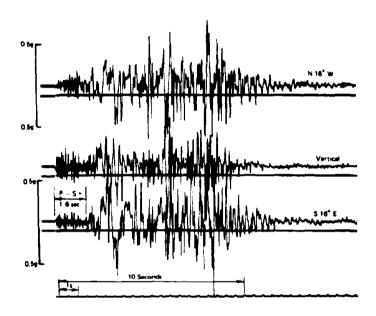
FIGURE 1 This accelerogram was recorded above the causative fault at the center of energy release during the 1971 magnitude 6.5 San Fernando earthquake. This very intense ground shaking was recorded on the side of a steep hill. More than \$1 billion in damage (1987 dollars) was caused by this intermediate-sized earthquake.
