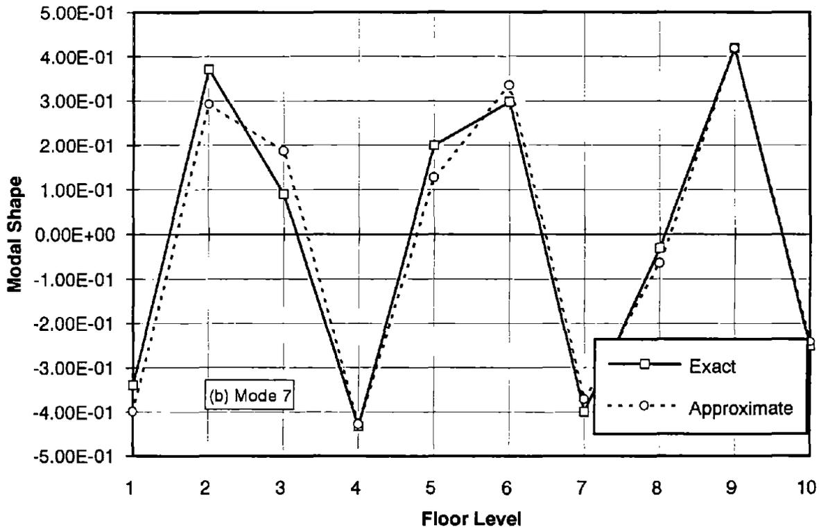
FIGURE 5.3: COMPARISON OF EXACT AND APPROXIMATE MODAL SHAPE FOR MODE 1 AND MODE 7. BUILDING NO. 1
