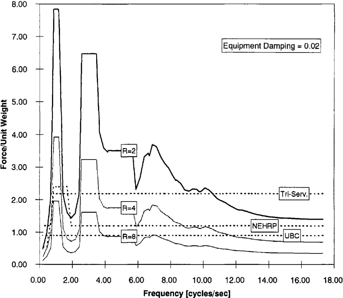
FIGURE 4.12: COMPARISON OF FLOOR 5 SPECTRA CALCULATED BY VARIOUS PROVISIONS AND THE PROPOSED RESPONSE SPECTRUM APPROACH. GENERAL EQUIPMENT - SOIL S1
