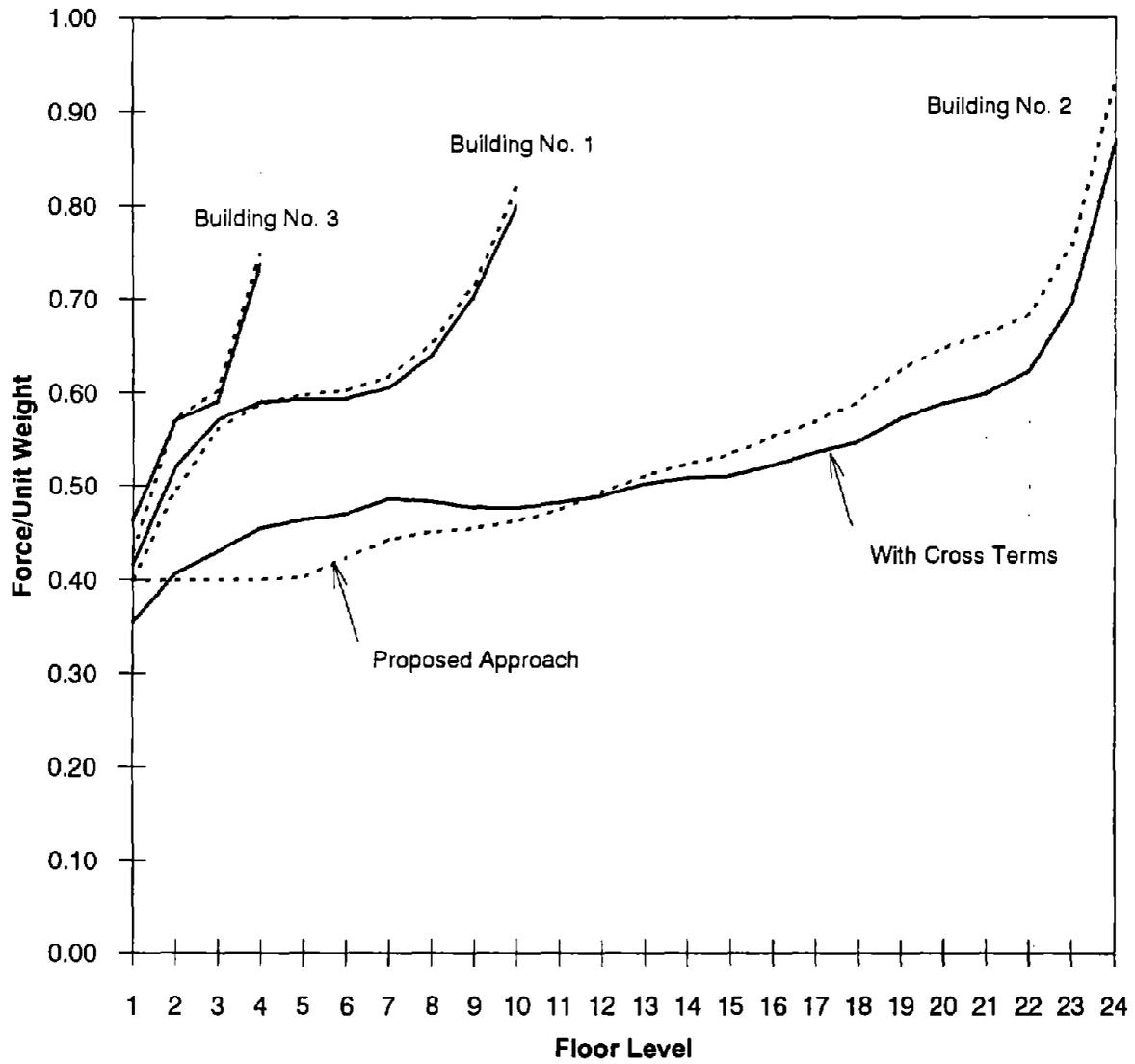
FIGURE A.3: COMPARISON OF FLOOR ACCELERATION CALCULATED WITH CROSS TERMS AND PROPOSED APPROACH FOR BUILDINGS 1,2 AND 3.
