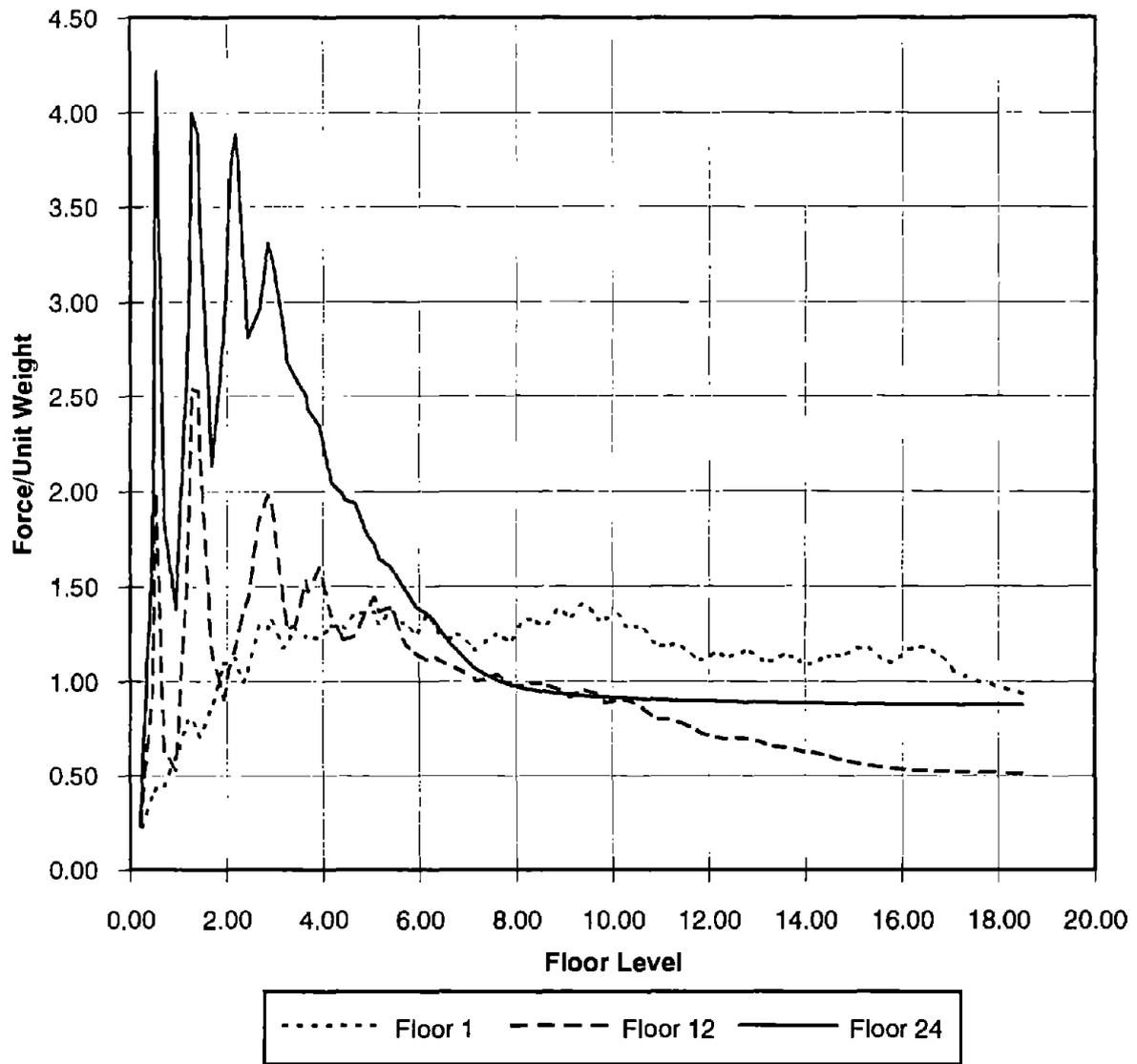
FIGURE 5.26: VARIATION OF FLOOR SPECTRA WITH FLOOR LEVEL.
