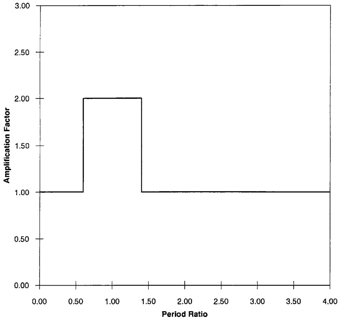
FIGURE 2.1: ATTACHMENT AMPLIFICATION FACTOR USED IN NEHRP PROVISIONS.
