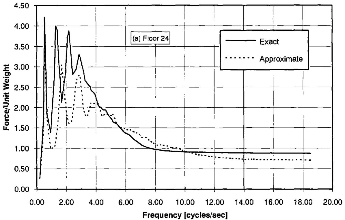
FIGURE 5.14: COMPARISON OF FLOOR SPECTRA FOR FLOORS 1 AND 24 CALCULATED WITH EXACT AND APPROXIMATE PROPERTIES.
