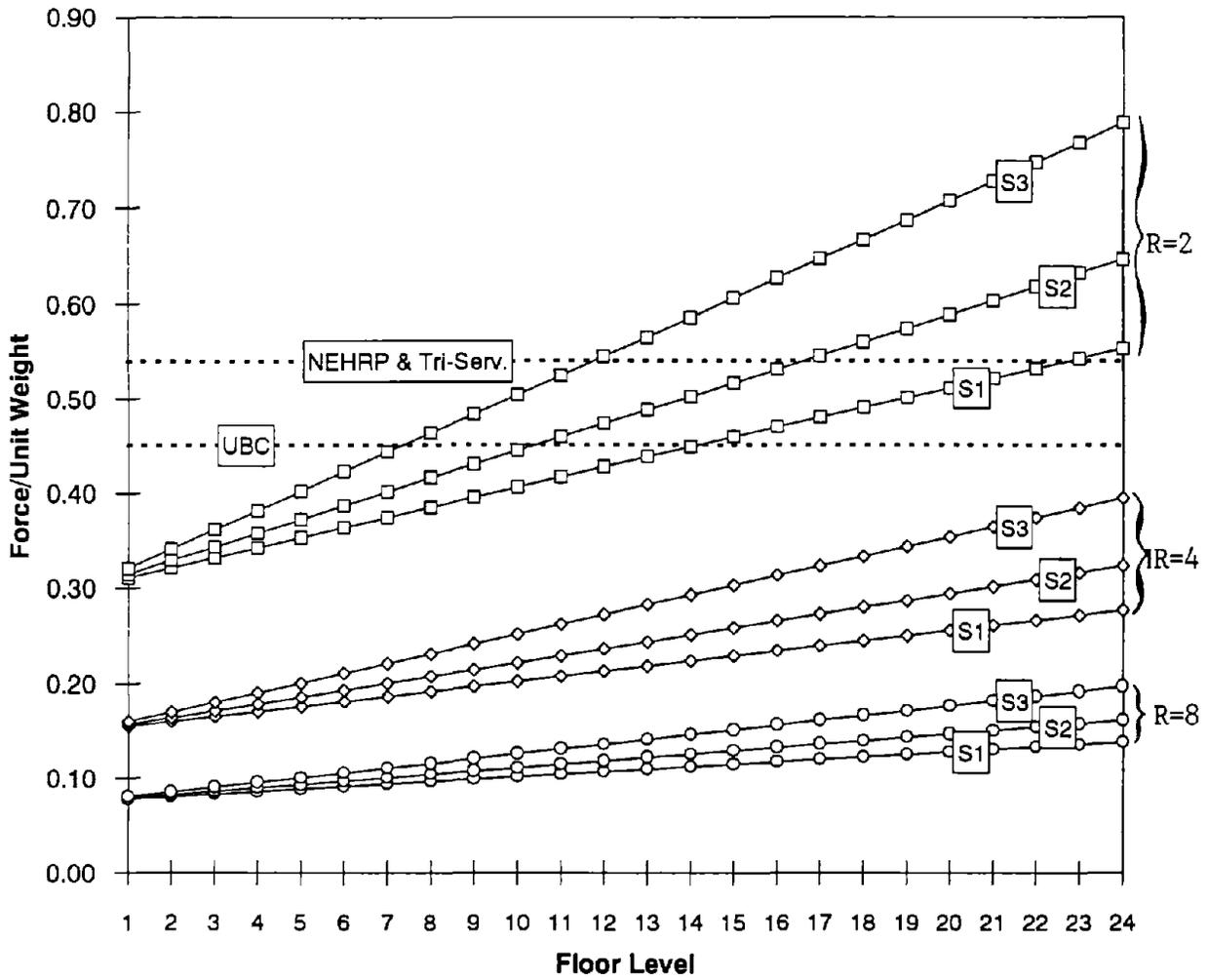
FIGURE 4.10: COMPARISON OF FORCES ON SUSPENDED CEILINGS CALCULATED BY VARIOUS CODE PROVISIONS AND SINGLE-MODE RESPONSE SPECTRUM APPROACH.
