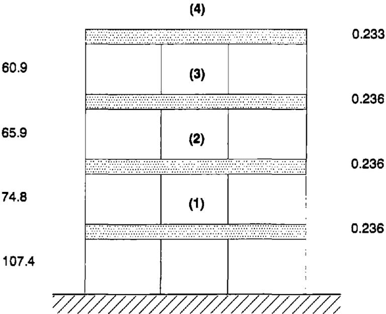
FIGURE 6.1: FOUR STORY SHEAR BUILDING USED IN THE STUDY.
