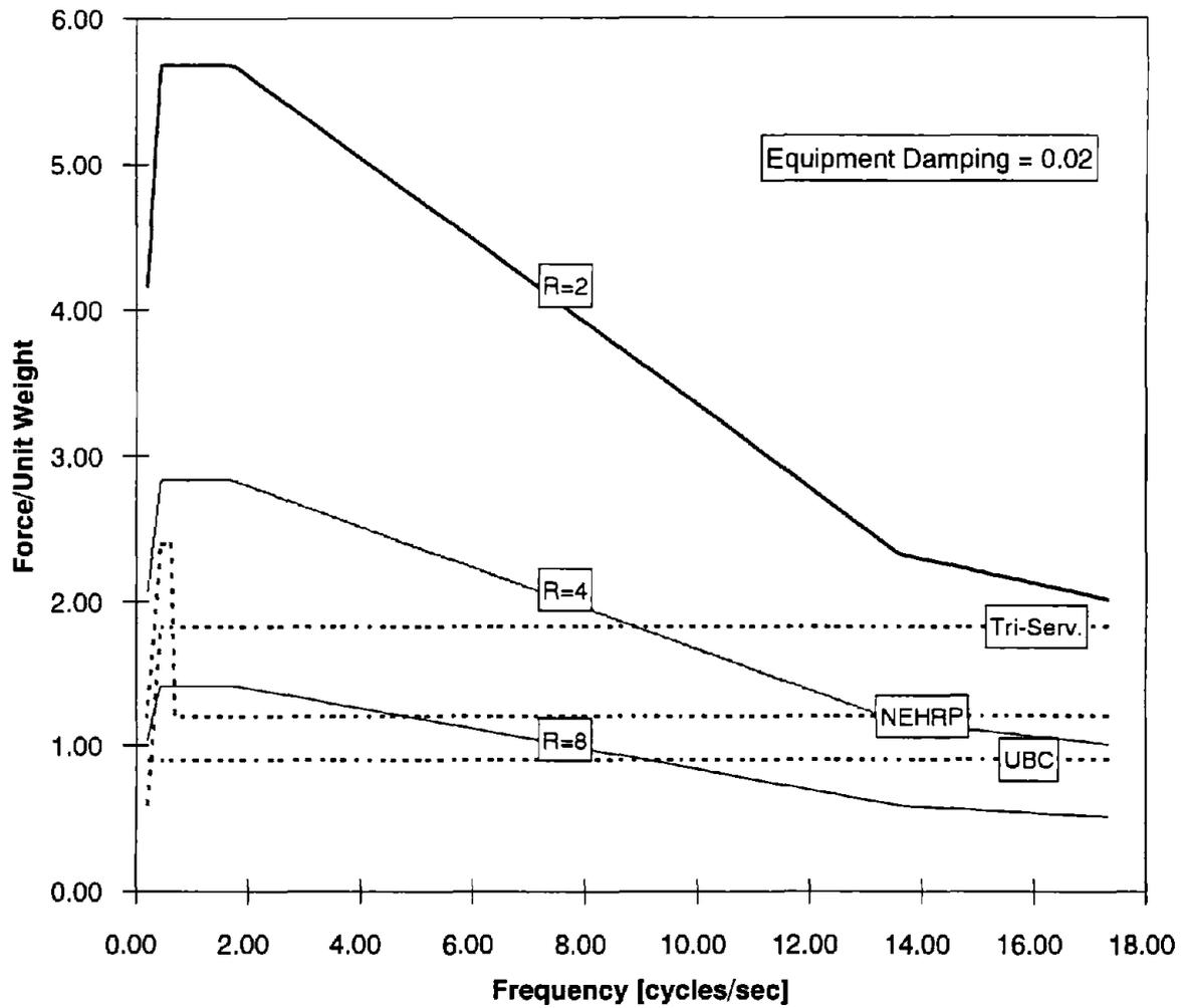
FIGURE 4.25: COMPARISON OF FLOOR 12 SPECTRA CALCULATED BY VARIOUS CODE PROVISIONS AND THE PROPOSED SIMPLIFIED APPROACH. GENERAL EQUIPMENT - SOIL S1
