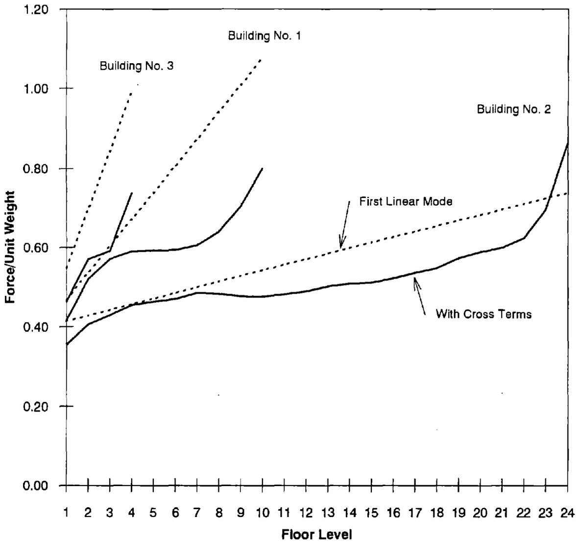
FIGURE A.5: COMPARISON OF FLOOR ACCELERATION CALCULATED WITH CROSS TERMS AND FIRST LINEAR MODE APPROACH FOR BUILDINGS 1,2 AND 3.
