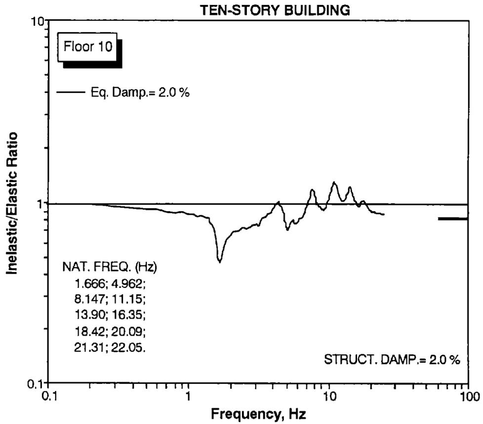
FIGURE 6.8: RATIO OF INELASTIC TO ELASTIC SPECTRA OF FLOOR 10
