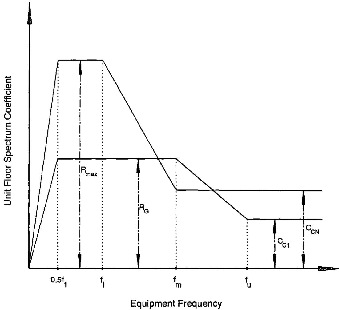
FIGURE B.7: FLOOR SPECTRA AT FIRST AND TOP FLOOR FOR SIMPLIFIED SINGLE MODE APPROACH.
