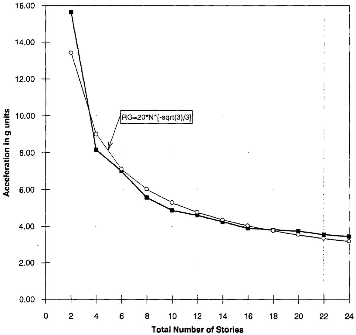
FIGURE B.8: PEAK FLOOR RESPONSE SPECTRUM VALUES FOR THE FIRST FLOOR OF UNIFORM BUILDINGS.
