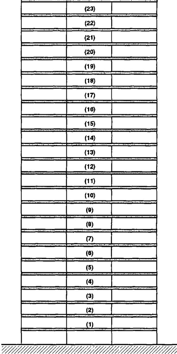
FIGURE 4.2: TWENTY FOUR STORY SHEAR BUILDING USED IN THE STUDY.
