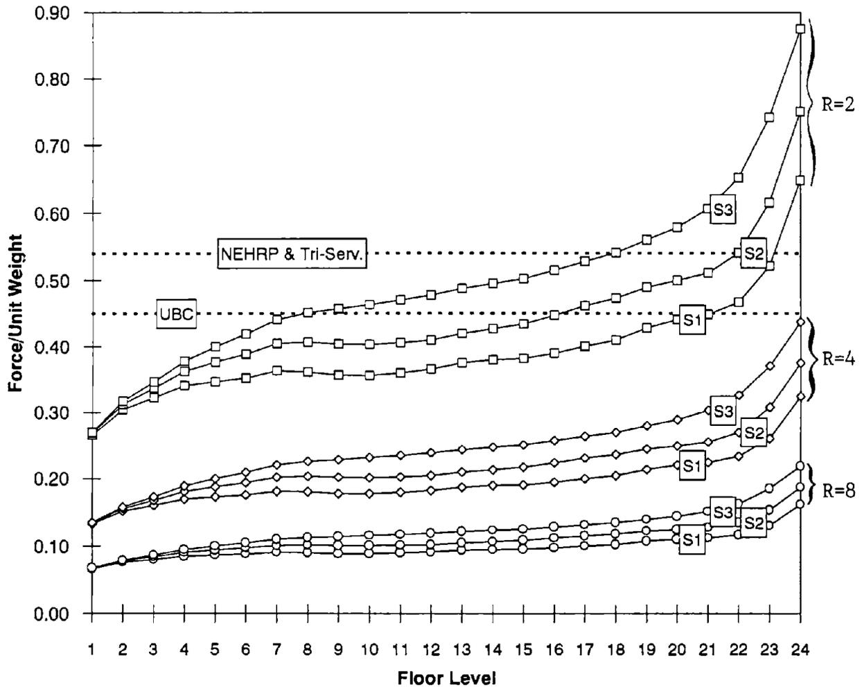
FIGURE 4.6: COMPARISON OF FORCES ON SUSPENDED CEILINGS CALCULATED BY VARIOUS CODE PROVISIONS AND MULTI-MODE RESPONSE SPECTRUM APPROACH.
