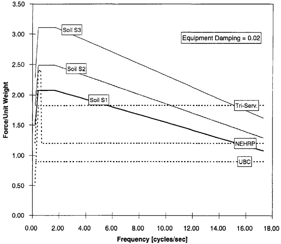
FIGURE 4.27: EFFECT OF SOIL TYPE ON THE FORCE ON GENERAL EQUIPMENT PLACED ON FLOOR 6.
