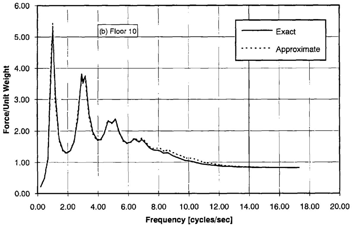
FIGURE 5.12: COMPARISON OF FLOOR SPECTRA FOR FLOORS 1 AND 10 CALCULATED WITH EXACT AND APPROXIMATE PROPERTIES. BUILDING NO. 1
