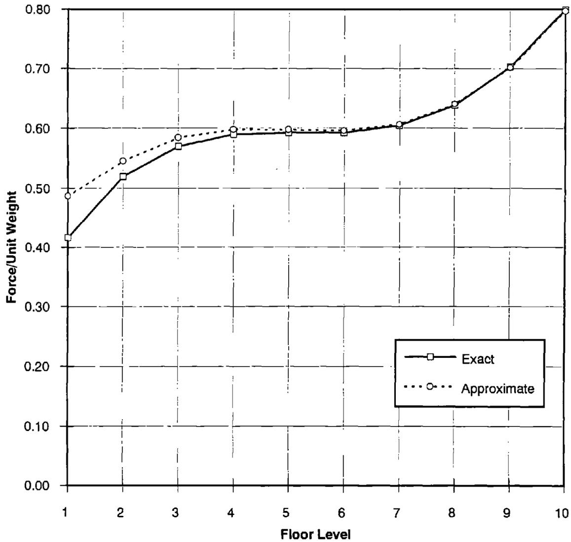
FIGURE 5.9: COMPARISON OF MAXIMUM FLOOR ACCELERATIONS CALCULATED WITH EXACT AND APPROXIMATE MODAL PROPERTIES. BUILDING NO. 1
