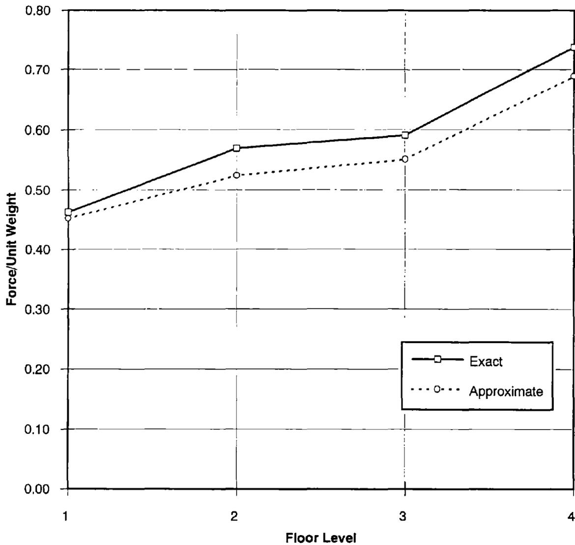
FIGURE 5.10: COMPARISON OF MAXIMUM FLOOR ACCELERATIONS CALCULATED WITH EXACT AND APPROXIMATE MODAL PROPERTIES. BUILDING NO. 3.
