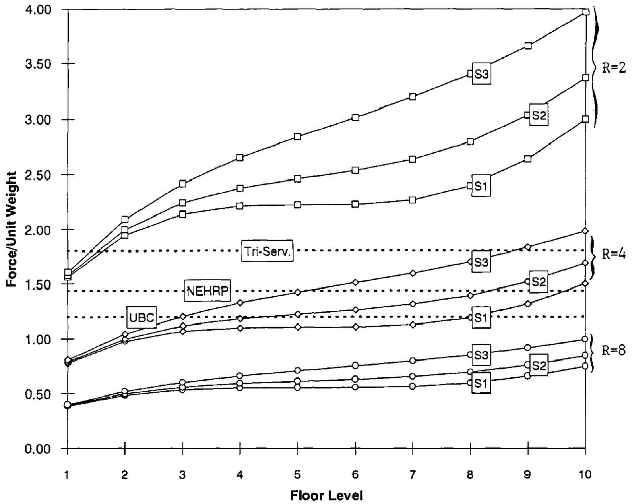
FIGURE 4.3: COMPARISON OF FORCES ON CANTILEVER PARAPETS CALCULATED BY VARIOUS CODE PROVISIONS AND MULTI-MODE RESPONSE SPECTRUM APPROACH.
