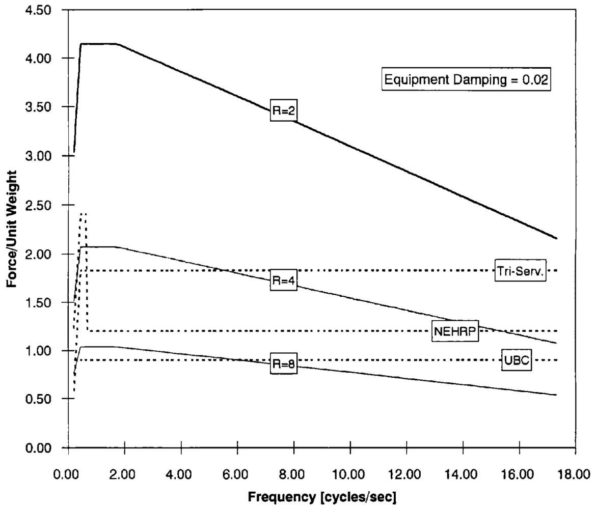
FIGURE 4.24: COMPARISON OF FLOOR 6 SPECTRA CALCULATED BY VARIOUS CODE PROVISIONS AND THE PROPOSED SIMPLIFIED APPROACH. GENERAL EQUIPMENT - SOIL S1
