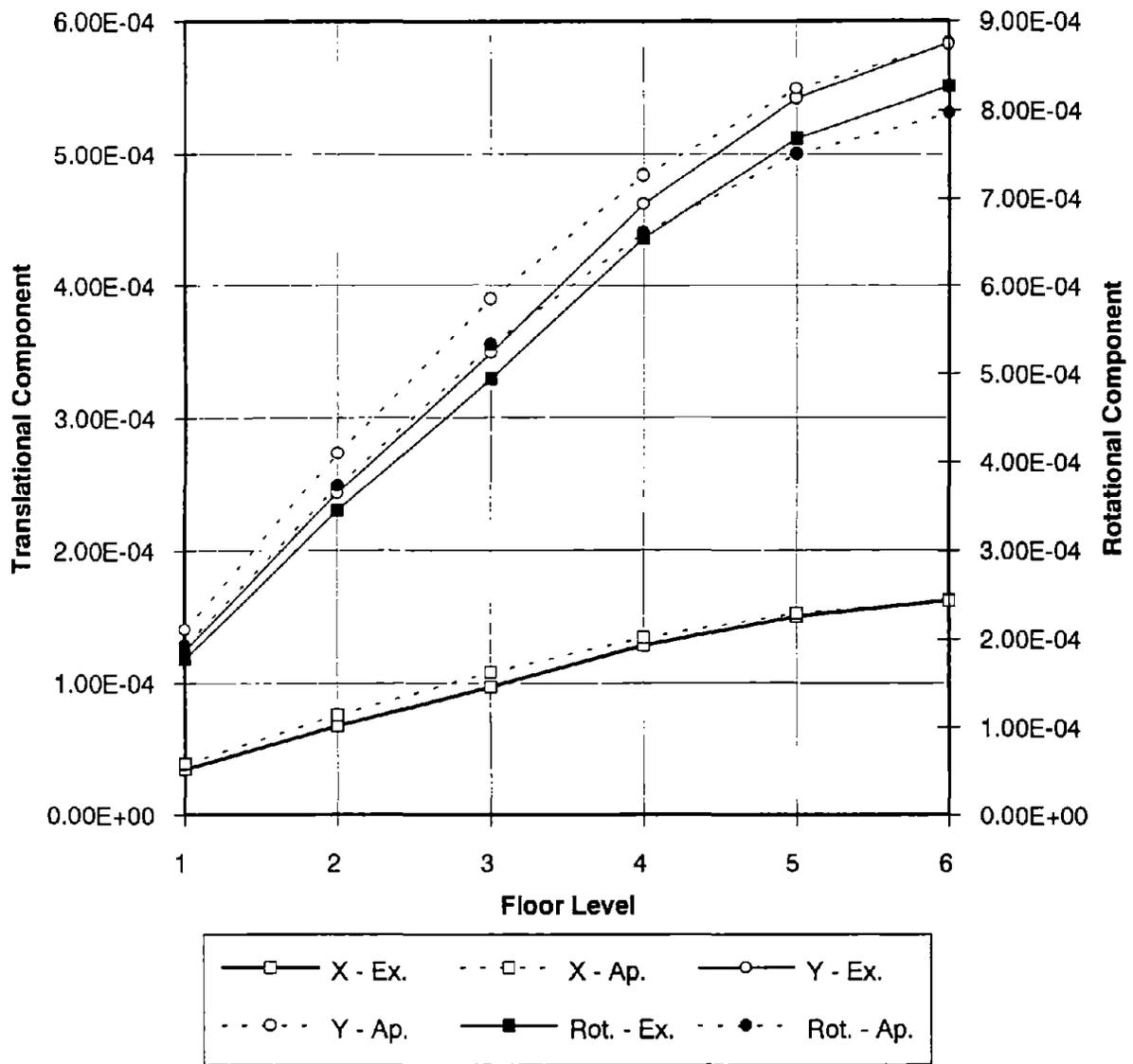
FIGURE 5.18: COMPARISON OF APPROXIMATE AND EXACT MODAL SHAPE OF MODE 3 OF THE TORSIONAL SYSTEM IN FIGURE 5.15
