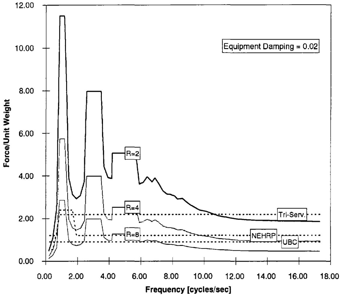
FIGURE 4.13: COMPARISON OF FLOOR 10 SPECTRA CALCULATED BY VARIOUS PROVISIONS AND THE PROPOSED RESPONSE SPECTRUM APPROACH. GENERAL EQUIPMENT - SOIL S1
