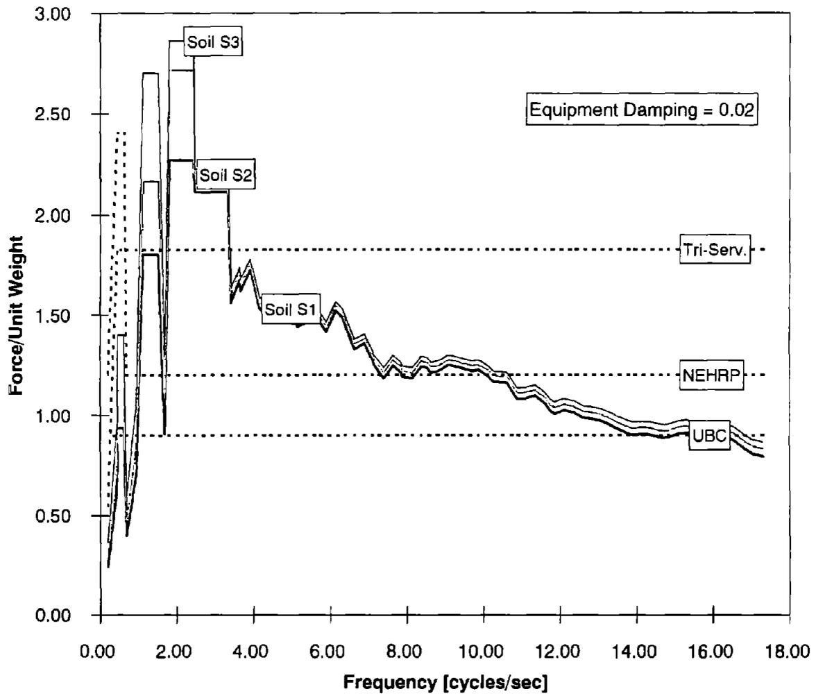
FIGURE 4.18: EFFECT OF SOIL TYPE ON THE FORCE ON GENERAL EQUIPMENT PLACED ON FLOOR 6.
