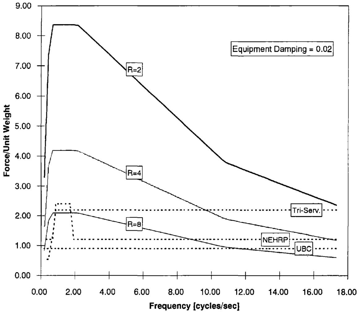
FIGURE 4.21: COMPARISON OF FLOOR 5 SPECTRA CALCULATED BY VARIOUS PROVISIONS AND THE PROPOSED SIMPLIFIED APPROACH. GENERAL EQUIPMENT - SOIL S1
