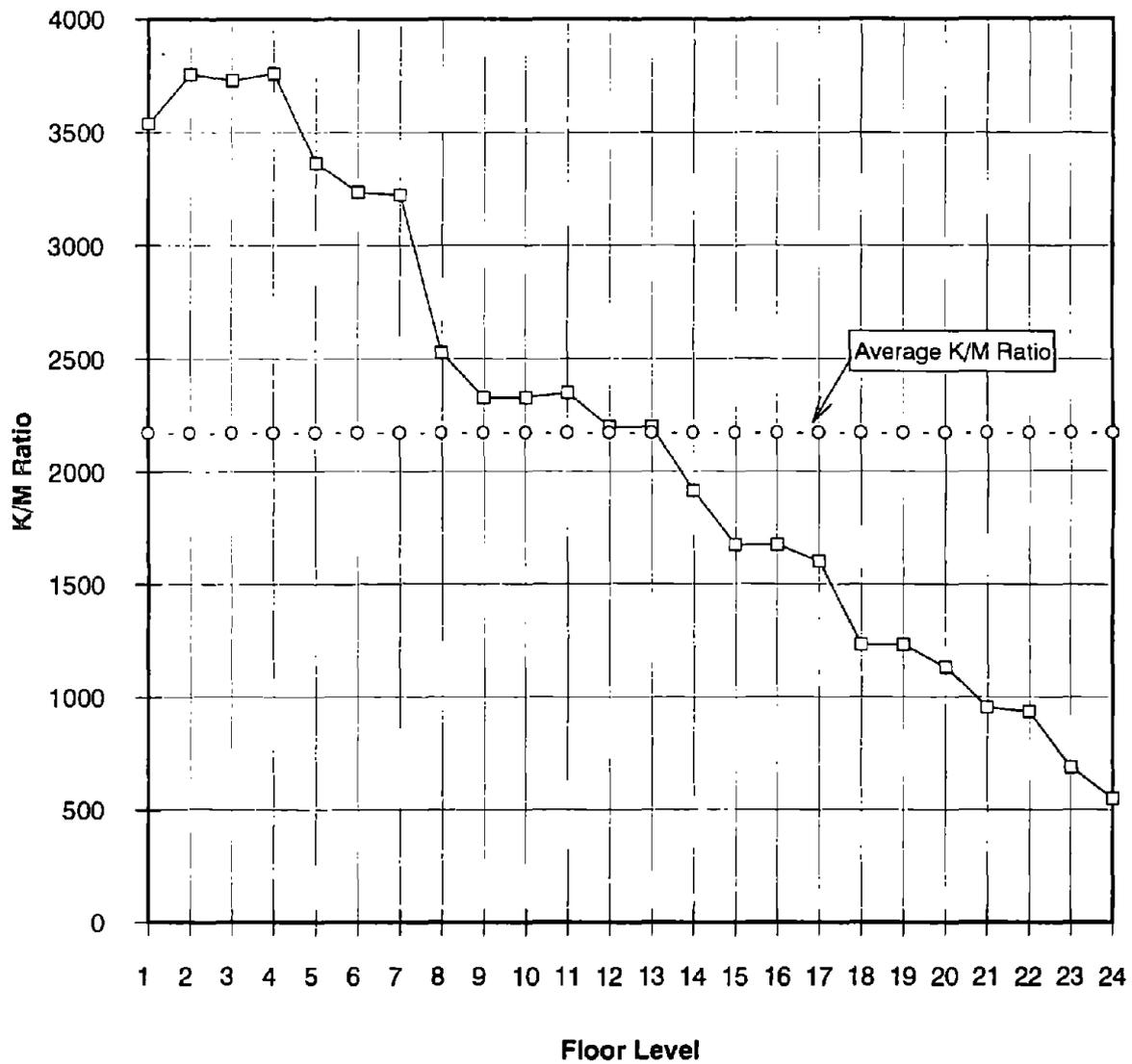
FIGURE 5.6: VARIATION OF K/M RATIO WITH HEIGHT FOR BUILDING NO. 2.
