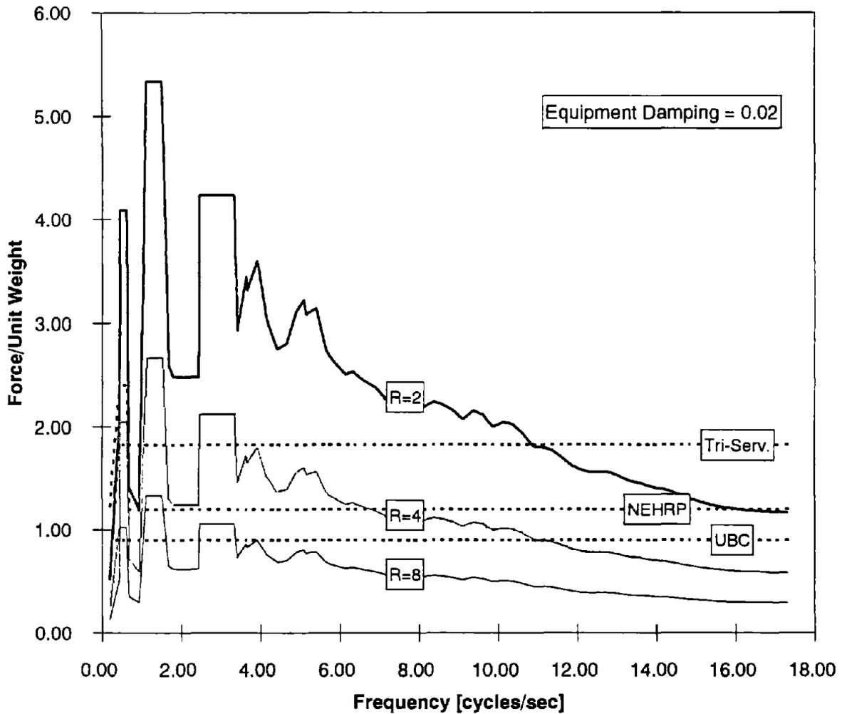
FIGURE 4.16: COMPARISON OF FLOOR 12 SPECTRA CALCULATED BY VARIOUS CODE PROVISIONS AND THE PROPOSED RESPONSE SPECTRUM APPROACH. GENERAL EQUIPMENT - SOIL S1
