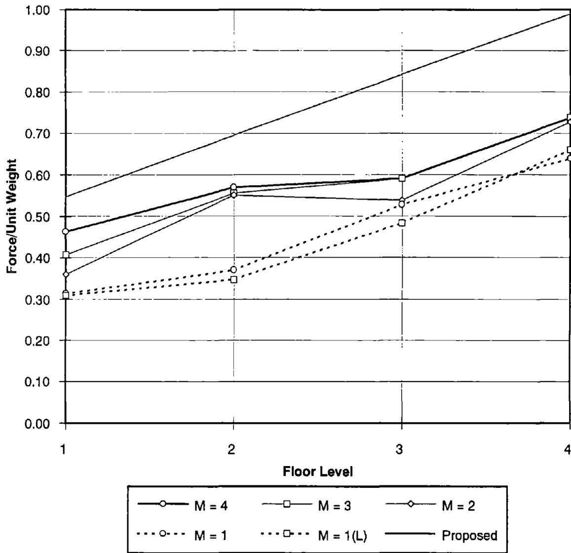
FIGURE 5.20: FLOOR ACCELERATIONS CALCULATED WITH INCREASING NUMBER OF MODES. BUILDING NO. 3
