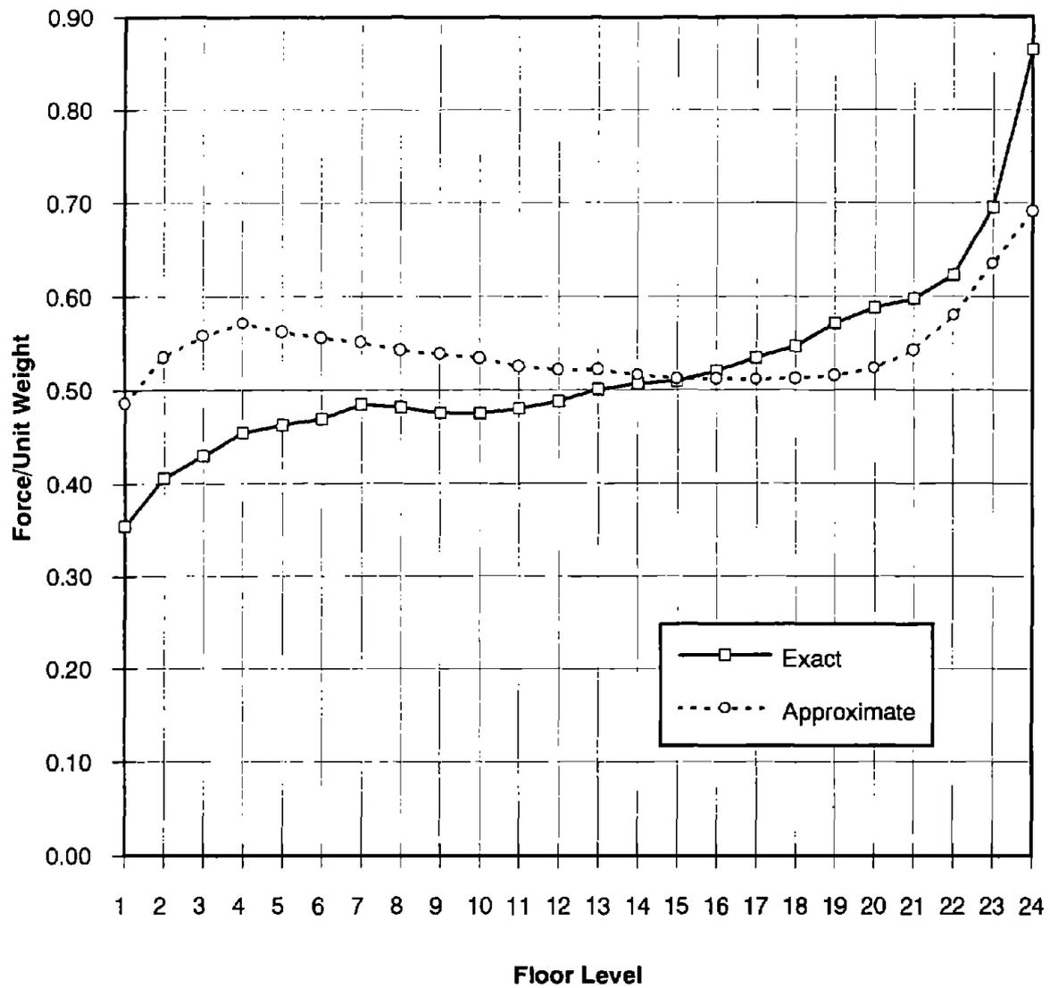
FIGURE 5.11: COMPARISON OF MAXIMUM FLOOR ACCELERATIONS CALCULATED WITH EXACT AND APPROXIMATE MODAL PROPERTIES. BUILDING NO. 2.
