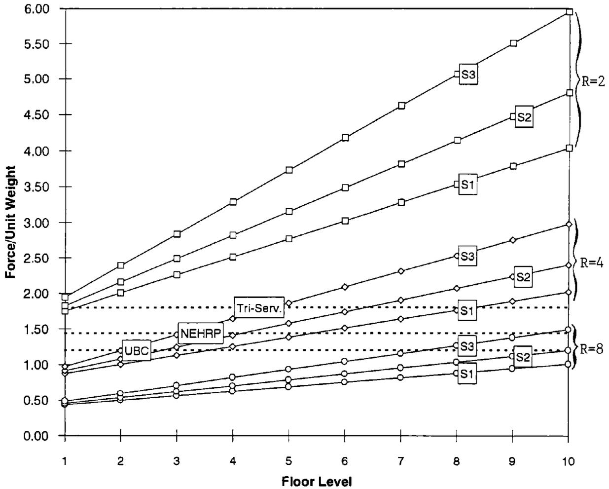
FIGURE 4.7: COMPARISON OF FORCES ON CANTILEVER PARAPETS CALCULATED BY VARIOUS CODE PROVISIONS AND SINGLE-MODE RESPONSE SPECTRUM APPROACH.
