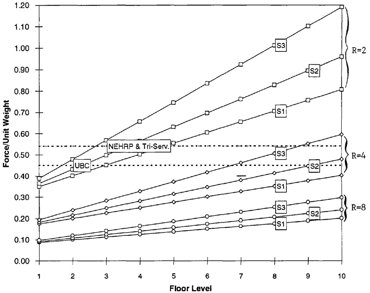
FIGURE 4.8: COMPARISON OF FORCES ON SUSPENDED CEILINGS CALCULATED BY VARIOUS CODE PROVISIONS AND SINGLE-MODE RESPONSE SPECTRUM APPROACH.
