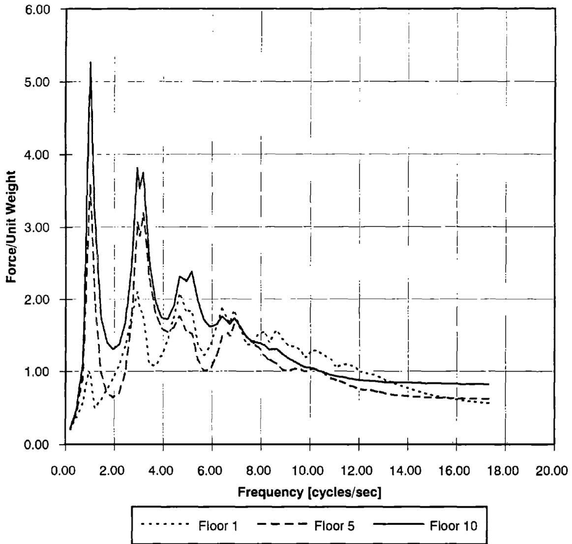
FIGURE 5.25: VARIATION OF FLOOR SPECTRA WITH FLOOR LEVEL.
