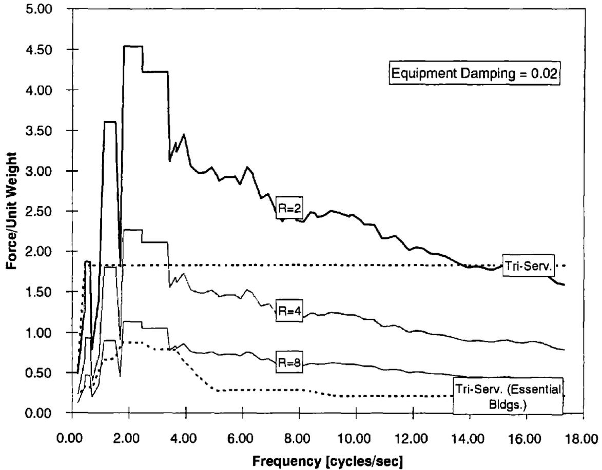
FIGURE 4.19: COMPARISON OF FORCE SPECTRA CALCULATED BY THE TWO TRI-SERVICES MANUALS AND THE PROPOSED RESPONSE SPECTRUM APPROACH. GENERAL EQUIPMENT - SOIL S1
