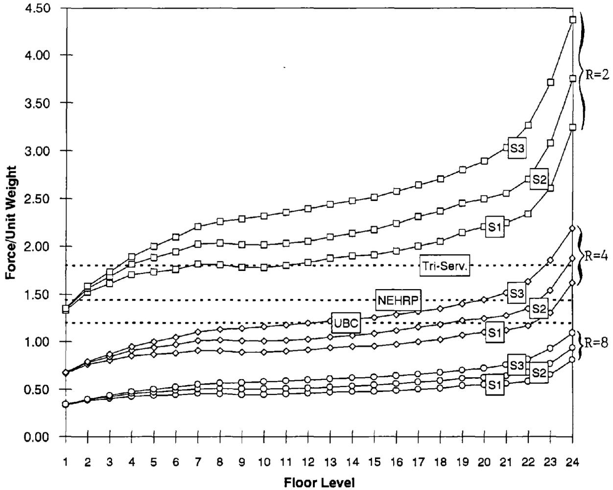
FIGURE 4.5: COMPARISON OF FORCES ON CANTILEVER PARAPETS CALCULATED BY VARIOUS CODE PROVISIONS AND MULTI-MODE RESPONSE SPECTRUM APPROACH.
