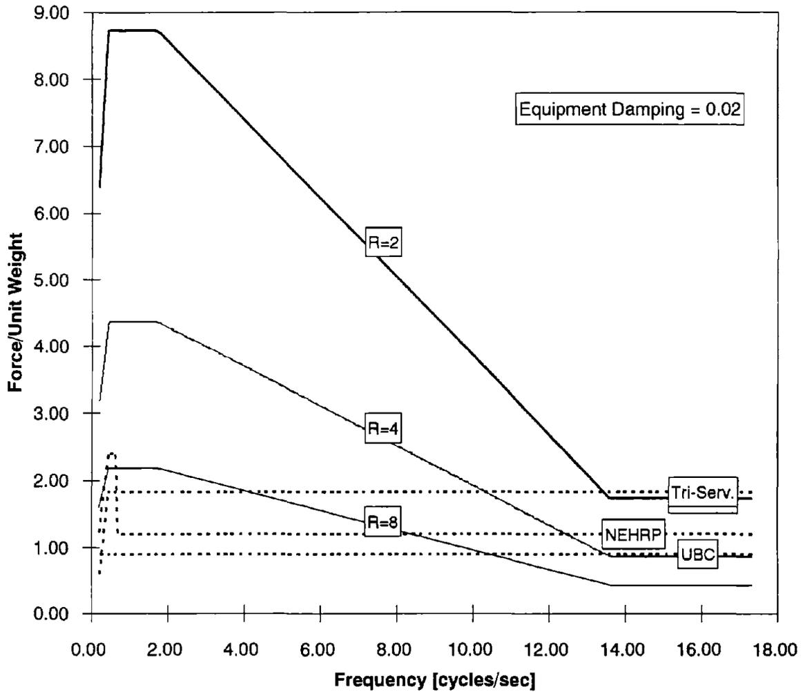
FIGURE 4.26: COMPARISON OF FLOOR 24 SPECTRA CALCULATED BY VARIOUS CODE PROVISIONS AND THE PROPOSED SIMPLIFIED APPROACH. GENERAL EQUIPMENT - SOIL S1
