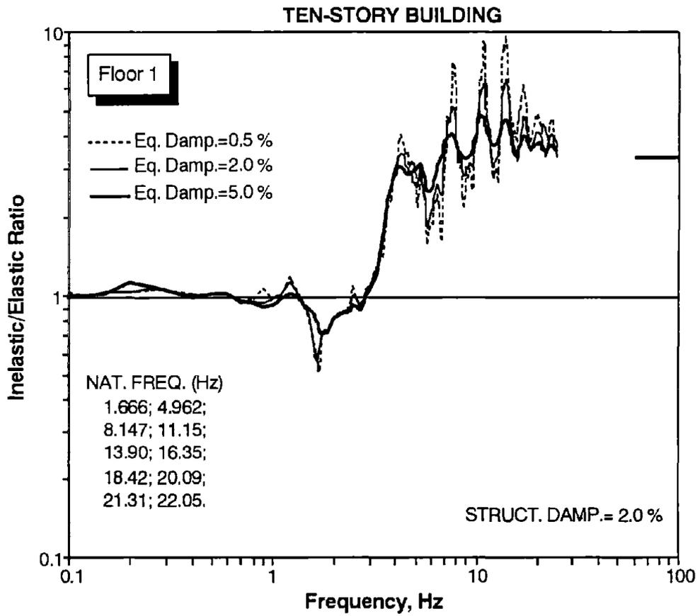
FIGURE 6.11: RATIO OF INELASTIC TO ELASTIC SPECTRA FOR FLOOR 1
