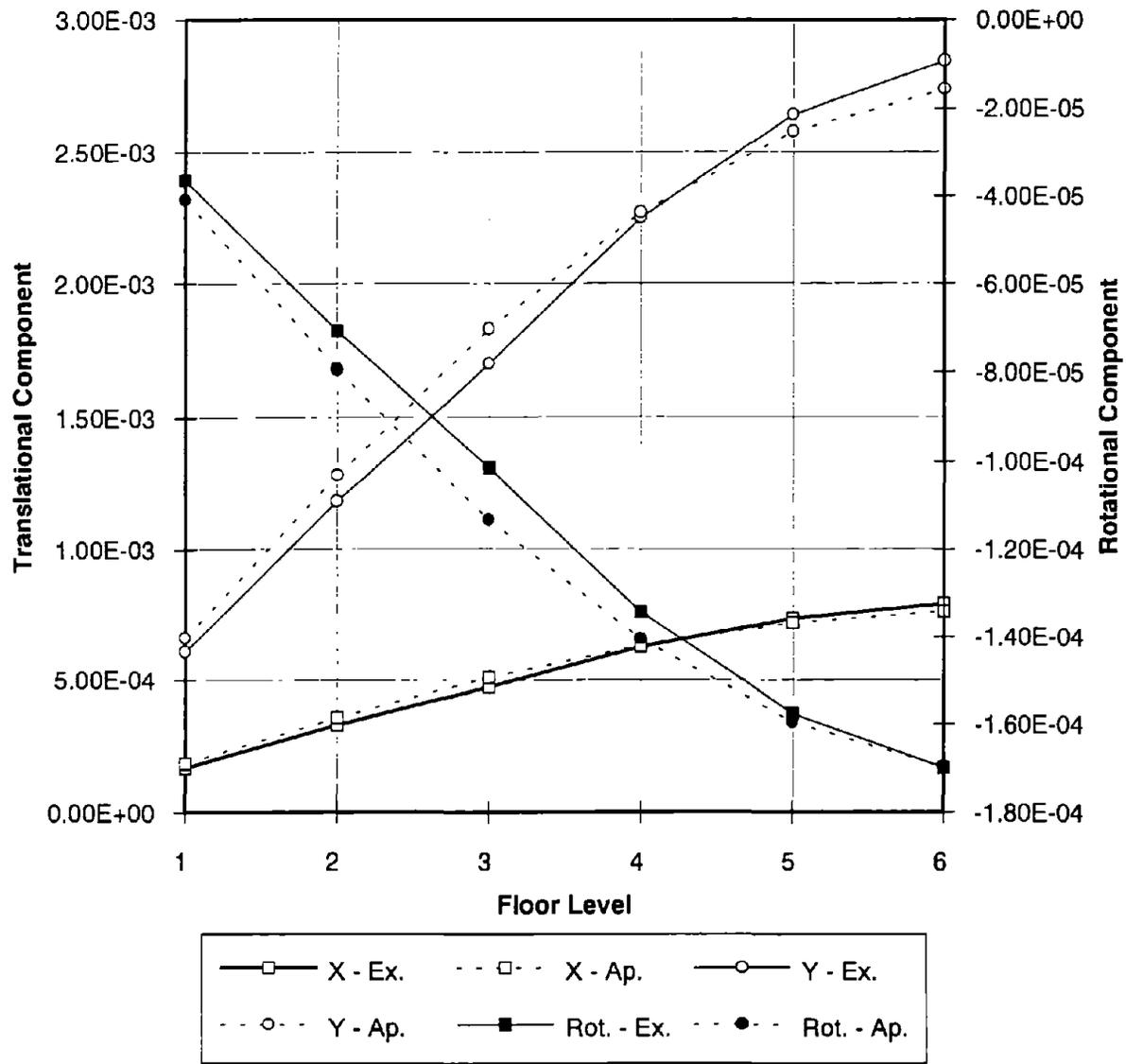
FIGURE 5.17: COMPARISON OF APPROXIMATE AND EXACT MODAL SHAPE OF MODE 1 OF THE TORSIONAL SYSTEM IN FIGURE 5.15
