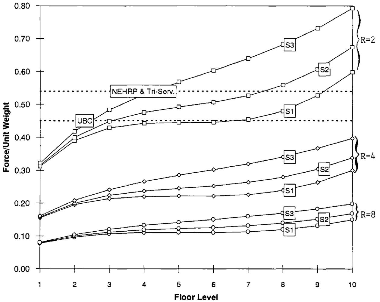
FIGURE 4.4: COMPARISON OF FORCES ON SUSPENDED CEILINGS CALCULATED BY VARIOUS CODE PROVISIONS AND MULTI-MODE RESPONSE SPECTRUM APPROACH.
