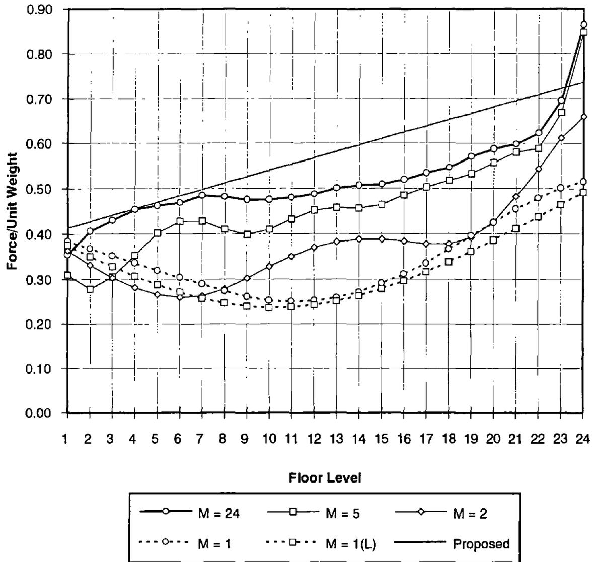
FIGURE 5.21: FLOOR ACCELERATIONS CALCULATED WITH INCREASING NUMBER OF MODES. BUILDING NO. 2
