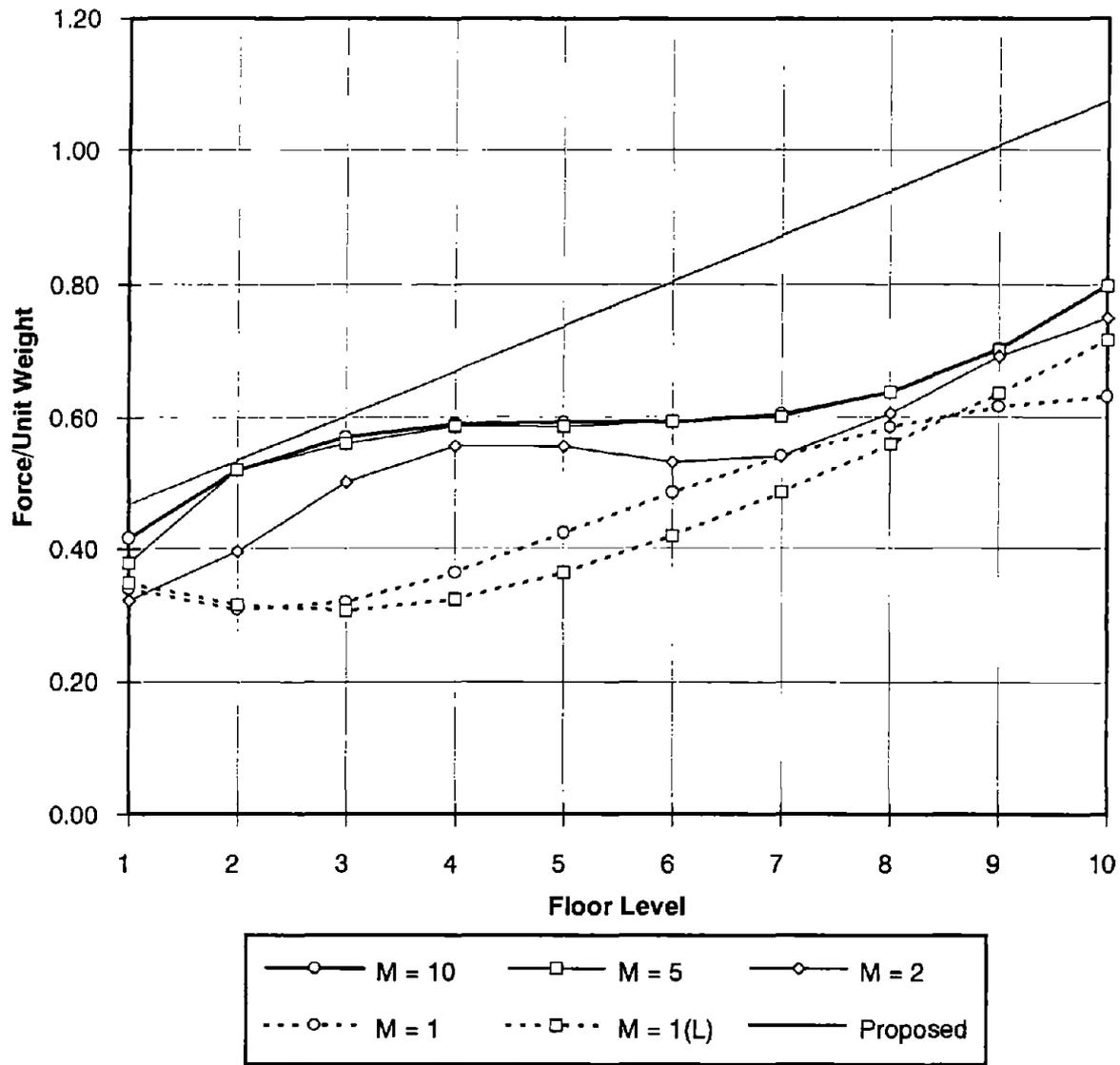
FIGURE 5.19: FLOOR ACCELERATIONS CALCULATED WITH INCREASING NUMBER OF MODES. BUILDING NO. 1
