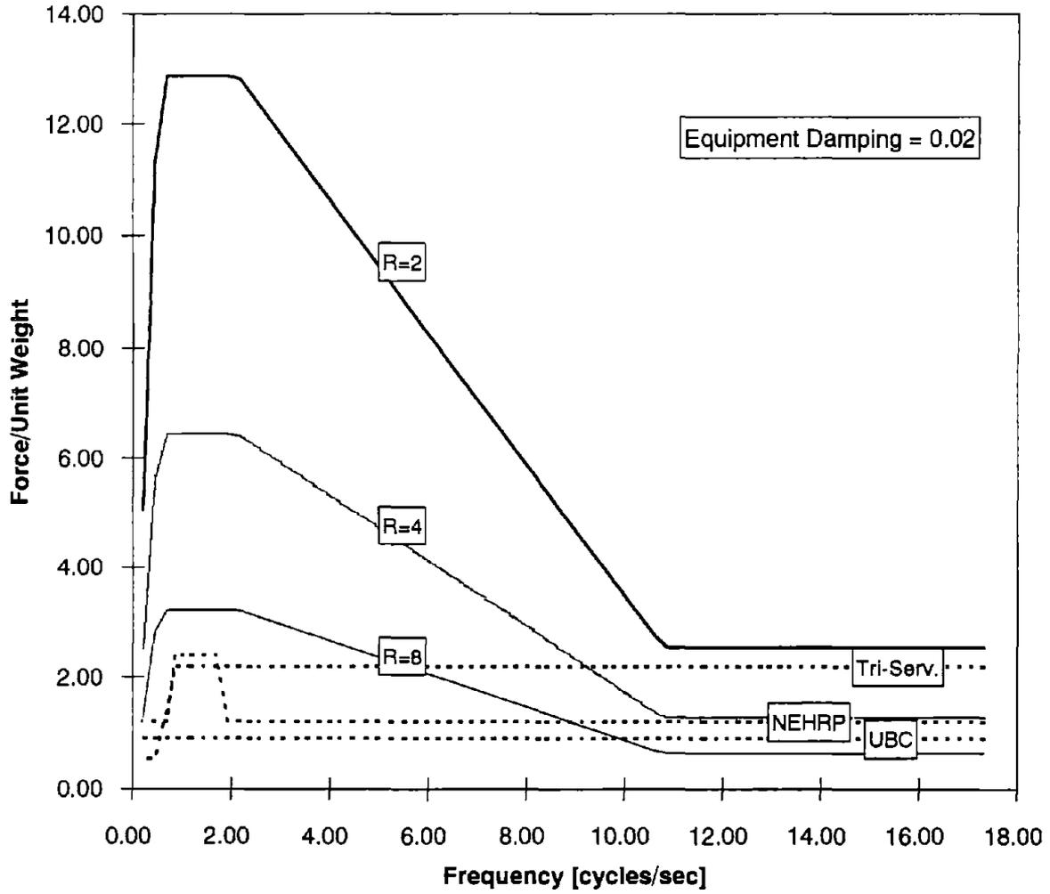
FIGURE 4.22: COMPARISON OF FLOOR 10 SPECTRA CALCULATED BY VARIOUS PROVISIONS AND THE PROPOSED SIMPLIFIED APPROACH. GENERAL EQUIPMENT - SOIL S1
