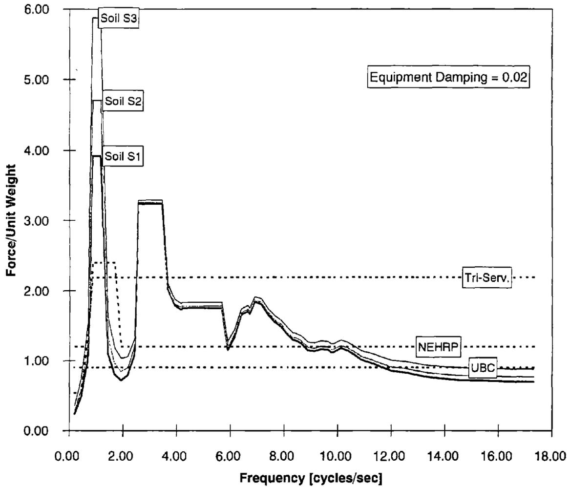
FIGURE 4.14: EFFECT OF SOIL TYPE ON THE FORCE ON GENERAL EQUIPMENT PLACED ON FLOOR 5.
