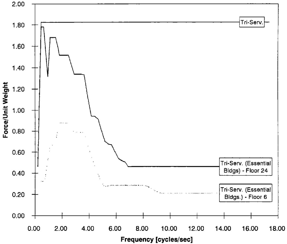
FIGURE 4.20: COMPARISON OF FORCE SPECTRA OBTAINED BY THE TWO TRI-SERVICES MANUALS.
