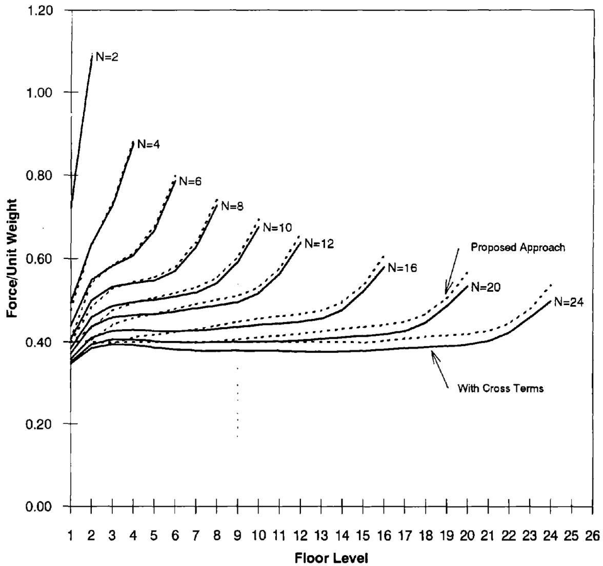
FIGURE A.2: COMPARISON OF FLOOR ACCELERATION CALCULATED WITH CROSS TERMS AND PROPOSED APPROACH FOR UNIFORM BUILDINGS OF DIFFERENT HEIGHTS.
