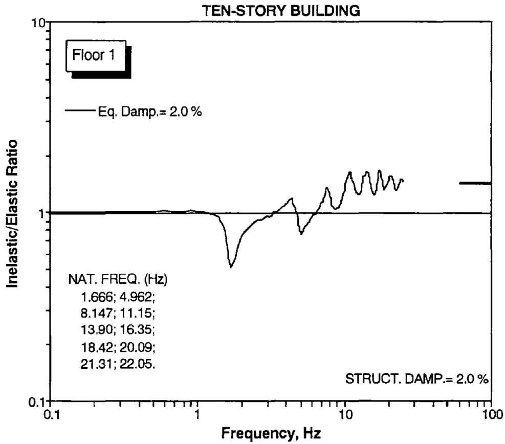
FIGURE 6.6: RATIO OF INELASTIC TO ELASTIC SPECTRA OF FLOOR 1
