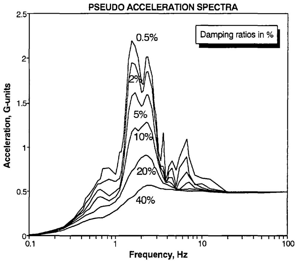
FIGURE 6.9: GROUND RESPONSE SPECTRA FOR PARKFIELD EARTHQUAKE (1966, CHOLAME-SHANDON ARRAY #2, N65E)
