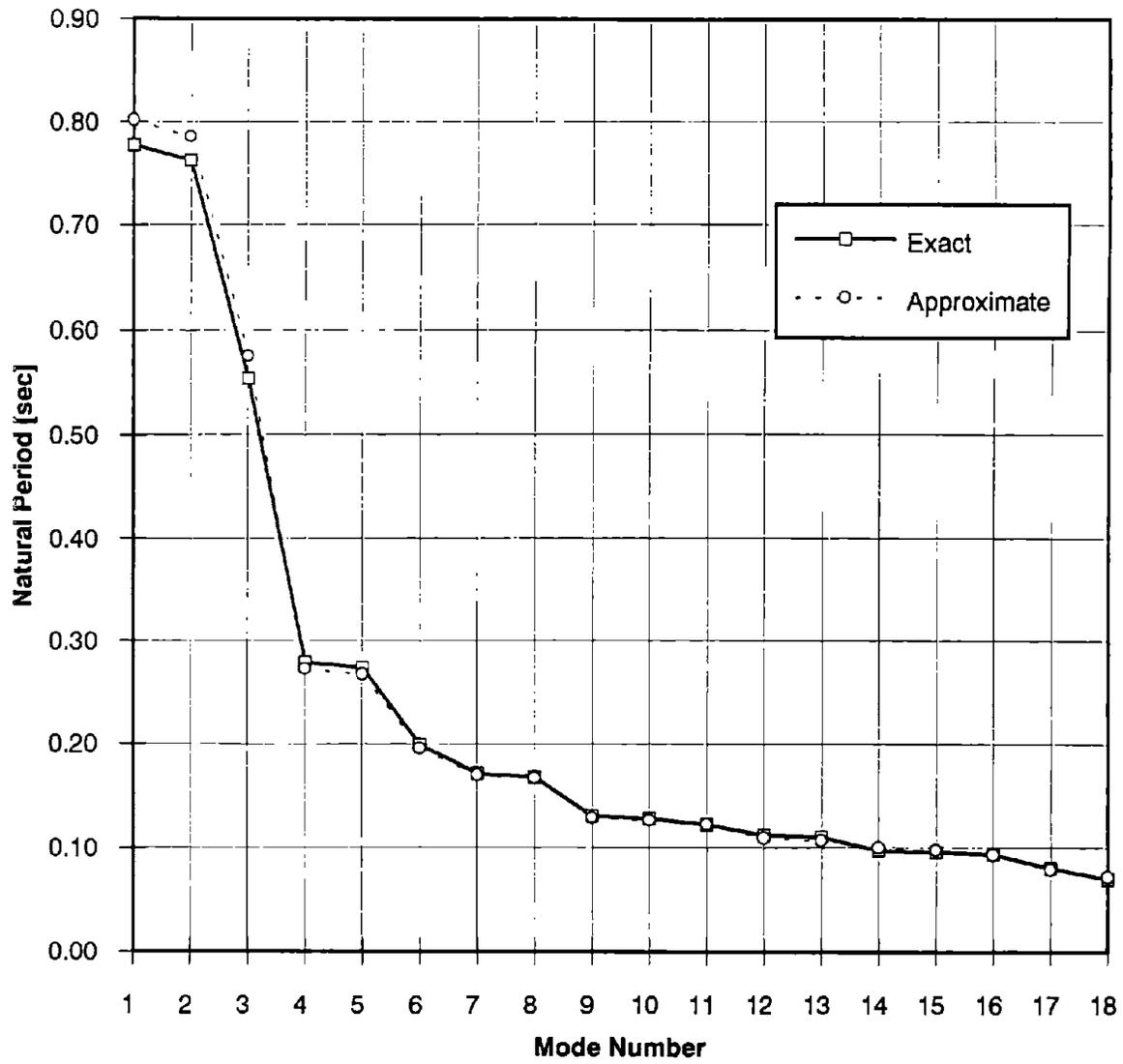
FIGURE 5.16: COMPARISON OF APPROXIMATE AND EXACT MODAL PERIODS OF THE TORSIONAL SYSTEM IN FIGURE 5.15
