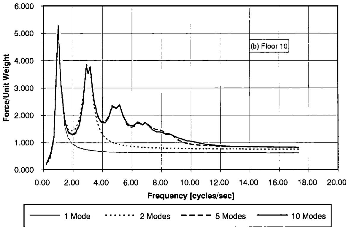
FIGURE 5.22: FLOOR SPECTRA FOR FLOORS 1 AND 10 CALCULATED WITH INCREASING NUMBER OF MODES.
