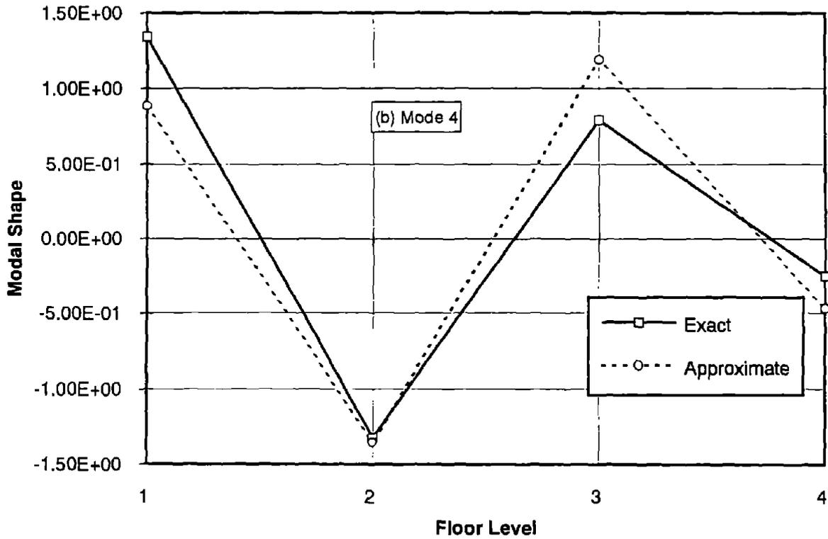
FIGURE 5.5: COMPARISON OF EXACT AND APPROXIMATE MODAL SHAPE FOR MODE 1 AND MODE 4. BUILDING NO. 3.
