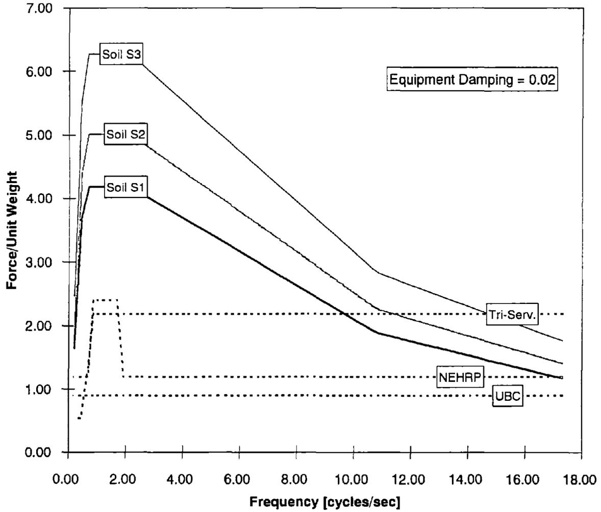
FIGURE 4.23: EFFECT OF SOIL TYPE ON THE FORCE ON GENERAL EQUIPMENT PLACED ON FLOOR 5.
