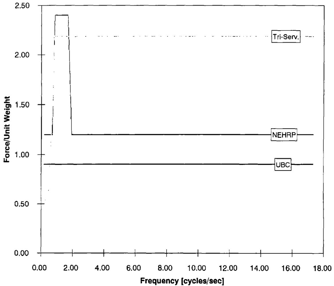
FIGURE 4.11: COMPARISON OF FORCES SPECTRA FOR GENERAL EQUIPMENT ACCORDING TO NEHRP PROVISIONS, TRI-SERVICES MANUAL AND UBC.
