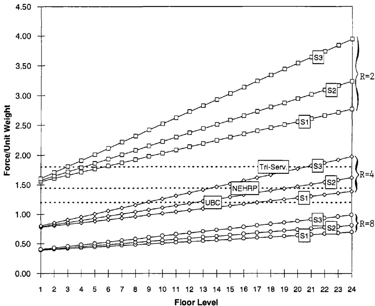
FIGURE 4.9: COMPARISON OF FORCES ON CANTILEVER PARAPETS CALCULATED BY VARIOUS CODE PROVISIONS AND SINGLE-MODE RESPONSE SPECTRUM APPROACH.
