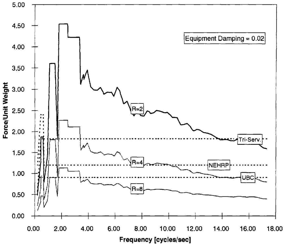
FIGURE 4.15: COMPARISON OF FLOOR 6 SPECTRA CALCULATED BY VARIOUS CODE PROVISIONS AND THE PROPOSED RESPONSE SPECTRUM APPROACH. GENERAL EQUIPMENT - SOIL S1
