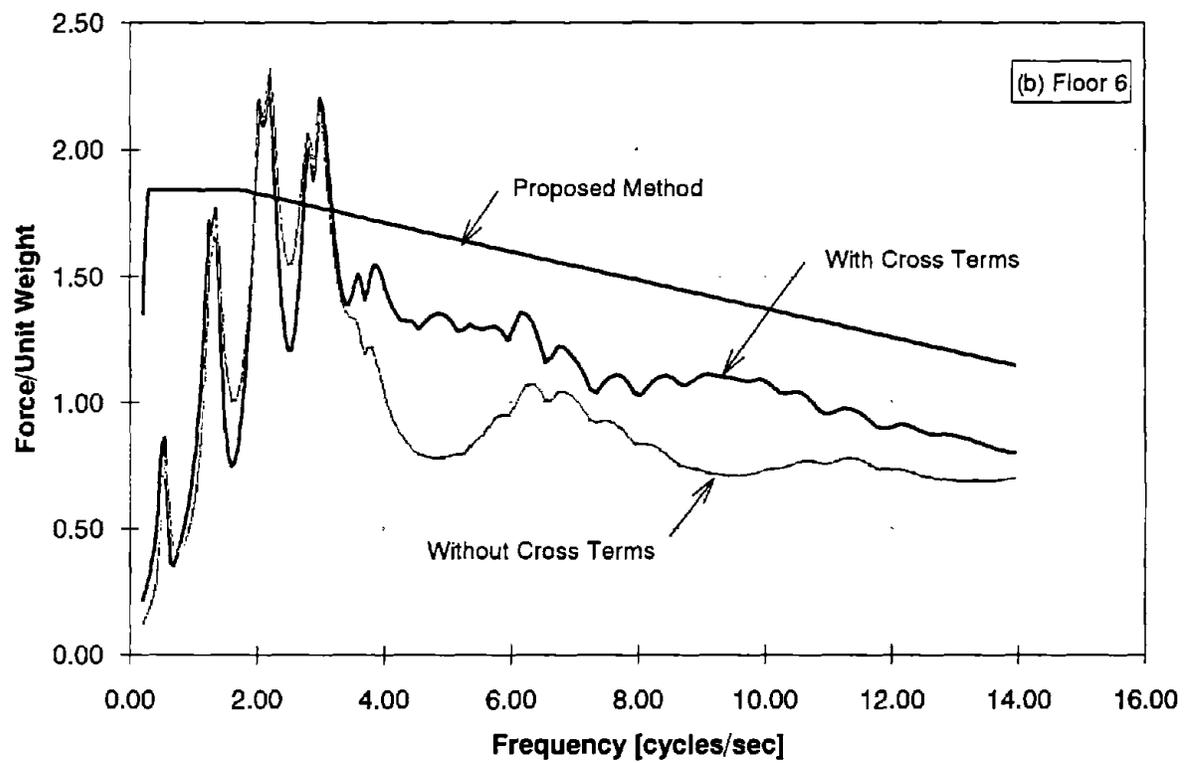
FIGURE B.4: COMPARISON OF FLOOR RESPONSE SPECTRA FOR FIRST AND SIXTH FLOOR OF BUILDING NO. 2.
