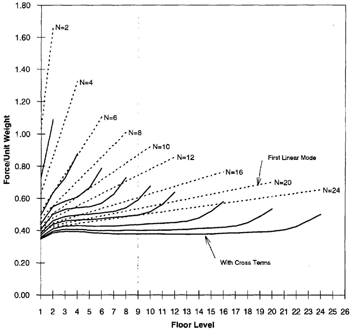
FIGURE A.4: COMPARISON OF FLOOR ACCELERATION CALCULATED WITH CROSS TERMS AND FIRST LINEAR MODE APPROACH FOR UNIFORM BUILDINGS OF DIFFERENT HEIGHTS.
