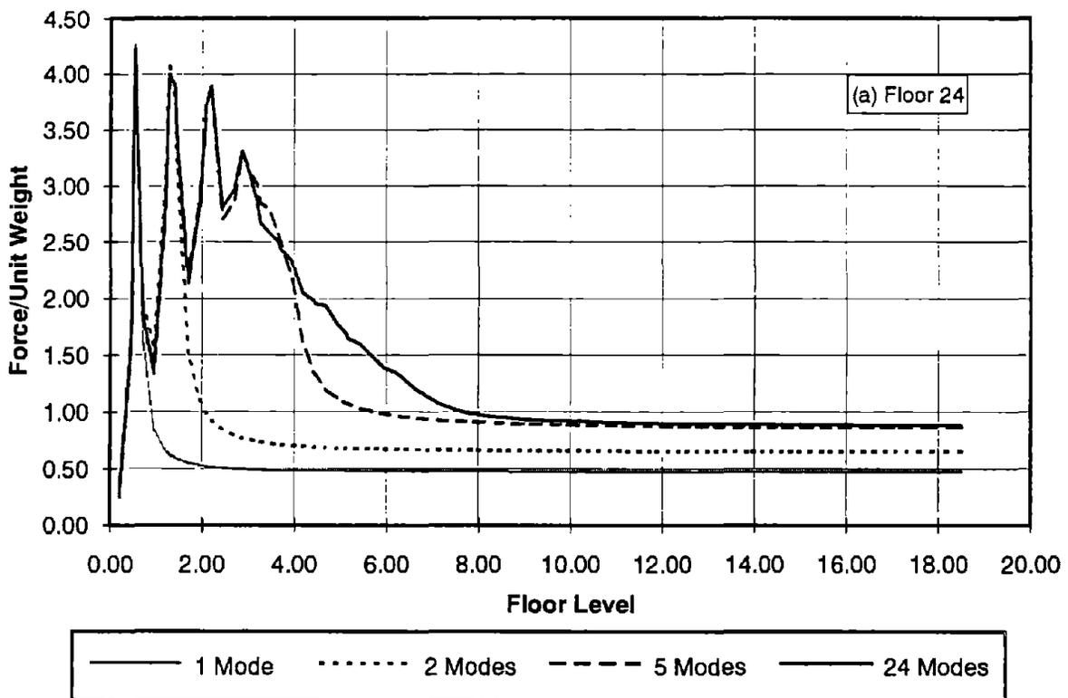
FIGURE 5.23: FLOOR SPECTRA FOR FLOORS 1 AND 24 CALCULATED WITH INCREASING NUMBER OF MODES.
