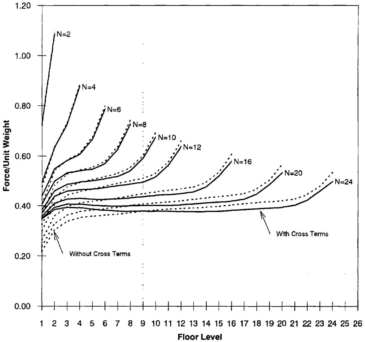
FIGURE A.1: COMPARISON OF FLOOR ACCELERATION CALCULATED WITH AND WITHOUT CROSS TERMS FOR UNIFORM BUILDINGS OF DIFFERENT HEIGHTS.
