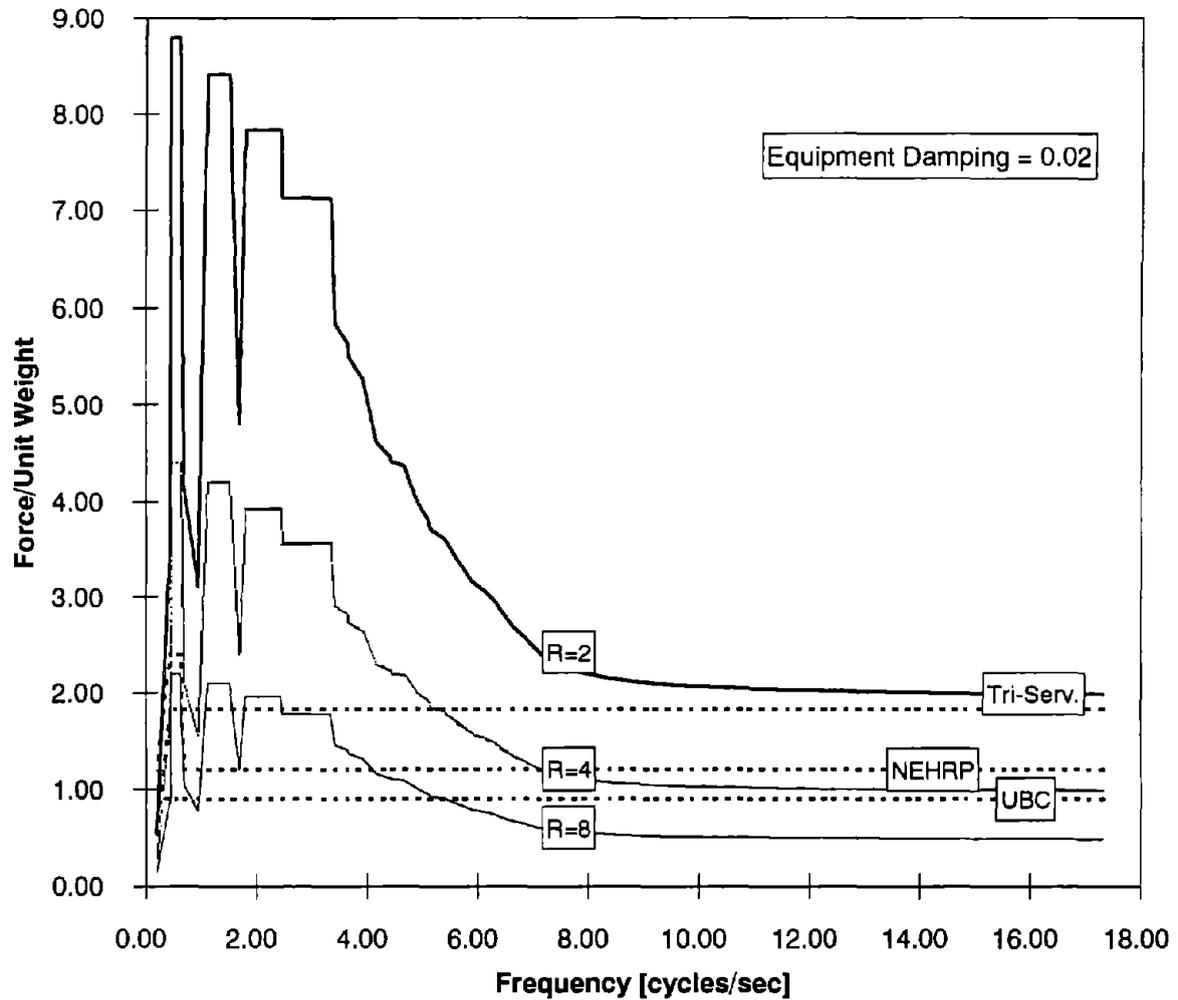
FIGURE 4.17: COMPARISON OF FLOOR 24 SPECTRA CALCULATED BY VARIOUS CODE PROVISIONS AND THE PROPOSED RESPONSE SPECTRUM APPROACH. GENERAL EQUIPMENT - SOIL S1
