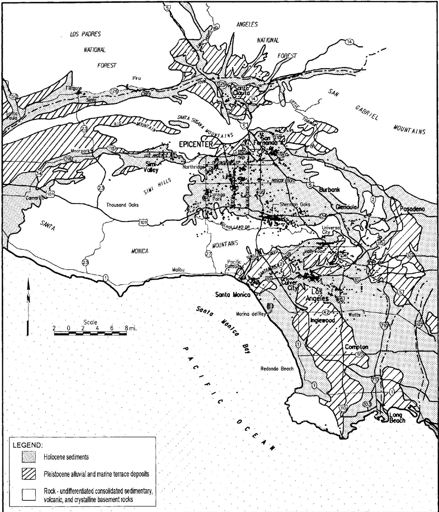
Fig. 3.24: Damage patterns from the 1994 Northridge Earthquake and generalized geologic conditions in the Los Angeles Area (Sources: Governor's Office of Emergency Services, 1994; Los Angeles County, 1990; California Division of Mines and Geology, 1969)
