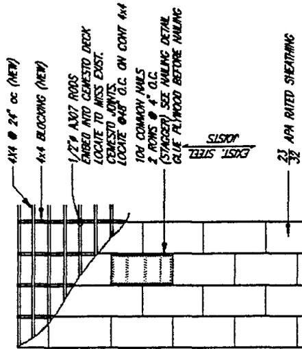
PLYWOOD INSTALLATION DIAGRAM
