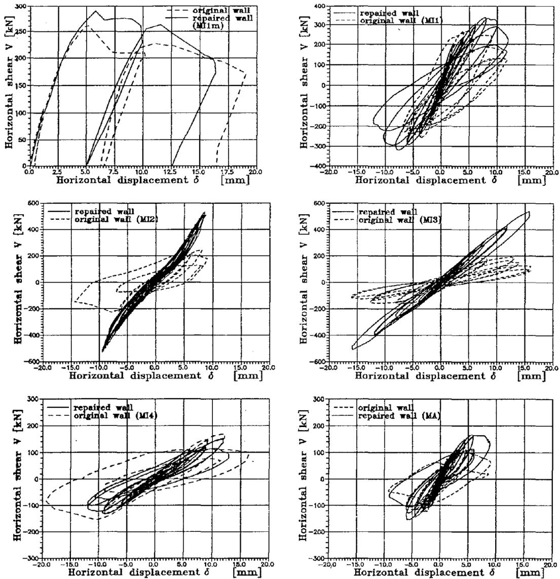
Fig. 1. Results of the shear-compression tests on brick masonry walls. Dashed line: original walls; solid line: repaired walls.
