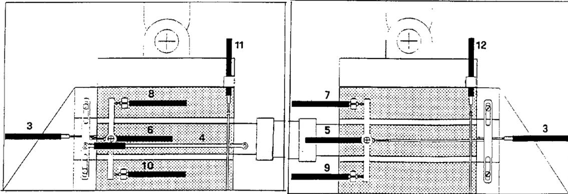
Fig. 17 - Design for displacement measurements on the triplet
