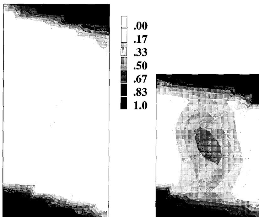
Figure 12- Computed damage index at maximum lateral displacement: the high wall fails by rocking whereas the low wall fails by diagonal cracking.
