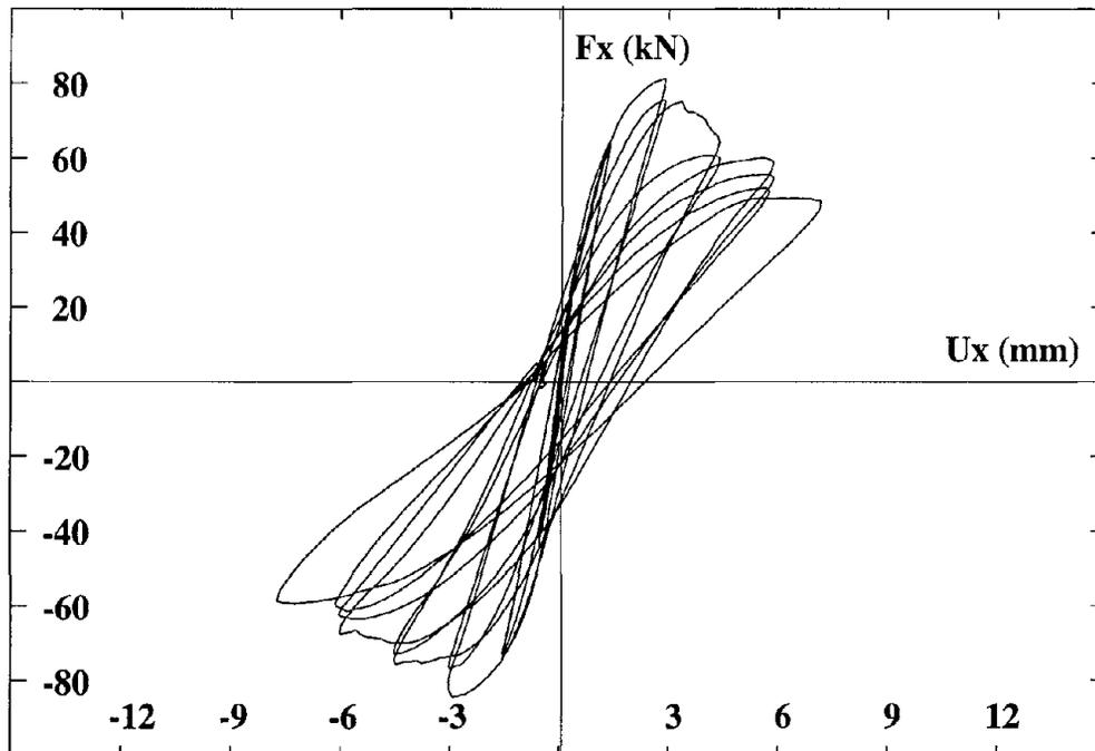
Figure 5- Horizontal force  $F_x$  versus lateral displacement  $U_x$  for the low wall.
