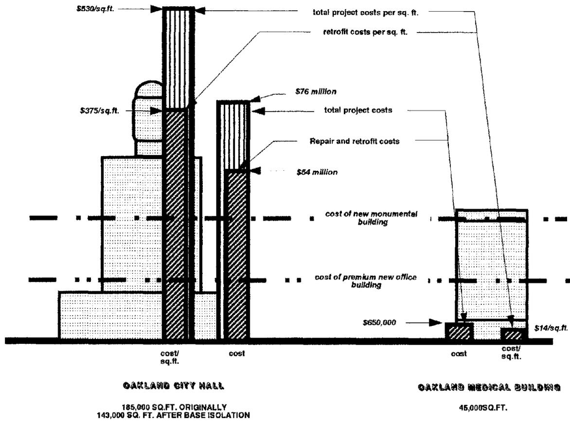
FIGURE 1: COST COMPARISON BETWEEN TWO RETROFIT PROJECTS
