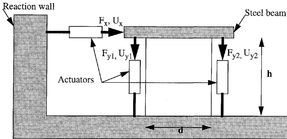
Figure 4- Schematic view of the test set-up.
