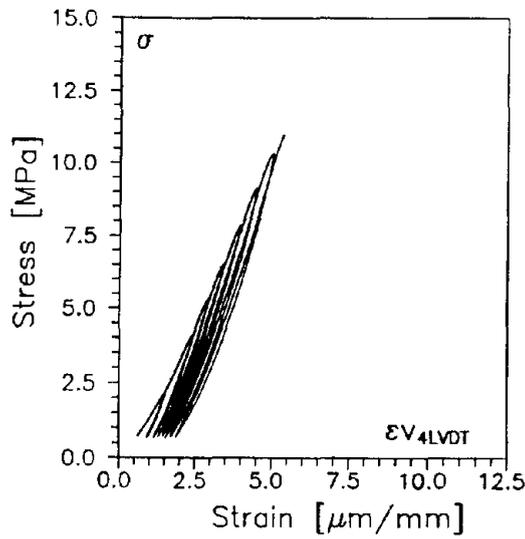
Fig. 16a - Stress-strain plot for EB under cyclic vertical load
