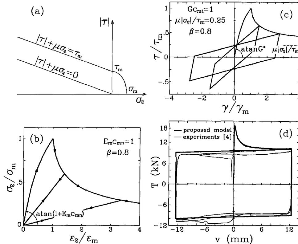
Figure 1. Damage model for mortar joint: (a) sliding and failure curves in the  $(\sigma_2, |\tau|)$  plane; (b) model response to tensile stresses; (c) model response to cyclic shearing strains; (d) simulation of direct shear tests by Atkinson et al. [4].
