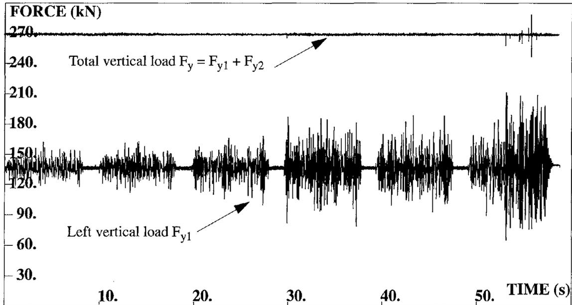
Figure 8- Total and left vertical loads during the pseudo dynamic test.
