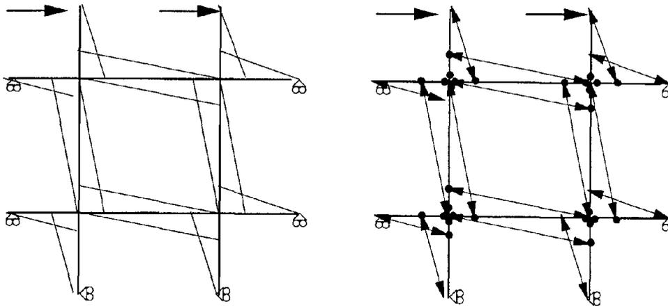
Fig. 9. Simple Model of Infill Strut Behavior
