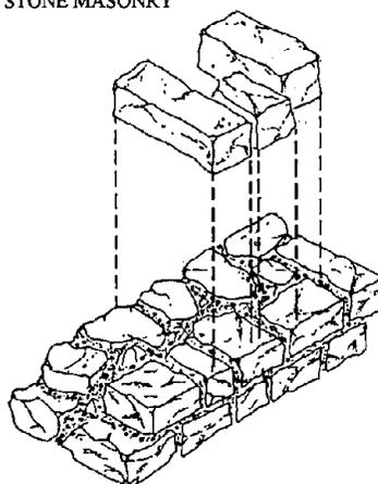
The masonry wall is made of superimposed stones: their interlocking conditions the possibility of an "monolithic" behaviour.
