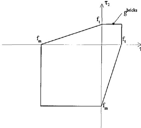
*Figure 7 Strength condition for bricks*
