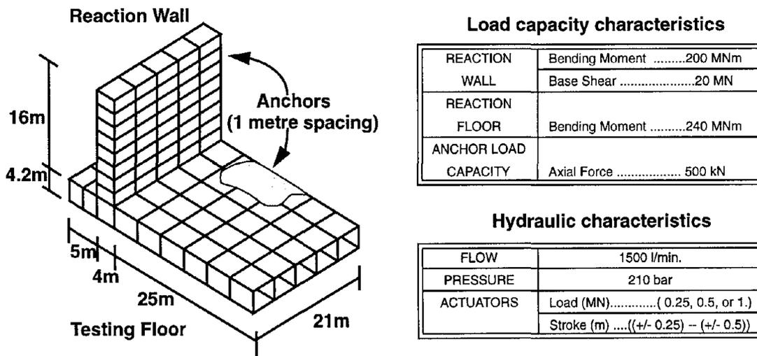
Figure 1- Characteristics of the ELSA-Reaction Wall Laboratory.
