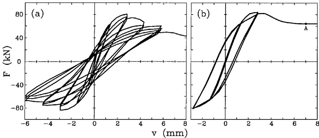
Figure 4. Lateral hysteretic response of a squat wall: (a) experimental, (b) continuum model.
