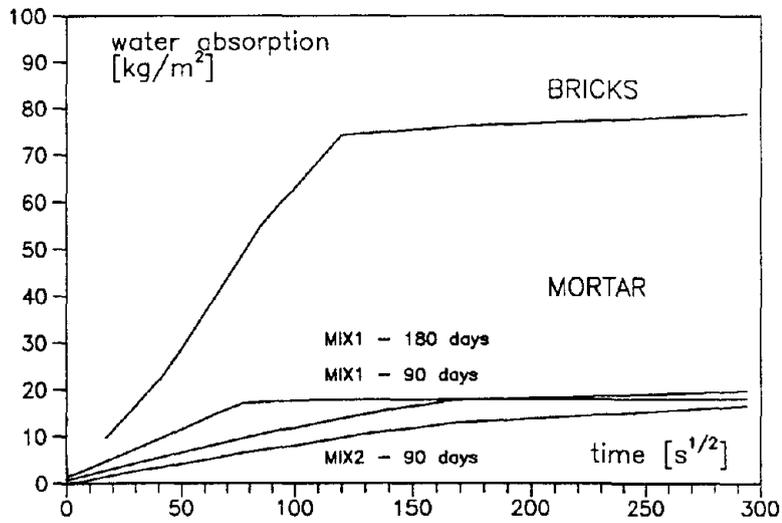
Fig. 6 - Capillary rise average plots for mortars and bricks
