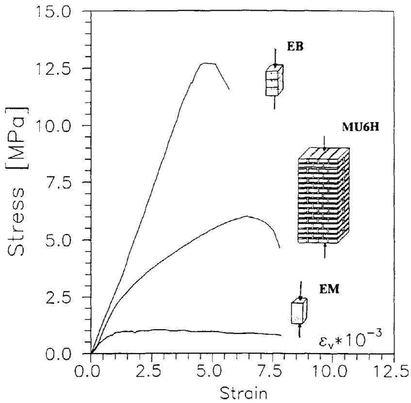
Fig. 22 - Stress-strain plots for mortar, brick and masonry prisms
