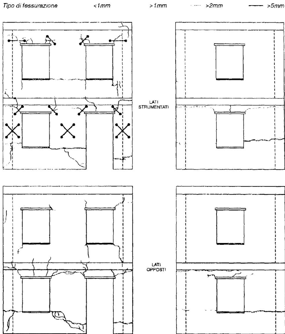
Fig. 5. Sketch of the experimentally observed damage for the test N. 5 (0 dB).
