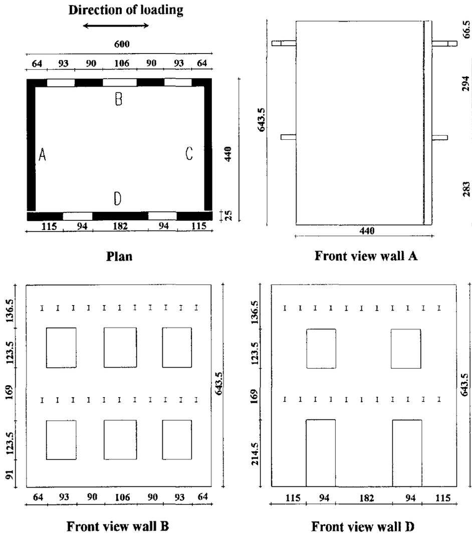
Fig.2. Plan, front, lateral views and dimensions of the prototype, dimensions in centimeters.
