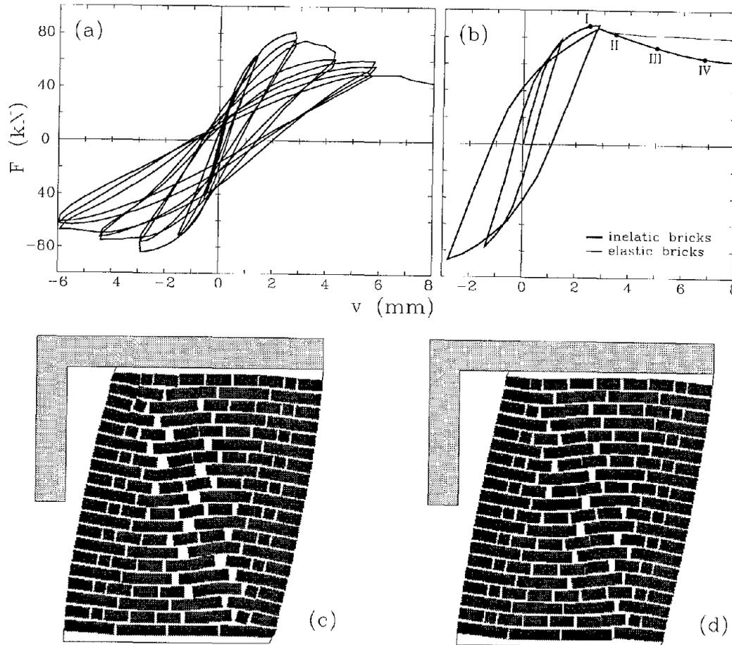
Figure 2. Rectangular masonry panel: (a) experimental response to horizontal actions [6]; (b) theoretical response by the composite model; (c) wall configuration ( $v=10$  mm); (d) wall configuration assuming elastic bricks ( $v=10$  mm).
