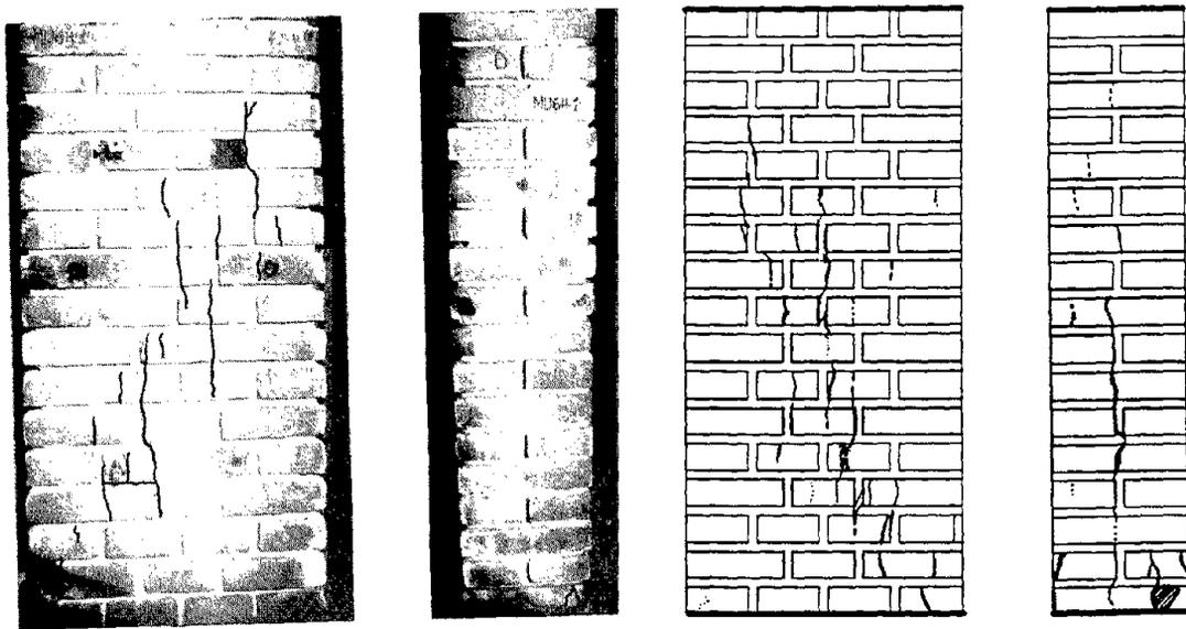
Fig. 20 - Design for displacement measurements on the prisms, and crack pattern
