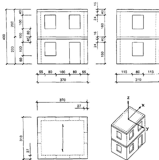
Fig. 1. Main geometrical features of the tested masonry building prototypes (lengths in cm).
