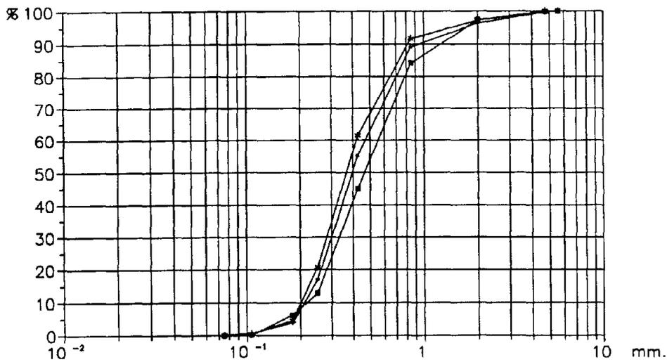
Fig. 4 - Grain size and distribution of the sand
