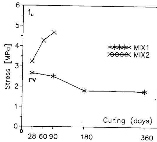
Fig. 9 - Strength versus curing time for mortars (MIX1, MIX2)
