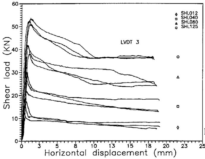
Fig. 18 - Shear load-displacement curve for the different values of horizontal load
