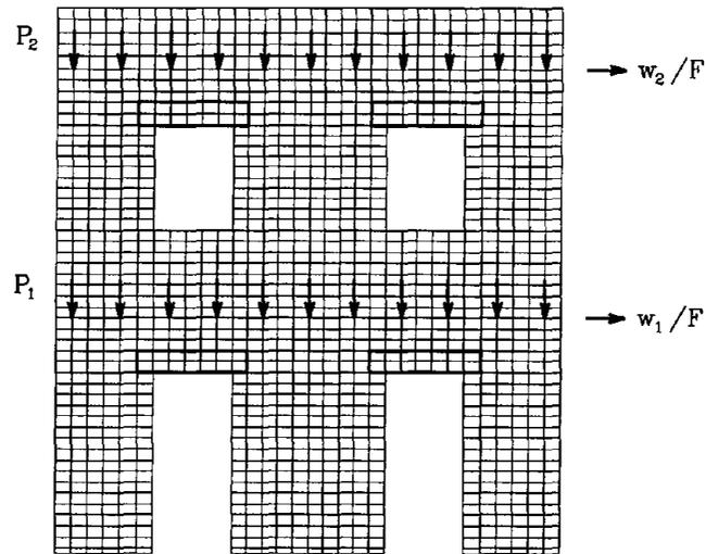
Figure 6: Finite element model of the large scale perforated wall [12].
