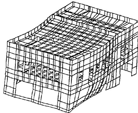
Fig. 2 Computed First-Mode Shape
