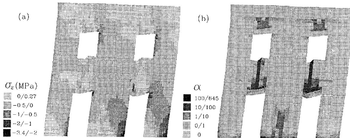
Figure 8. Large scale perforated wall: vertical stress (a) and mortar joint damage  $\alpha_m$  (b) distributions for 0.2 % drift.
