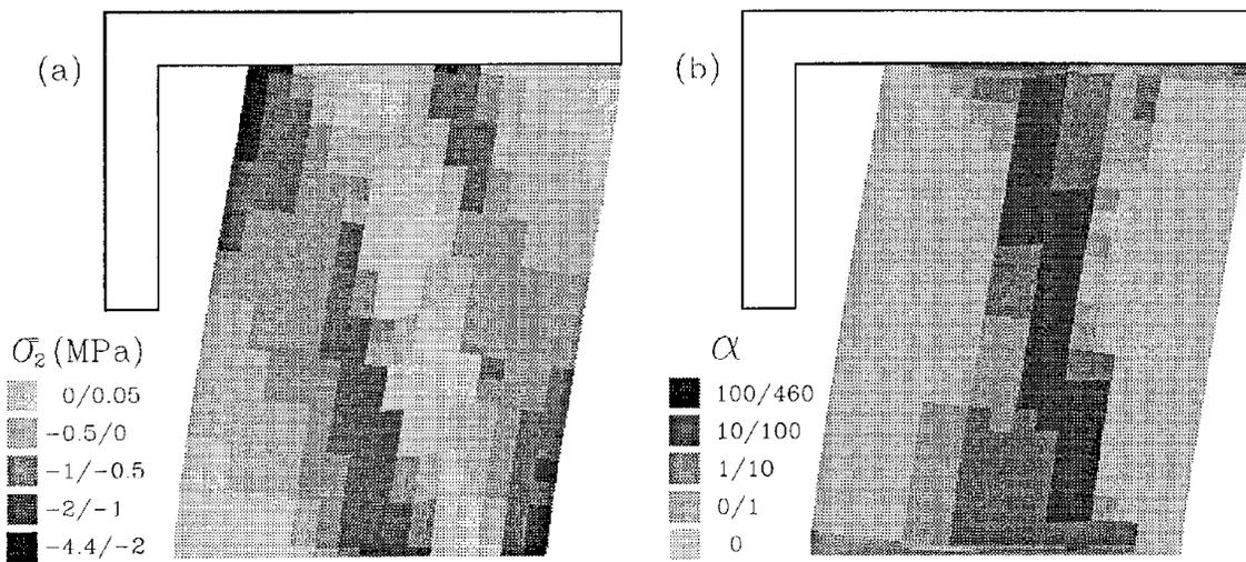
Figure 5. Rectangular wall: vertical stress (a) and joint damage  $\alpha_m$  (b) distributions at the state A.
