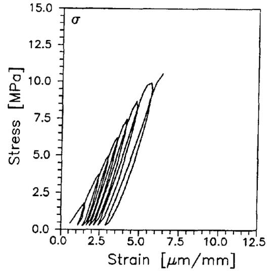
Fig. 16b - Stress-strain plot for EBB under cyclic vertical load
