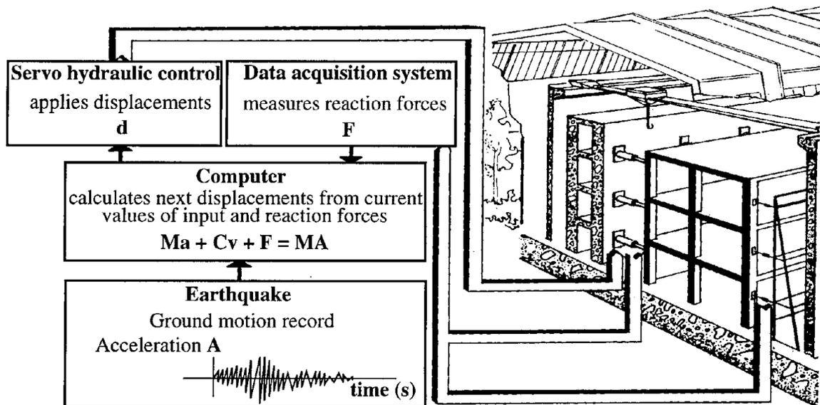
Figure 2- Pseudo-dynamic test (schematic)
