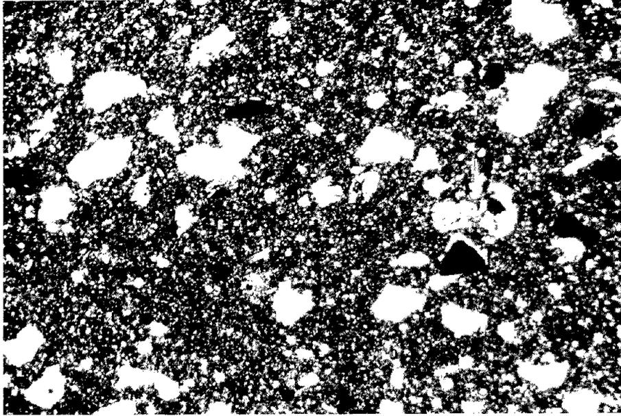
Fig. 5 - Thin section of the brick; the two distinct grain size of the quartz are clearly visible
