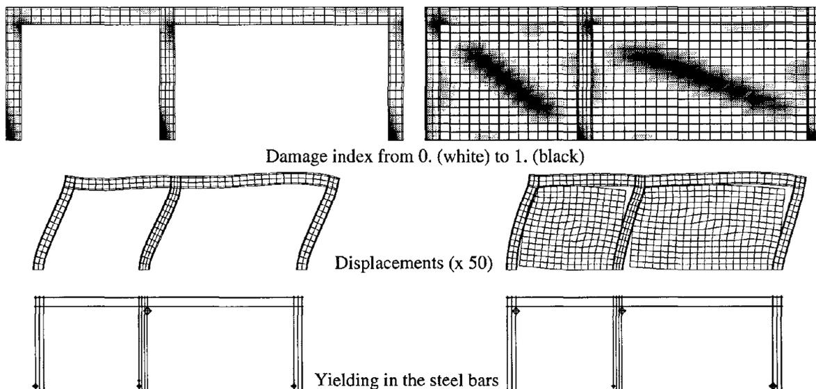
Figure 13- Results for the first storey with and without infill.
