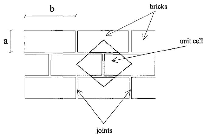
Figure 6 Unit cell of on line brickwork
