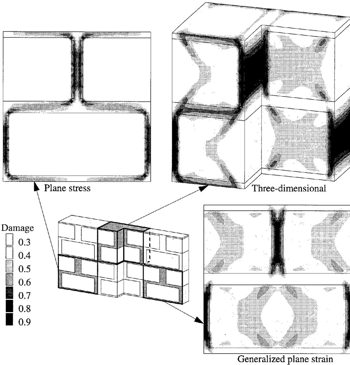
Figure 11- Damage at maximum compression stress.
