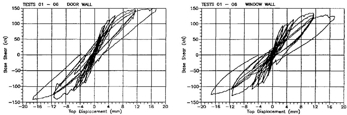
Fig. 10. Top displacement vs. base shear for walls D (door wall) and wall B (window wall).
