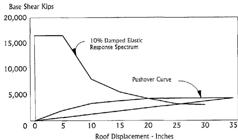
Fig. 11 Capacity Spectrum Plot for Example Structure
