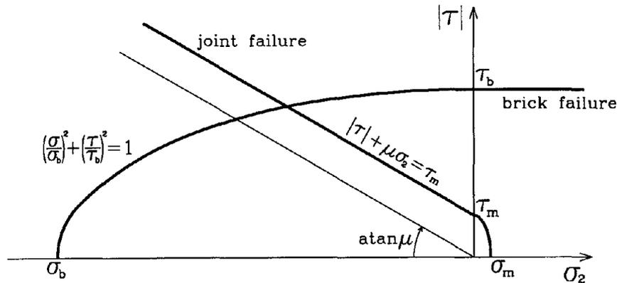
Figure 3. Joint and brick failure domains in the  $(\sigma_2, |\tau|)$  plane.
