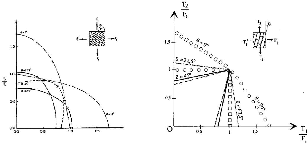
Figure 10 Comparison with the failure condition numerically obtained by Page (12) in the tension range
