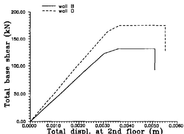
Figure 6. Example of calculated shear-displacement envelopes for walls B and D, assuming a 1/1 ratio for the seismic forces at 1st and 2nd storey.
