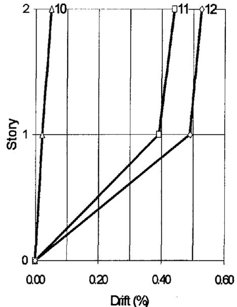
Fig. 8 Deflected Shapes for North Wall
