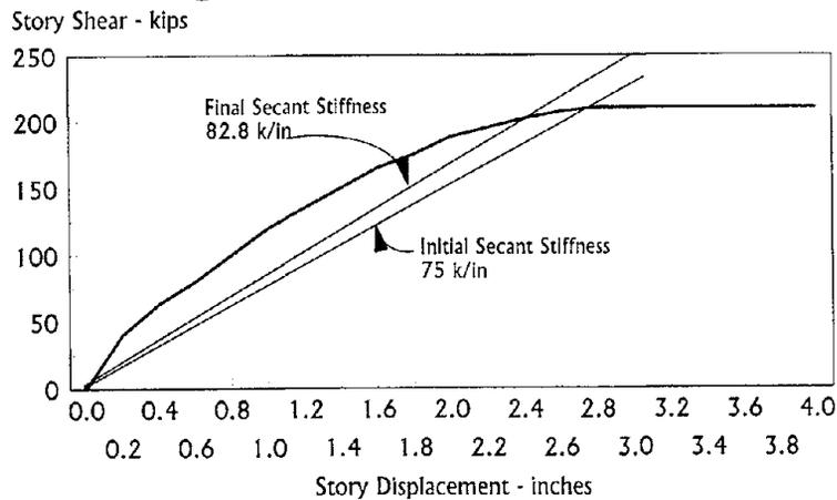
Fig. 10 Pushover Curve for Story, showing iterative deflection estimation approach
