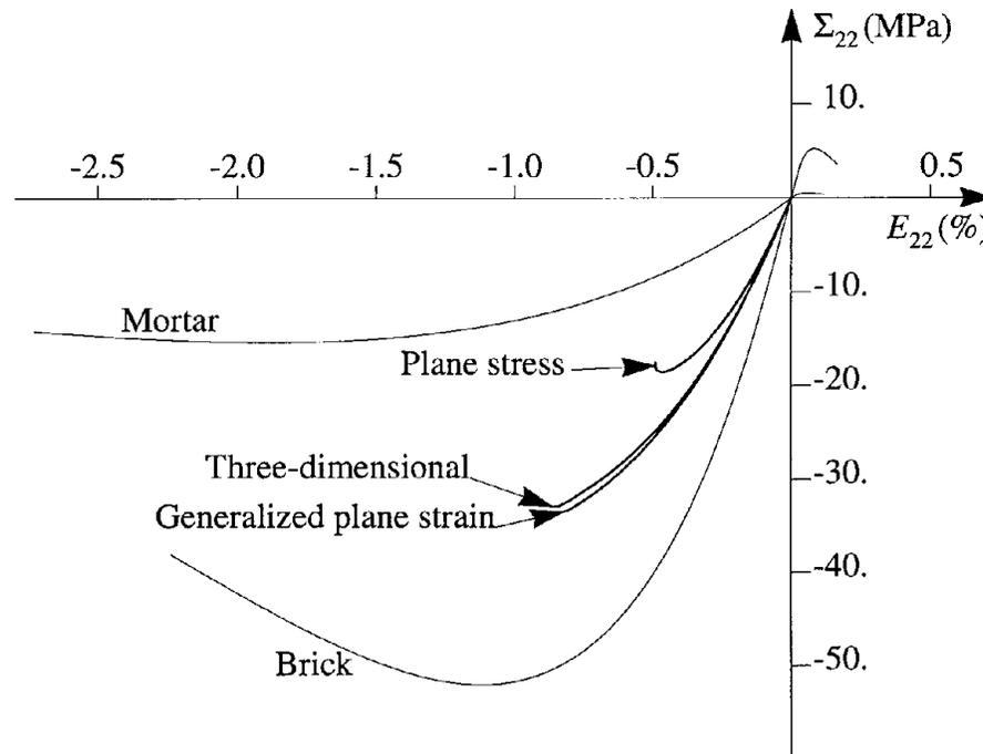
Figure 10- Uniaxial vertical compression curves.
