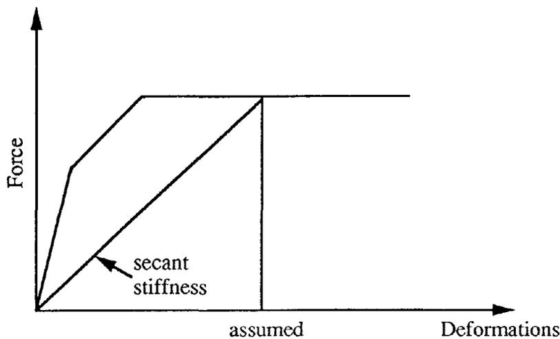
Fig. 2 Secant Member Stiffness for Iterative Approach
