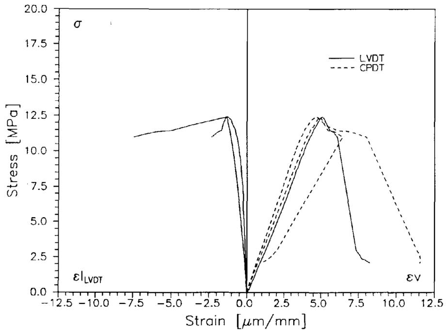
Fig. 15 - Stress-strain curves obtained from CPDT and LVDT measurements for EB
