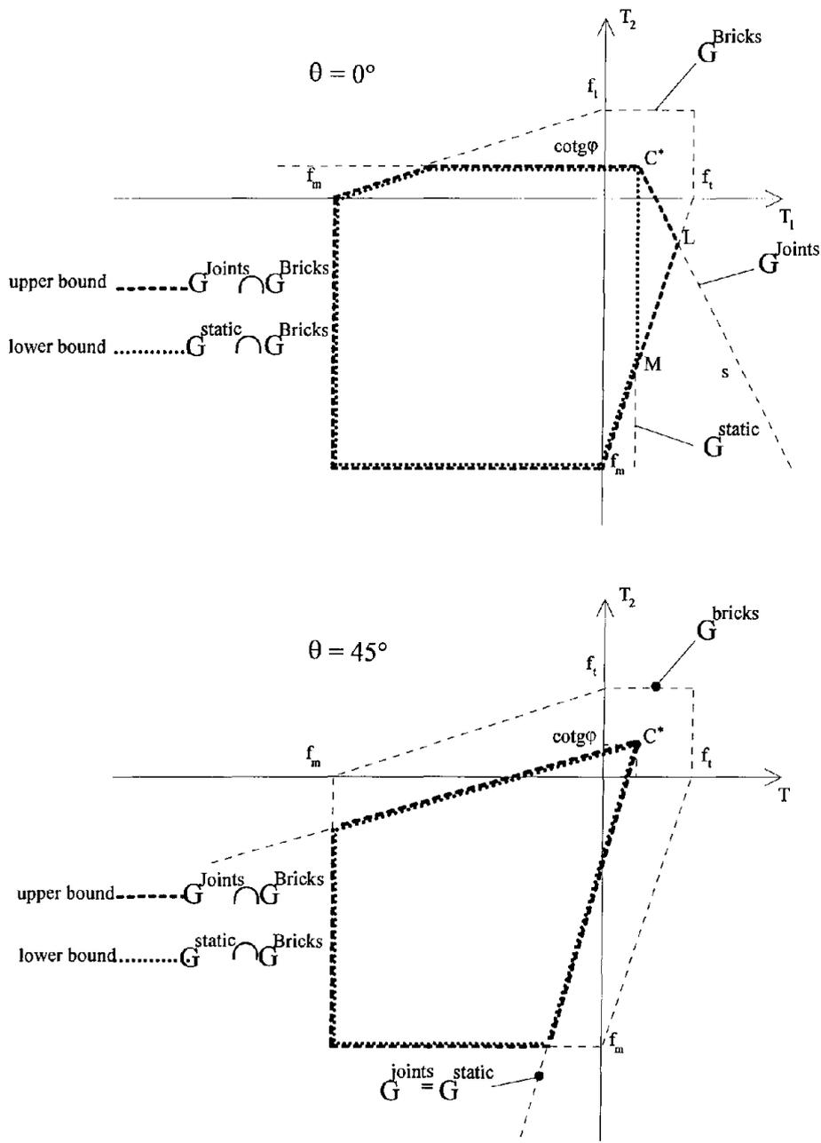
Figure 11 Macroscopic strength condition with respect to joint and brick failure
