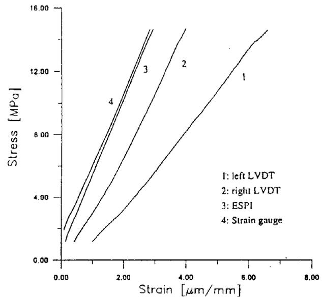
Fig. 13b - Stress-strain curves obtained with the strain gauges and by measuring the interferometric fringes
