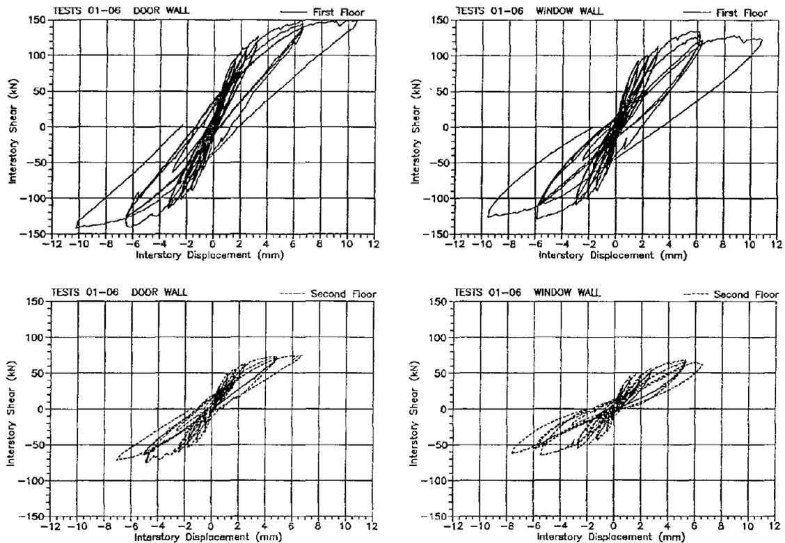
Fig. 9. Experimental interstorey shear vs. interstorey displacement curves
