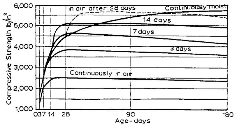
Fig. 10 - Influence of moist and air curing on concrete strength
