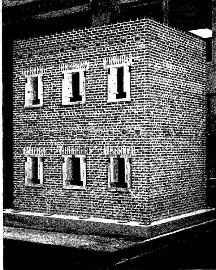
Fig. 3 Test Structure on Shaking Table
