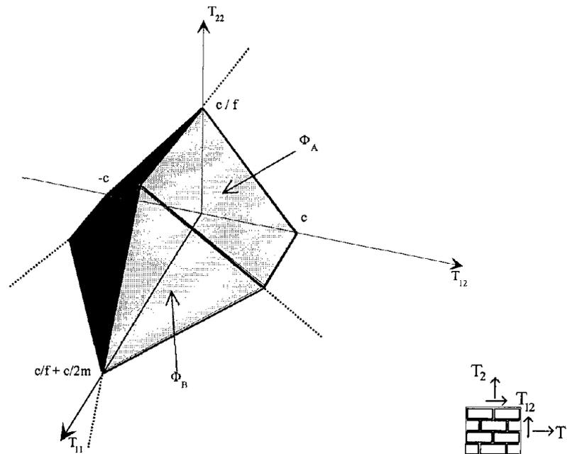
Figure 9 Macroscopic strength condition whit respect to joint failure in the stress space on the refernce of joint directions
