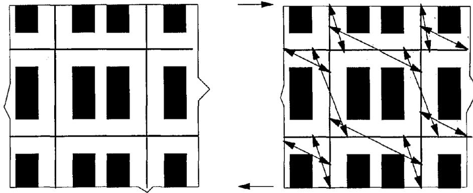
Fig. 8 Typical Compressive Fields in Laterally Loaded Penetrated Wall Panel
