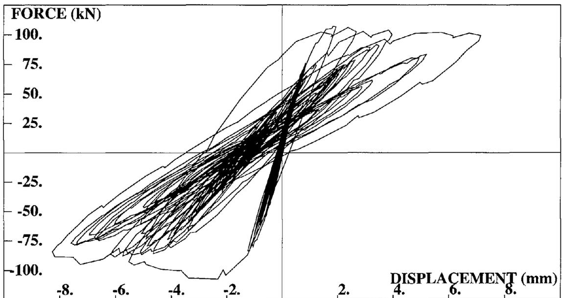
Figure 9- Horizontal force versus horizontal displacement at the top of the wall.
