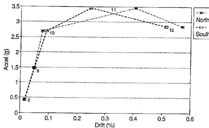
Fig. 6 Measured Top-Level Diaphragm Acceleration vs. Drift
