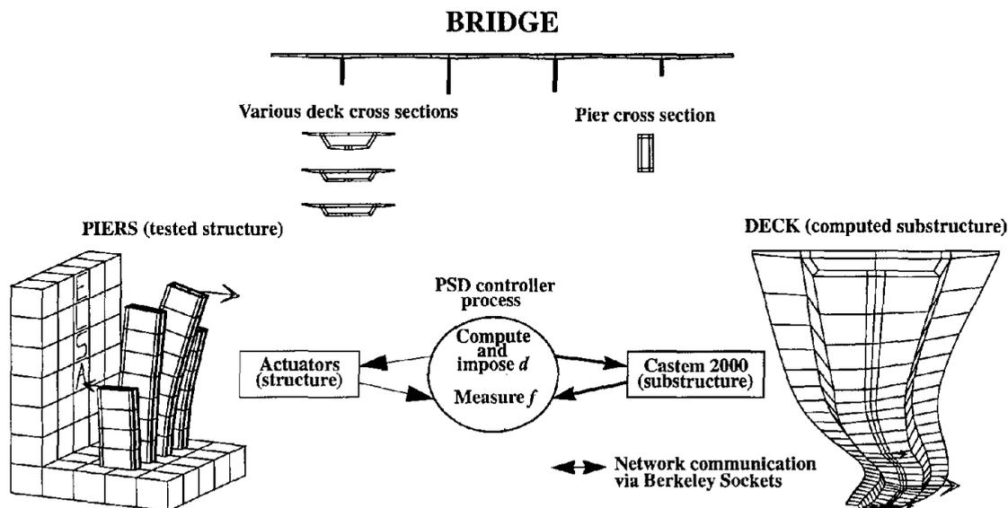
Figure 3- Pseudo-dynamic testing with substructuring: a four piers bridge case.
