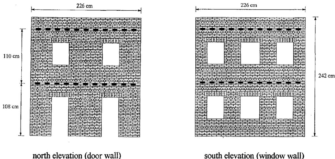
Fig. 4 Dimensions of Shaking Table Structure
