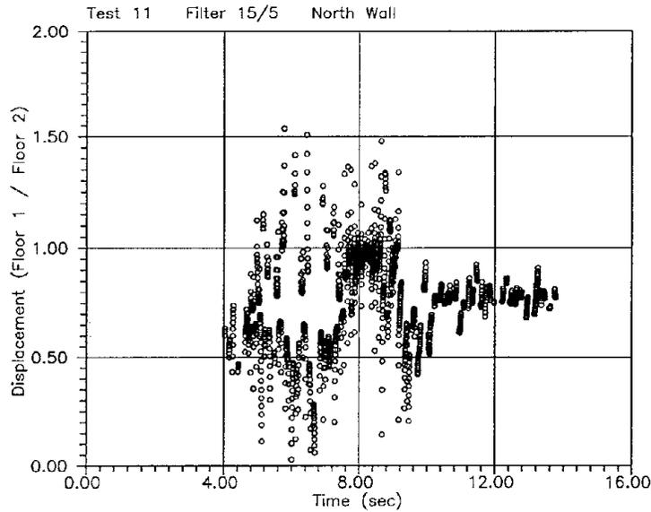
Fig. 9 Ratio of First to Second Level Deflection vs. Time - Run 11
