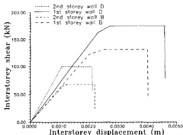
Figure 5. Calculated interstorey shear-drift envelopes for walls B (window wall) and D (door wall).
