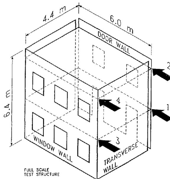
Fig. 3. The seismic forces in the full scale static test are simulated with four concentrated forces.
