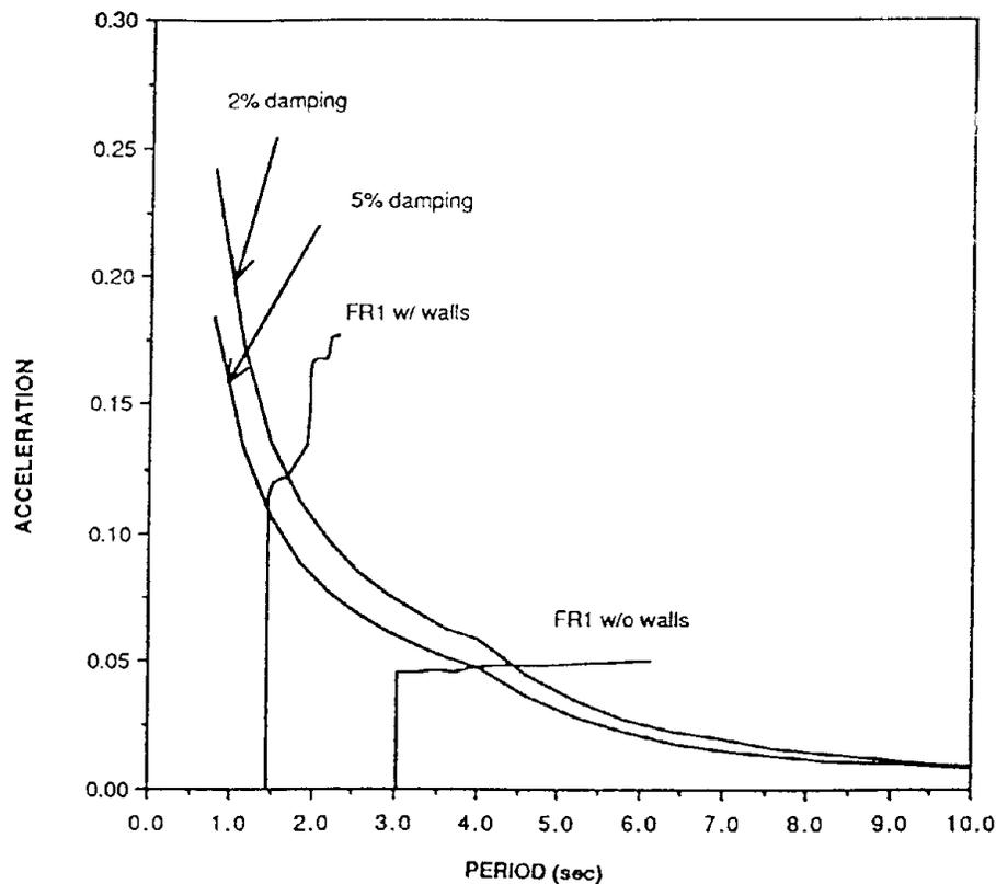
Fig. 3 The Capacity Spectrum Method for a Ten-story Infilled Steel Frame
