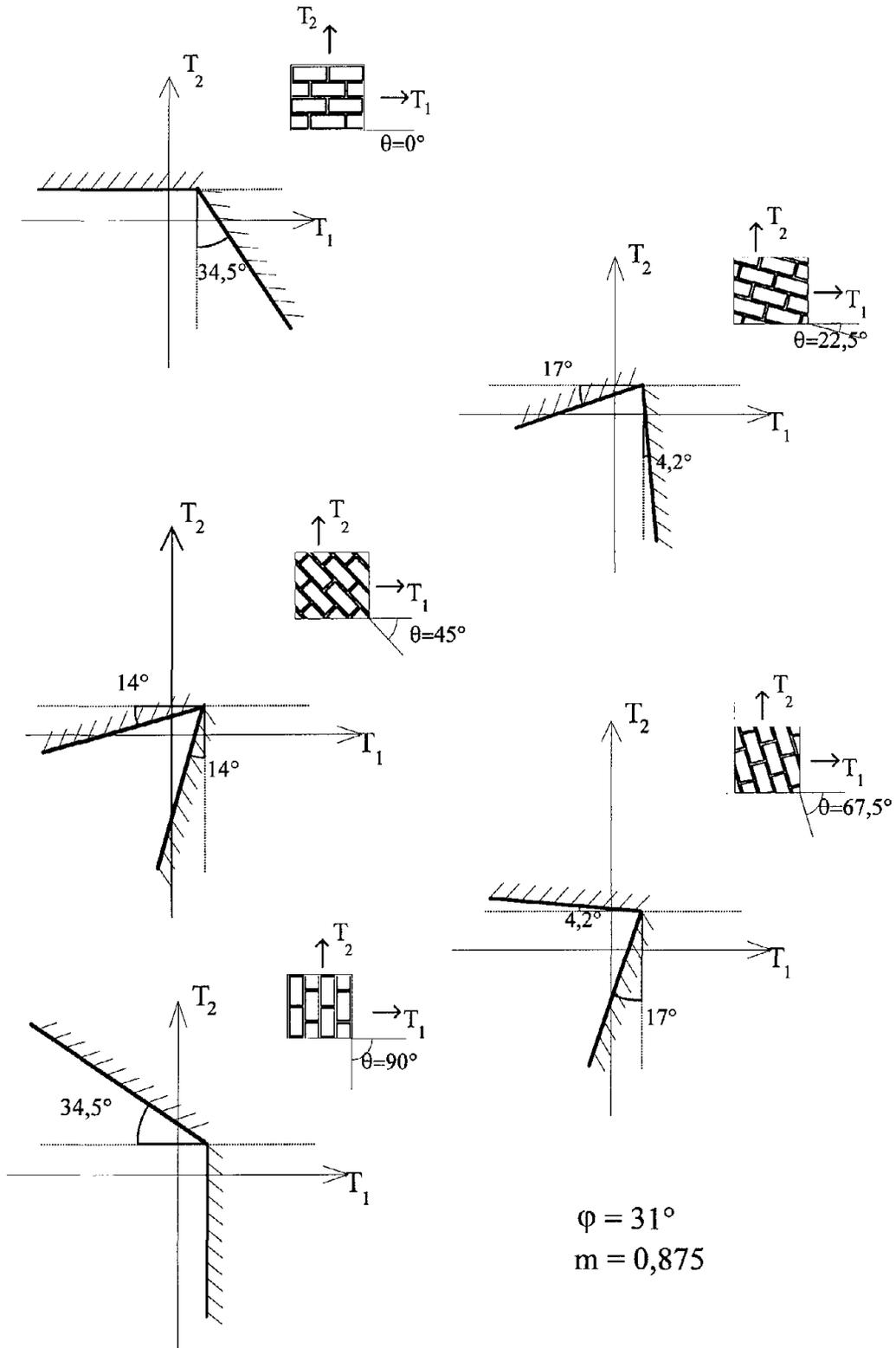
Figure 8 Macroscopic strength condition with respect to joints failure in the plane of principal stress
