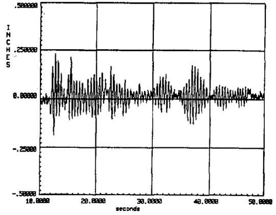
Figure (a) Experimental Results for OPW Walls-Test Phase 1
