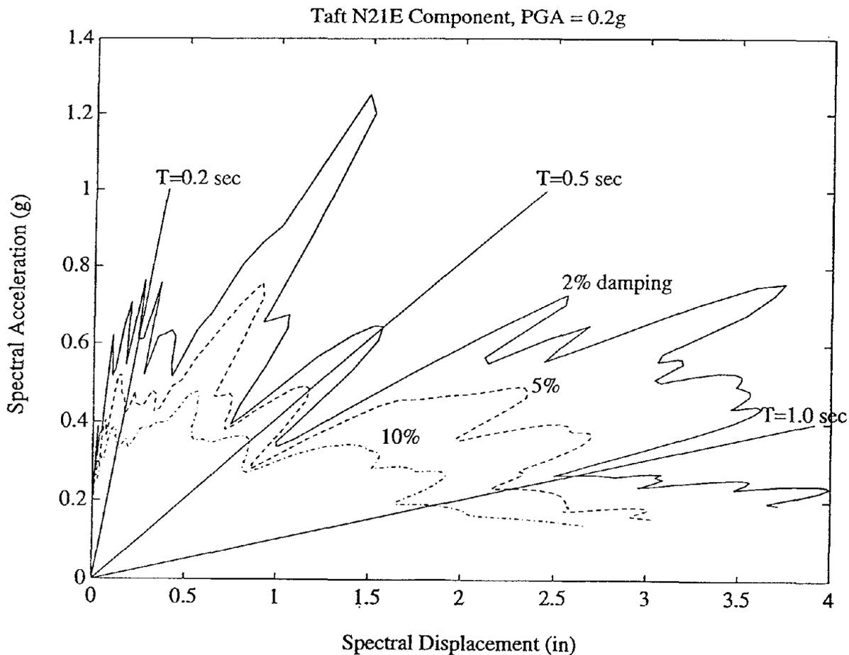
Fig. 4 Response Spectrum Curve Plotted in a New Way
