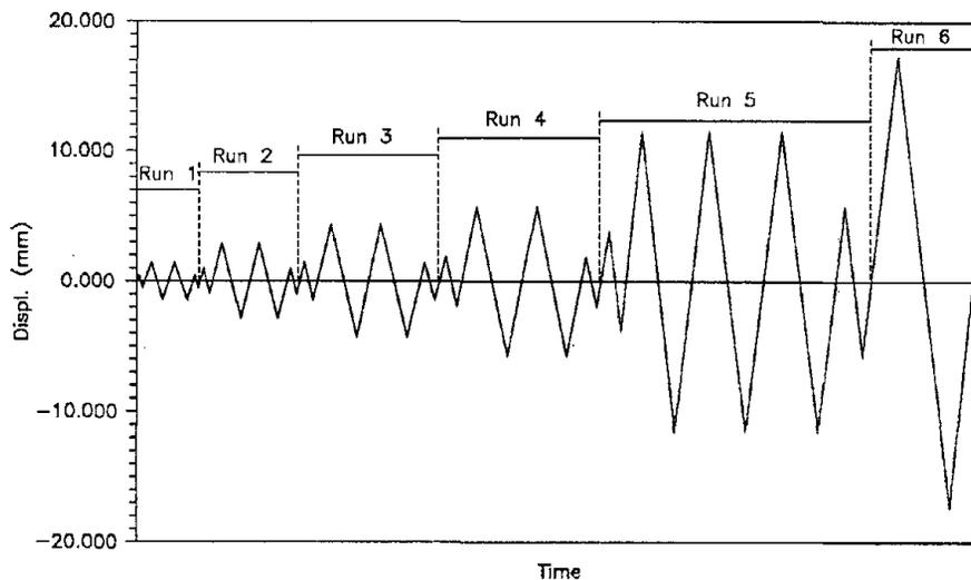
Fig. 8. Displacement history applied at the top floor in the runs already completed.
