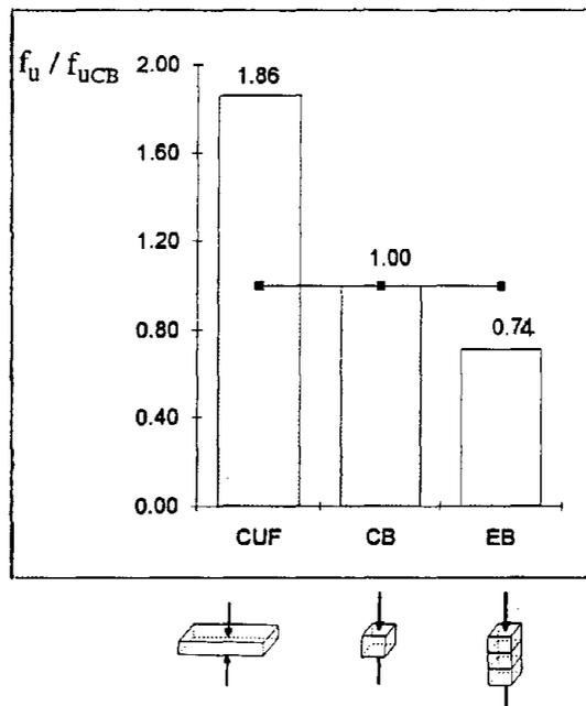
Fig. 23 - Brick specimens: strength ratio cube/whole units, cubes/prisms
