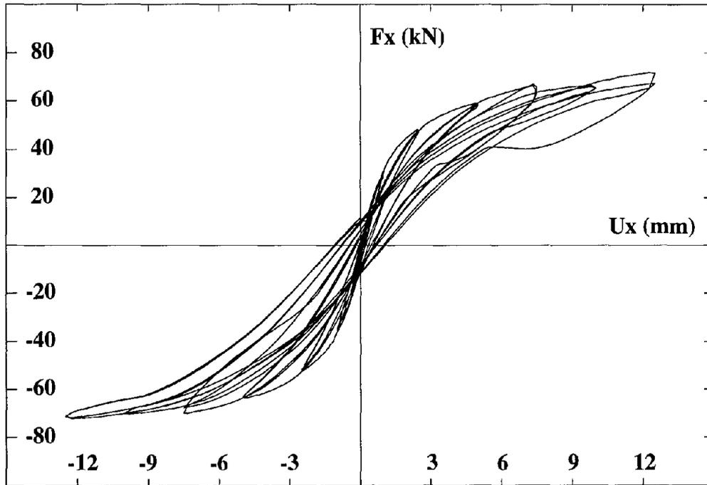
Figure 6- Horizontal force  $F_x$  versus lateral displacement  $U_x$  for the high wall.
