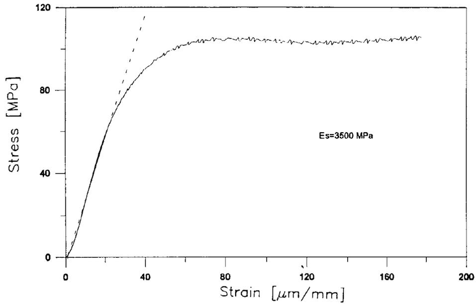
Fig. 12 - Stress-strain plot of the glue used to attach strain gauges
