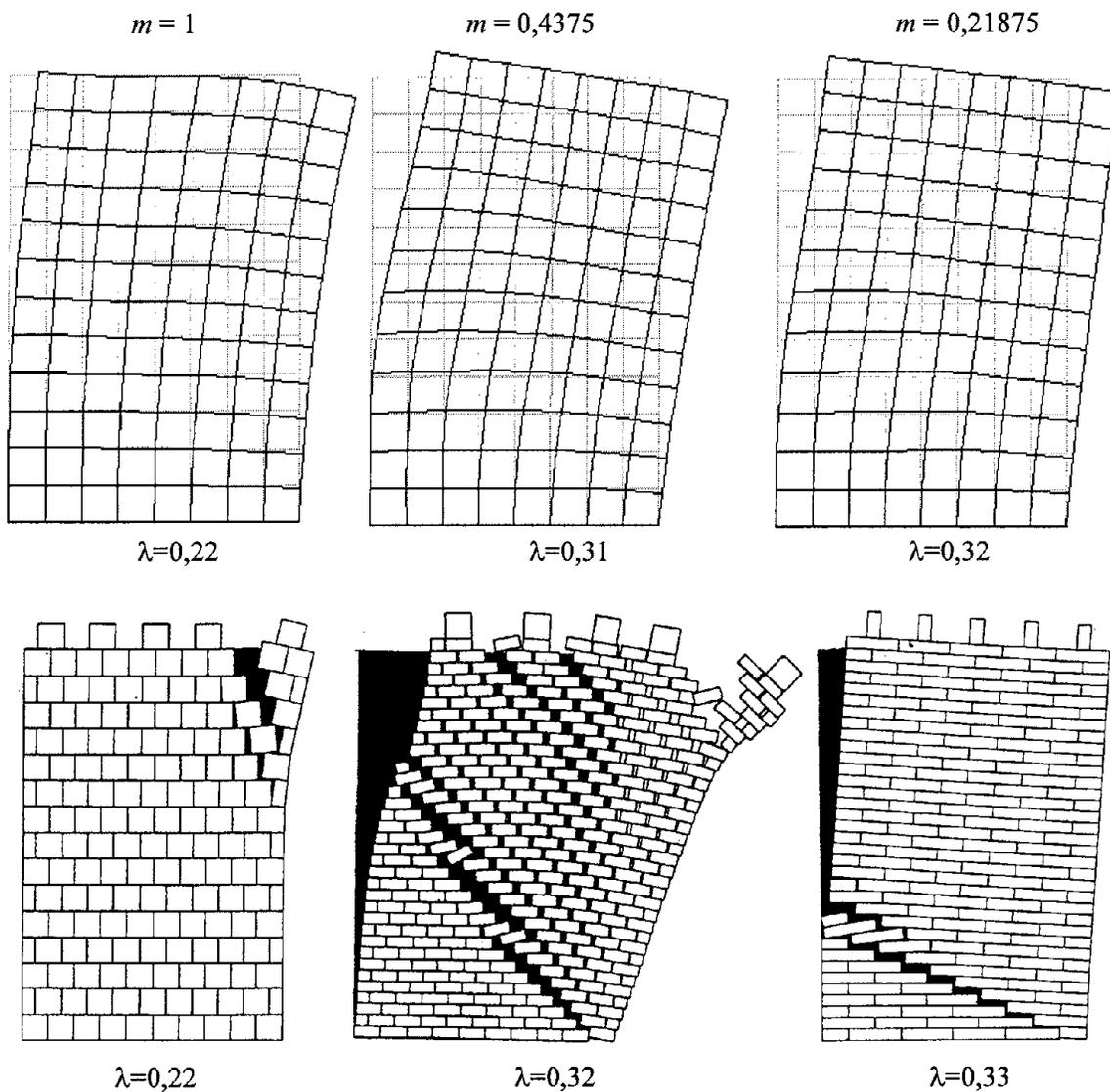
Figure 12 Comparison between homogenized and discrete structure limit behaviour
