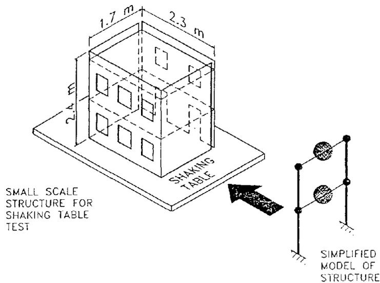
Fig. 7. Idealization of the response of the shake table model tested in Urbana.
