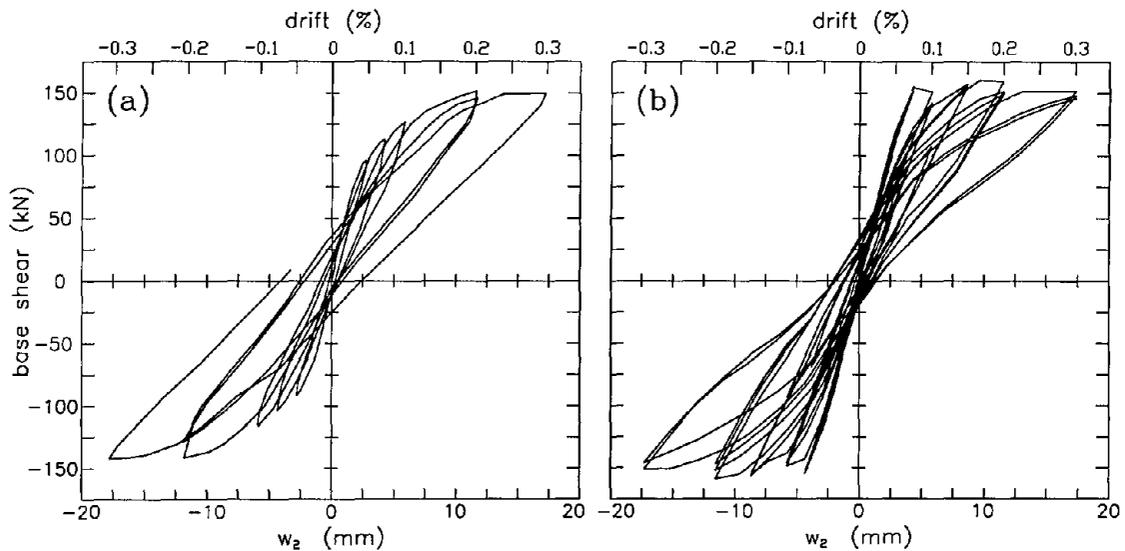
Figure 7. Experimental (a) and theoretical (b) lateral hysteretic response of the large scale perforated wall [12].
