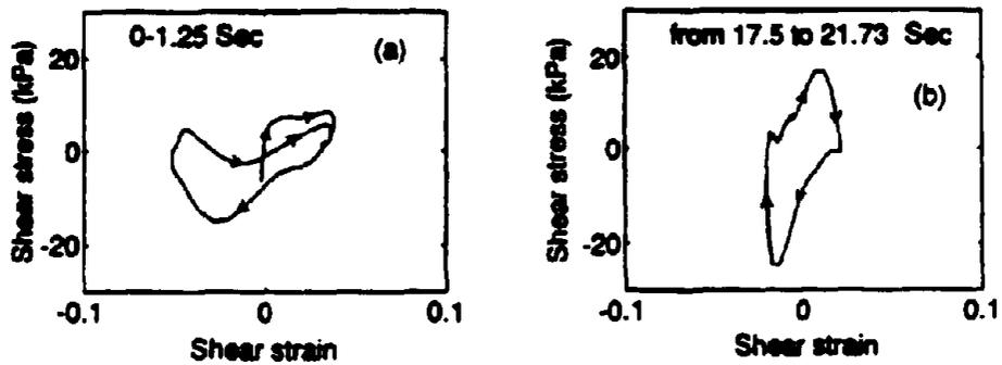
Fig. 3 Sample calculated stress-strain response.
