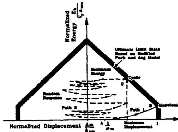
Figure 2: Non-Linear Response in Normalized Energy-Normalized Displacement Space
