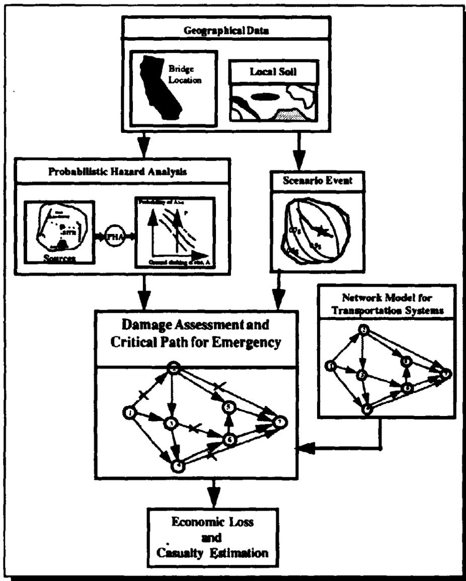
Figure 1. Methodology for Seismic Consequence Analysis of Transportation System
