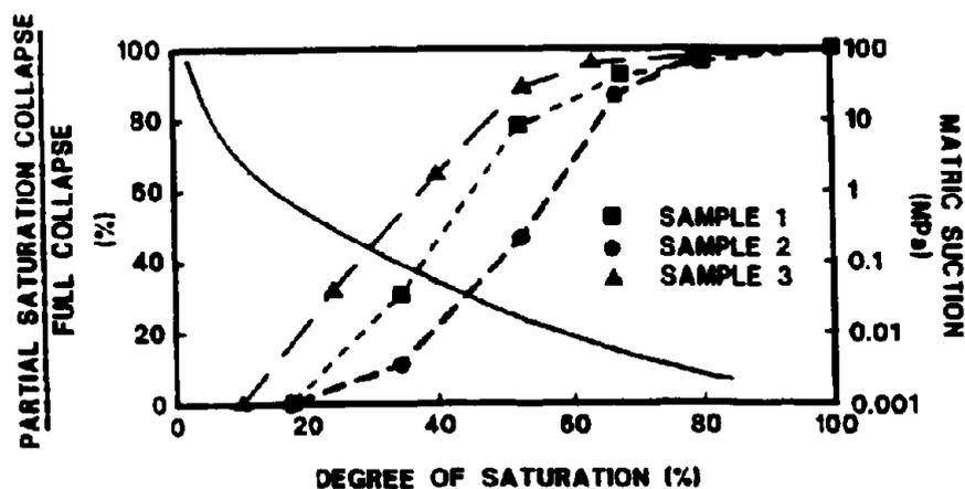
Figure 1. Partial Collapse Due to Partial Wetting for Three Collapsible Silts
