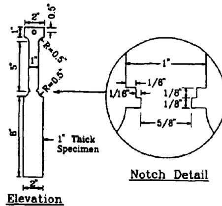
Figure 3: Specimen Dimensions and Test Setup
