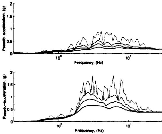
Fig. 3 Response Spectra Below Isolators
