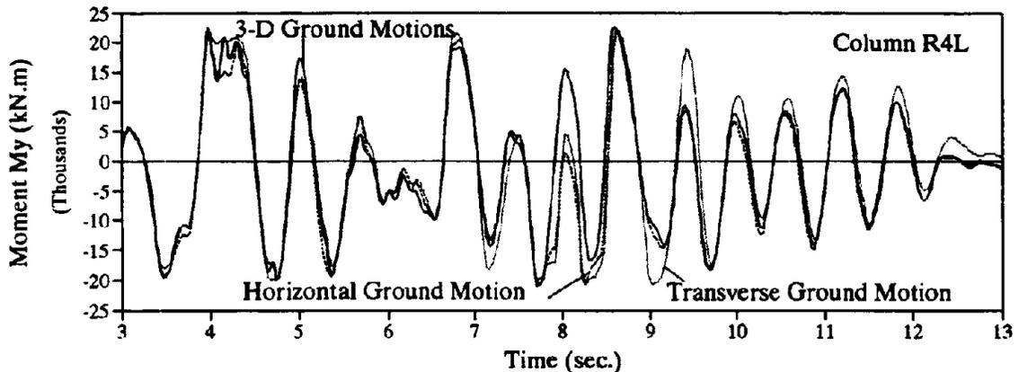
Fig. 4 Moment  $M_y$  Due to 1-D, 2-D, and 3-D Ground Motions
