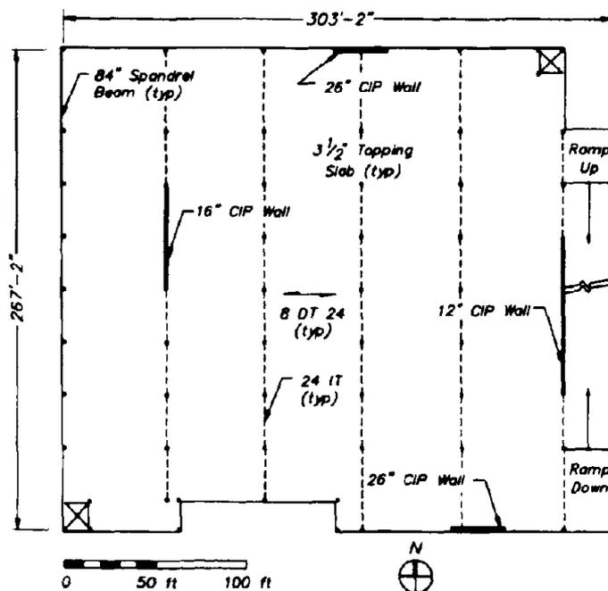
Fig. 2 Second-Floor Plan of Parking Garage B
