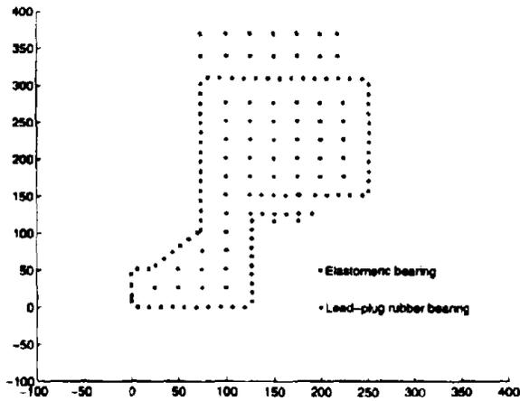
Fig. 1 Layout of Isolators for USC Building
