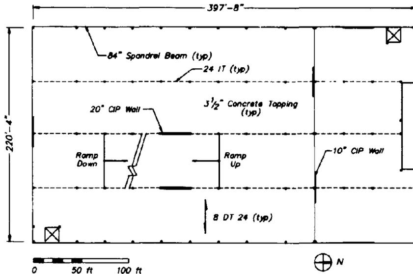
Fig. 1 Second-Floor Plan of Parking Garage A
