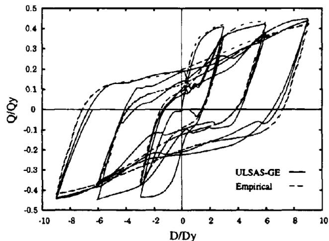
Fig. 4 Comparison between Analytical and Predicted Hysteresis of a Panel
