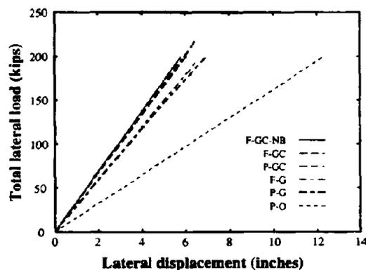
**Fig. 2 Behavior of Frame-Wall & Frame Systems with Different Connection Arrangements**
