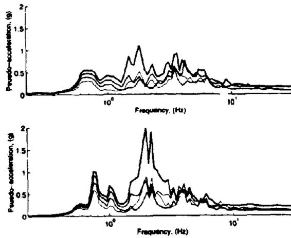
Fig. 4 Response Spectra in Superstructure, Damp=0.01
