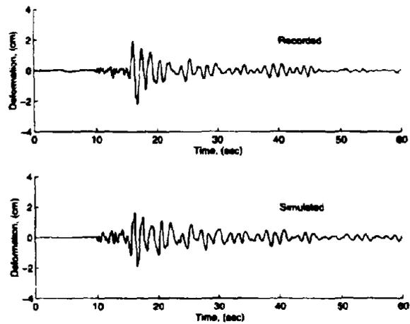
Fig. 6 Comparison of Recorded and Simulated Isolator Deformations, NS Direction
