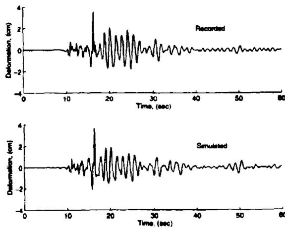
Fig. 5 Comparison of Recorded and Simulated Isolator Deformations, EW Direction
