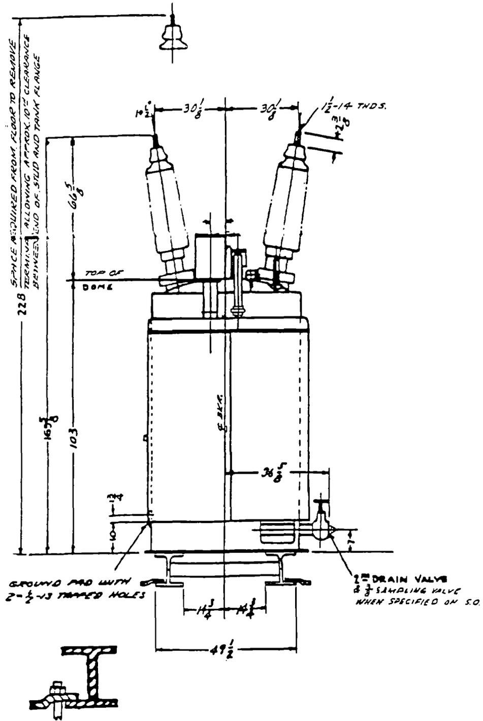
FIGURE 11-6 Elevation of GM-5 Type 115 kV OCB
