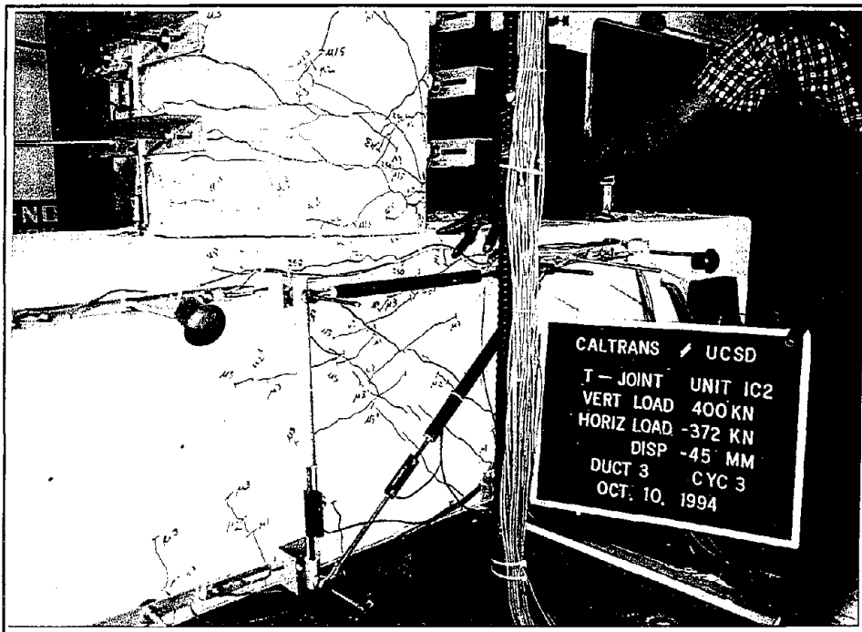
Figure 5.7 Condition of test unit IC2 at the end of testing at \mu_{\Delta} = 3 .
