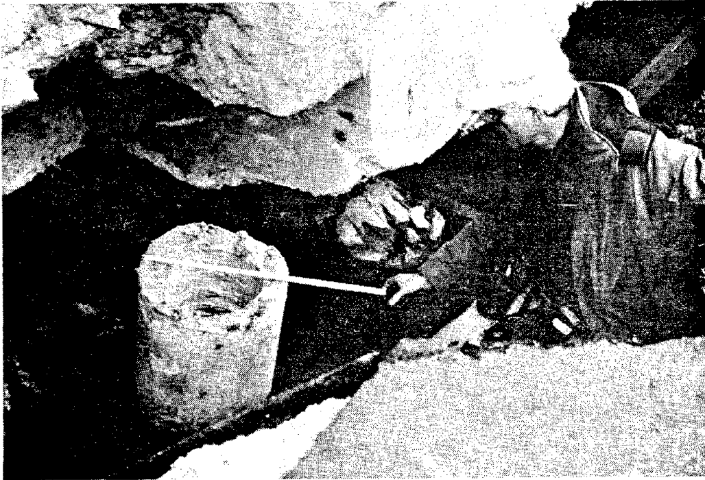
Fig. 4.6 Sheared and translated hollow tube pile.
