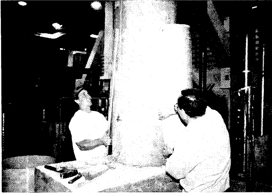
Figure 16 SnapTite System Being Prepared For Testing
