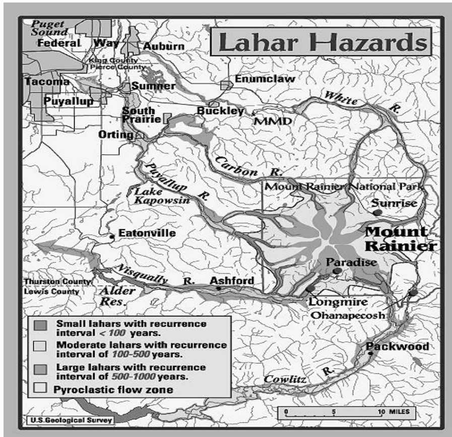
Hazard zones from lahars, lava flows, and pyroclastic flows from Mount Rainier (USGS Open-File Report 98-428 by Hoblitt and others, 1998)
