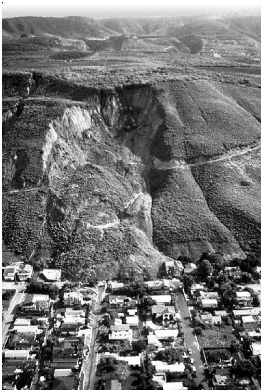
Massive Landslide at La Conchita, California - a small seaside community along Highway 101 north of Santa Barbara. This landslide and debris flow occurred in the spring of 1995. Many people were evacuated because of the slide, and the houses nearest the slide were completely destroyed. Fortunately, no one was killed or injured. (Photograph by R.L. Schuster, USGS)
