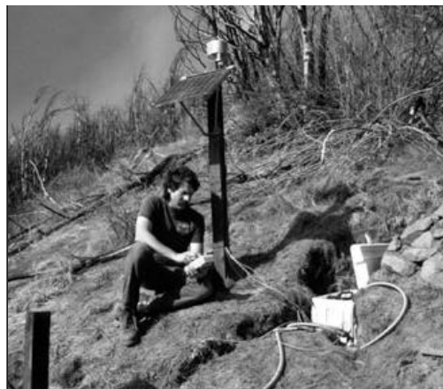
Testing a solar-powered radio telemetry system for remote transmission of real-time landslide data. (Photo by Mark Reid, USGS)
