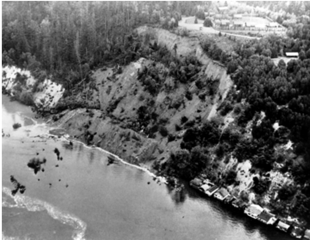
Figure 203. Tacoma, Wash., landslide, April 16, 1949 (pl. 5, loc. 81). This landslide was probably initiated by the 1949 earthquake that occurred 3 days previously. The large mass narrowly missed homes to the south on Salmon Beach as it plunged into the waters of the Tacoma Narrows. The resulting 2.5 m tidal wave damaged small boats and nearby dock facilities. Photograph used by permission of the Associated Press.
