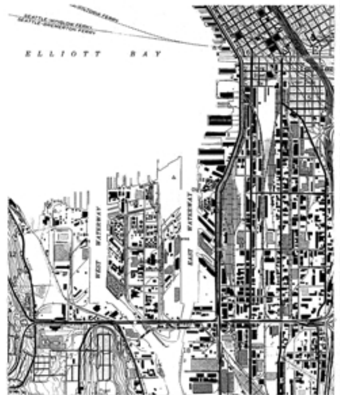
Figure 192. Maps showing the sequence of development of the former tidal flats area at the mouth of the Duwamish River, Seattle, between the years 1893 and 1973. Since 1893, the tidal flats have been extensively covered by artificial fill to allow waterfront development. The area was the site of many earthquake-induced ground failures and considerable property damage in both 1949 and 1965. From U.S. Geological Survey (1894, 1909, and 1949 (photorevised 1968, 1973)).
