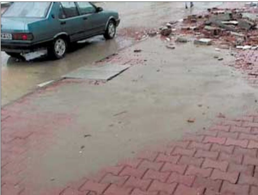
Figure 36. Sand boil on sidewalk in Adapazari. Sand ejected from underground when sandy soils beneath the ground-water table liquefied during the earthquake. Photograph by Mehmet Çelebi.
