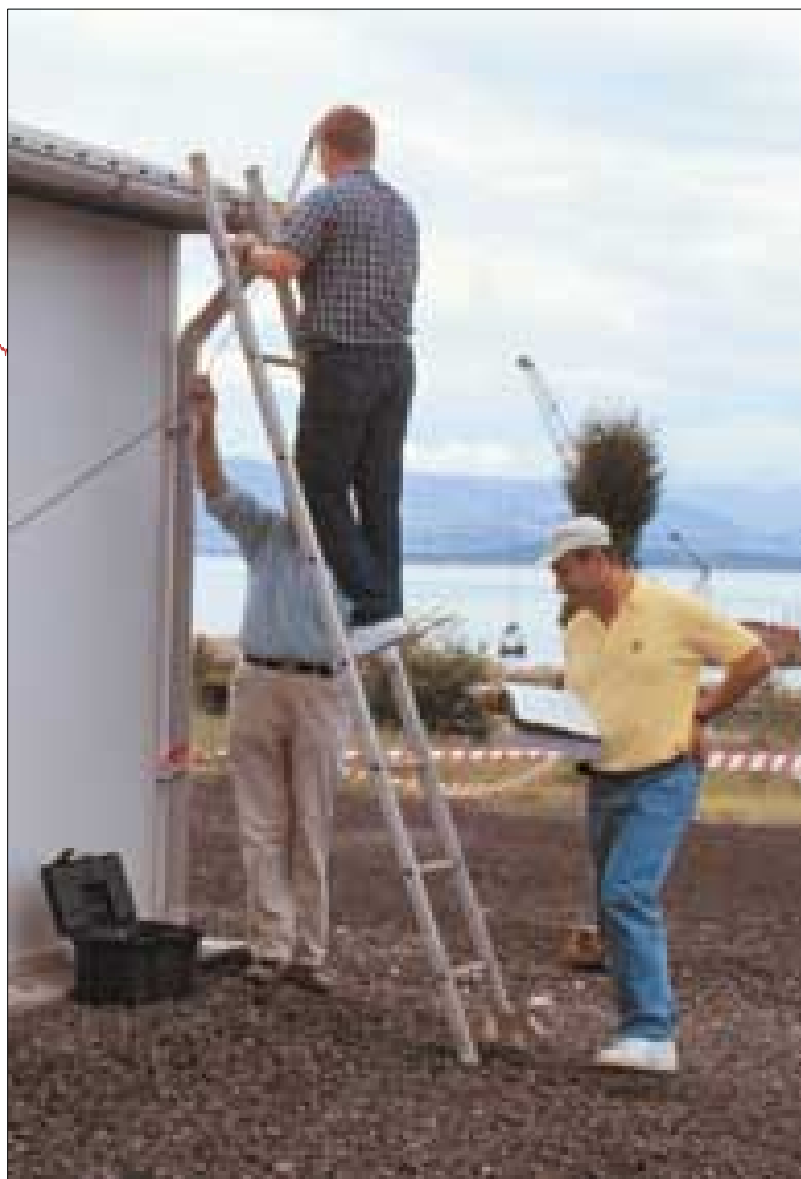
Figure 29. USGS scientists deploy an antenna for a portable seismic recording system at Dilovasi. Antenna receives time signals from a satellite and allows the timing on the portable seismographs to be synchronized with each other. Photograph by Thomas L. Holzer.
