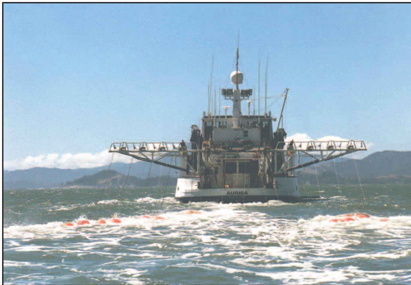
Figure 7.—Motor vessel Auriga , with 12-airgun source array, working in San Pablo Bay (see figs. 1, 5) during BASIX-3.
