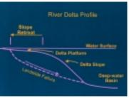
4. Overloading: Addition of material at the top of the delta slope (e.g. artificial fill) increases downslope weight of soil mass.
