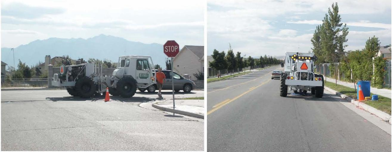
**Figure 3.** Photos of minivib during acquisition along 3200 W. in South Jordan, Utah. Left: view east toward Wasatch Range; right: view south showing seismic cabling along curb and minivib base plate in contact with asphalt. Similar source vehicle was used during S-wave minivib acquisition in Salt Lake and Utah Valleys during field investigations described in this report.
