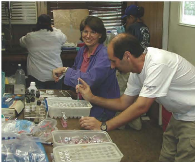
USGS scientist inoculating microbial growth media to determine the number and type of microorganisms carrying out biodegradation in a contaminated aquifer.
