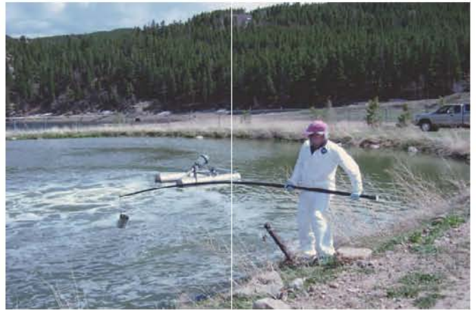
USGS scientist using a long sampling device to collect a sample of liquid from a municipal wastewater holding pond in Colorado as part of the Source Characterization Study for Emerging Contaminants Project. The sample was analyzed for pharmaceuticals and other wastewater compounds.
