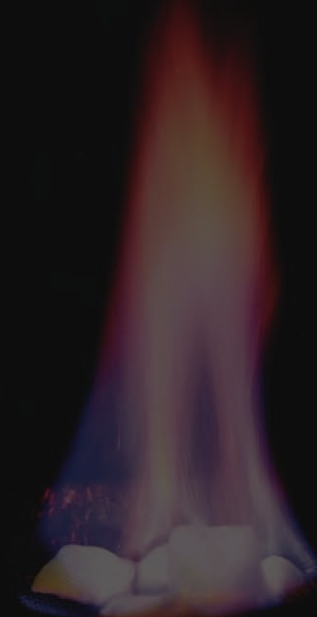
Fire in the ice: Although gas hydrates look like ice, they burn if the methane is ignited. Photograph by John Pinkston, U.S. Geological Survey.
