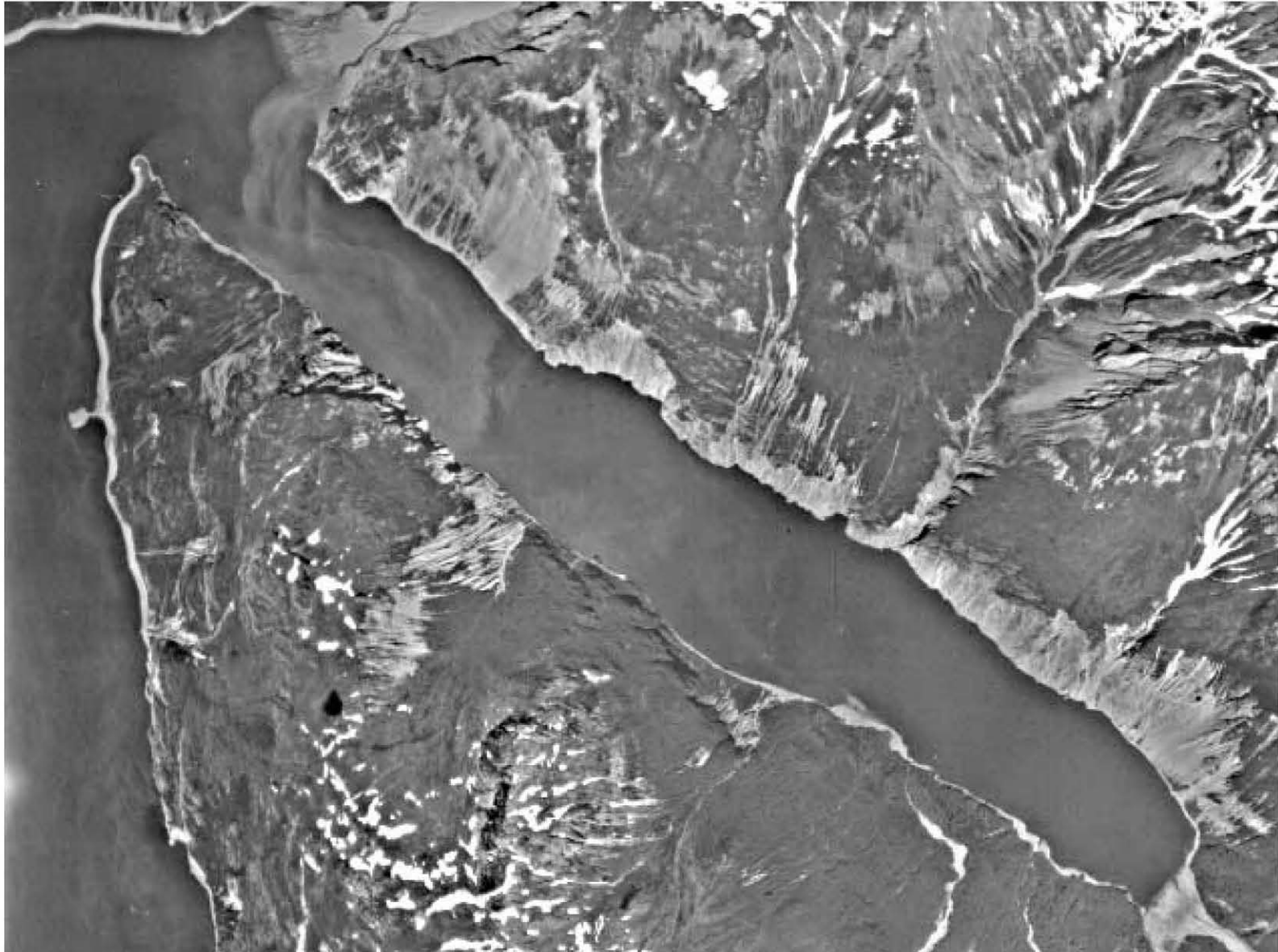
Figure 8. -- Portion of aerial photograph showing Tidal Inlet and eastern side of west arm Glacier Bay taken July 6, 1948. Note talus (bright light color) below recent landslide mass above northern shore (upper left corner) extending from landslide toe to shore of Tidal Inlet below central portion of landslide. Photograph taken by US Navy at 1:40,000-scale.
