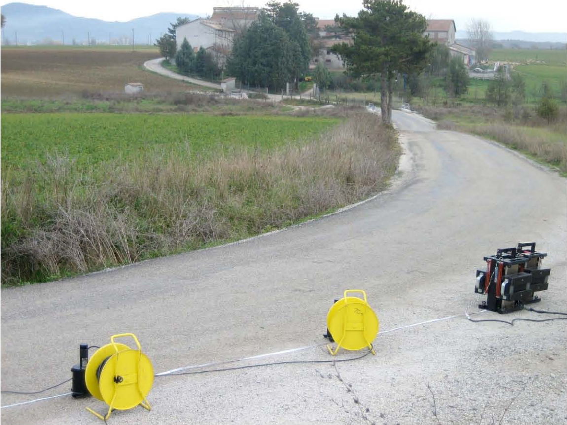
Figure 2. Configuration of the USGS surface wave testing system at site 262GBP Gubbio Soil Site Piana (43.314°N,12.59°E) composed of 1-Hz vertical motion sensors and two-100 kg electro-mechanical harmonic wave shakers. The shaker apparatus are arrayed in a parallel circuit and synchronized in phase for controlled swept-sine analysis.
