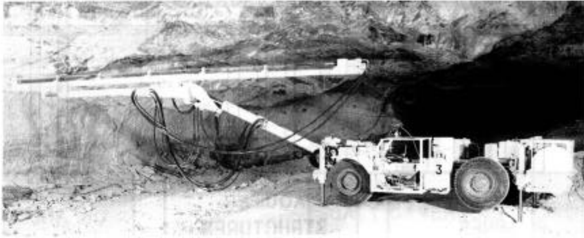
Fig 14. Photograph of a drilling “jumbo,” an example of the type of specialized equipment necessary to construct large caverns in hard rock.
