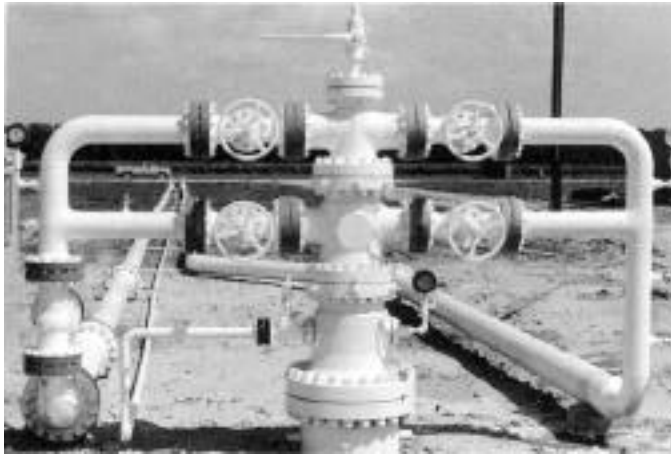
Fig 4. Photograph of a wellhead “Christmas tree” above a solution mined storage cavern, at natural gas storage well No. 2, Boling, Texas. At an operating storage cavern like Boling (which has two caverns, each 2.5 Mbbbl), this may be the only visible evidence for the mining operation.
