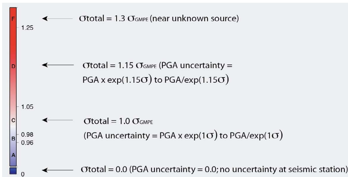
Figure 5. ShakeMap uncertainty scale bar. The decimal values at the right of the scale bar are the multiplicative factor to scale the uncertainty from the ground-motion prediction equation used. Zero uncertainty (blue) occurs at seismic stations; high uncertainty (red) occurs close to a unconstrained finite-fault source region. Letter “grades” are provided for the average uncertainty on a given ShakeMap, on land and within the zone of intensity VI or greater. See text for further details.
