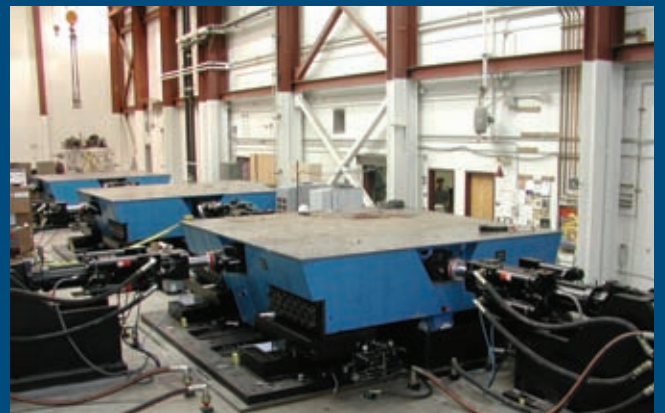
The James E. Rogers and Louis Weiner, Jr. Bridge Structures Laboratory at the University of Nevada, Reno features three identical shake tables.
